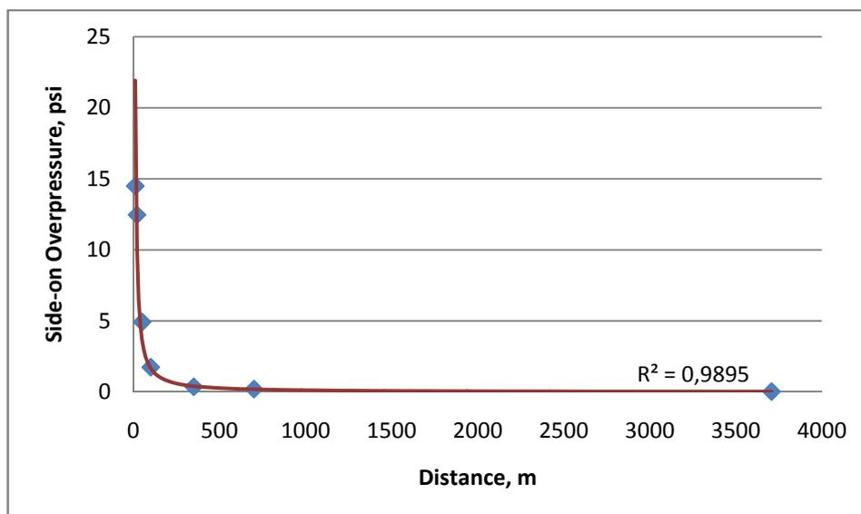
Figure 7.15: Side-on Overpressure vs. Distance
