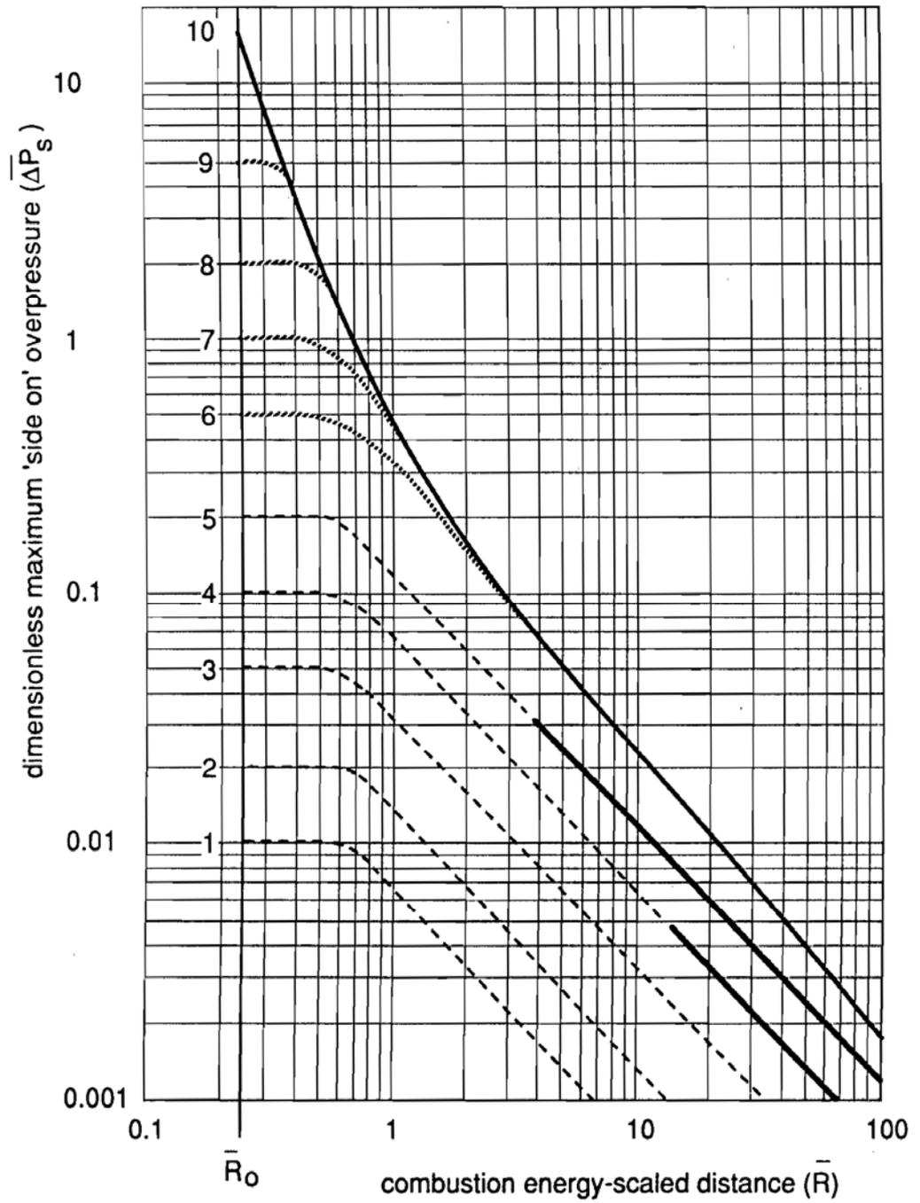
Figure F.1: Sachs scaled side-on peak overpressure of blast from a hemispherical fuel-air charge [65]
