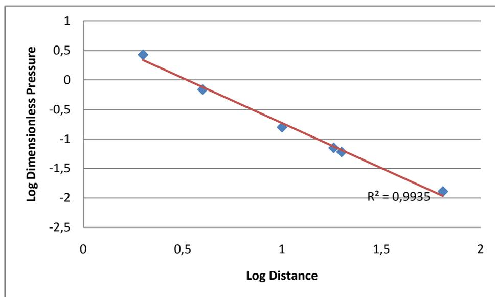
Figure 7.5: Side-on overpressure vs. distance
