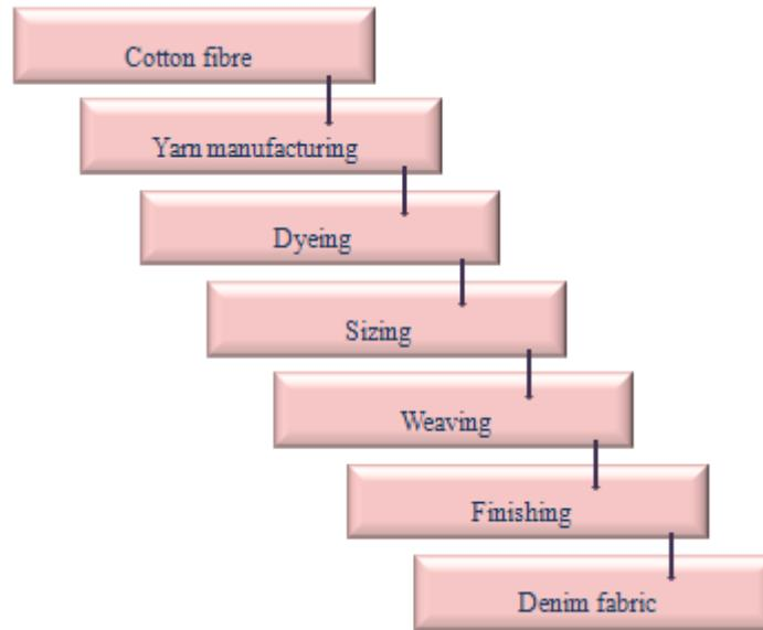
Figure 4.2: Process scheme inside the mill
