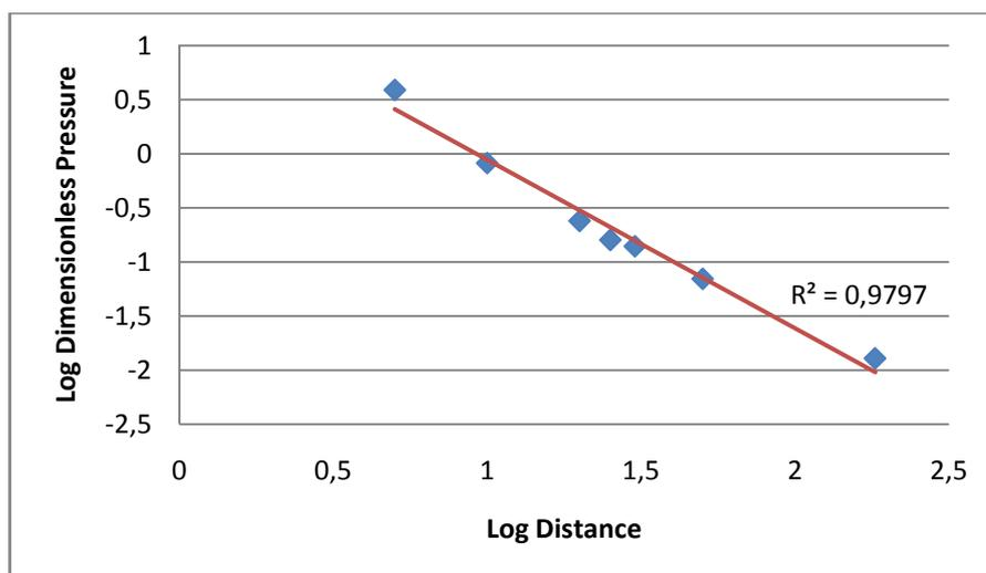
Figure C.2: Side-on overpressure vs. distance
