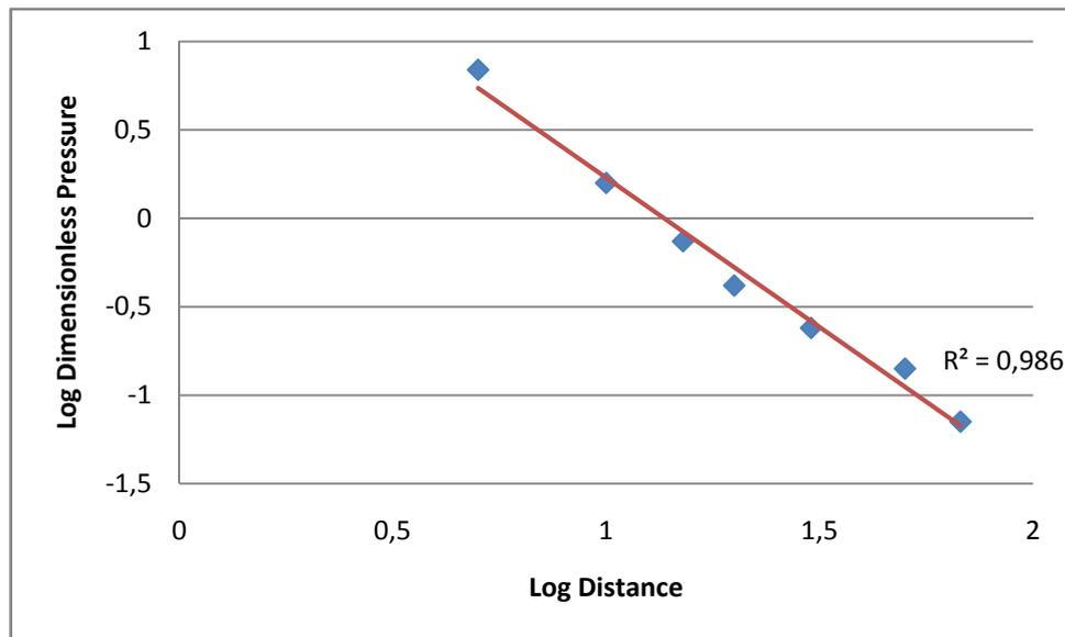
Figure 7.1: Side-on overpressure vs. distance
