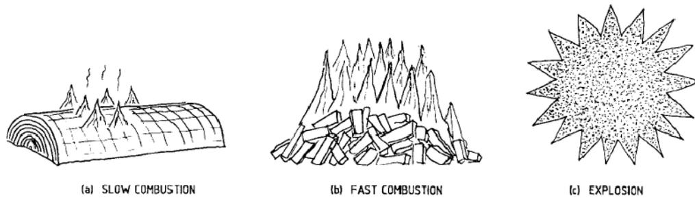
Figure 2.7: As surface area of solid substance increases, combustion rate increases [56]
