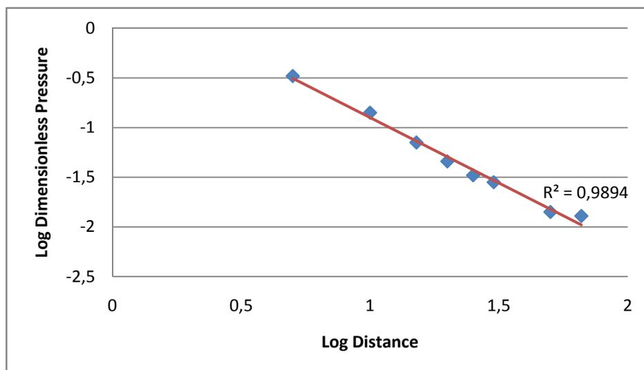
Figure C.3: Side-on overpressure vs. distance
