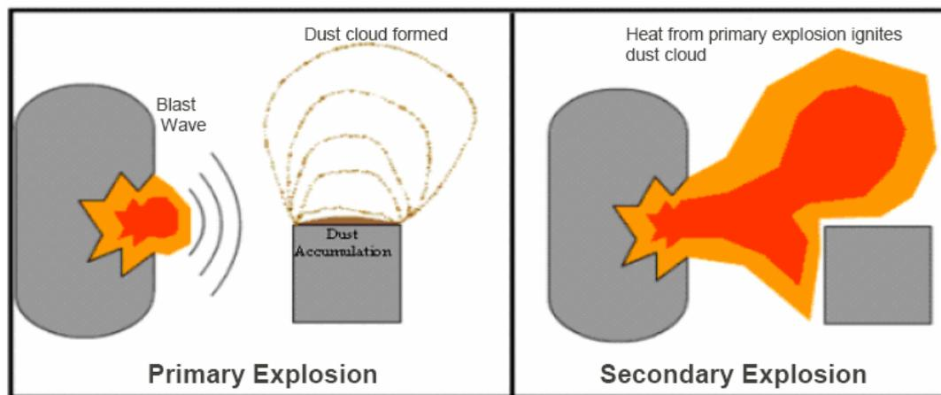
Figure 2.8: Primary and secondary dust explosion [62]
