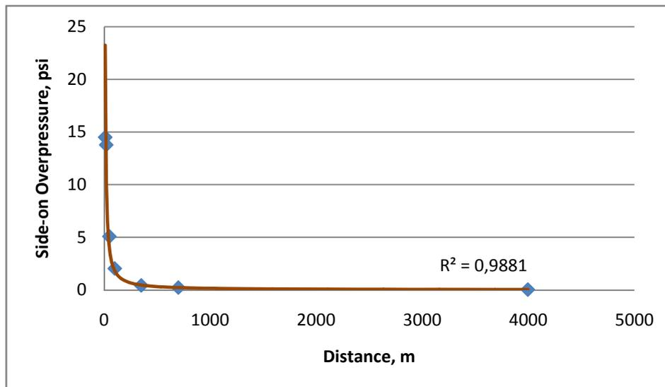
Figure 7.16: Side-on Overpressure vs. Distance
