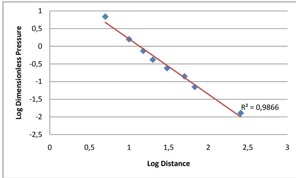
Figure 7.4: Side-on overpressure vs. distance
