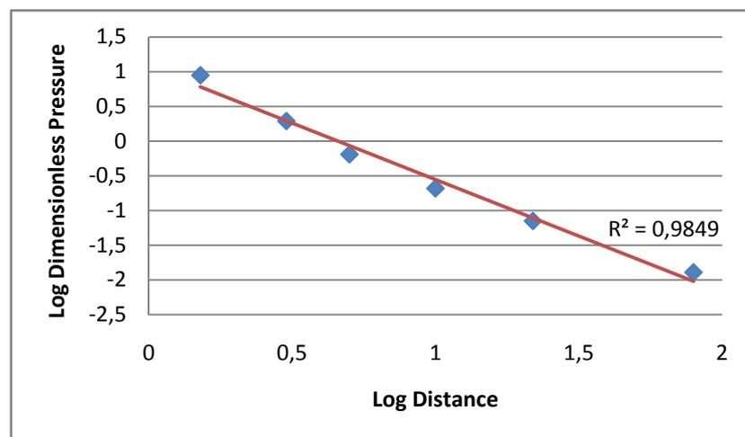
Figure 7.3: Side-on overpressure vs. distance
