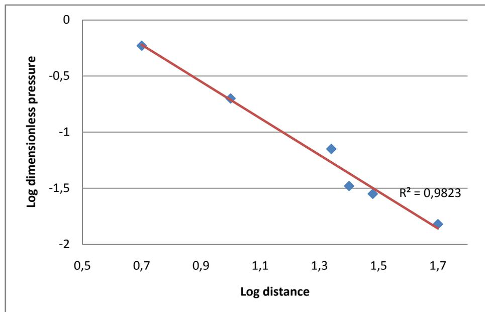
Figure C.1: Side-on overpressure vs. distance
