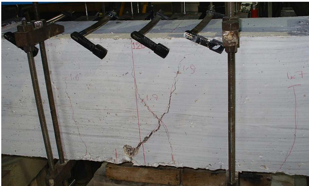
Figure 3.9 Crack pattern of A1 after failure
