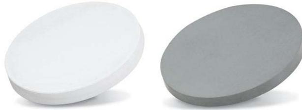
Figure 3.2 The targets used in the experiments: Al<sub>2</sub>O<sub>3</sub> (left) and Si (right)
