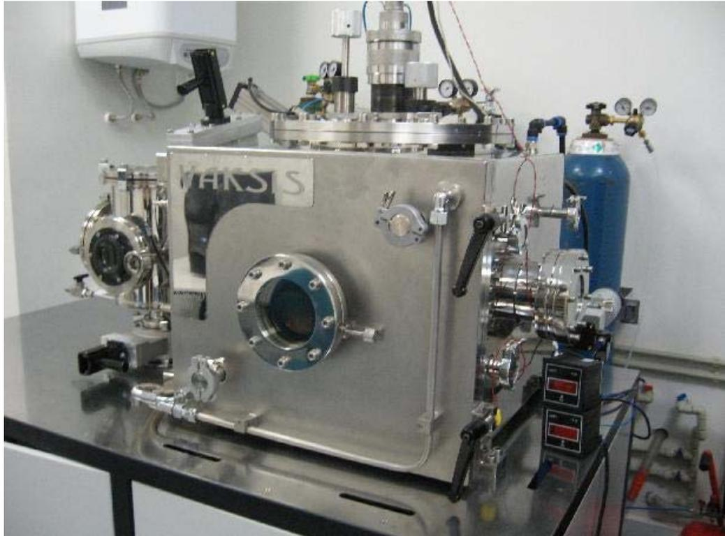
Figure 3.1. Main chamber of the sputter deposition system located in Semiconductor Material & Device Fabrication Lab.
