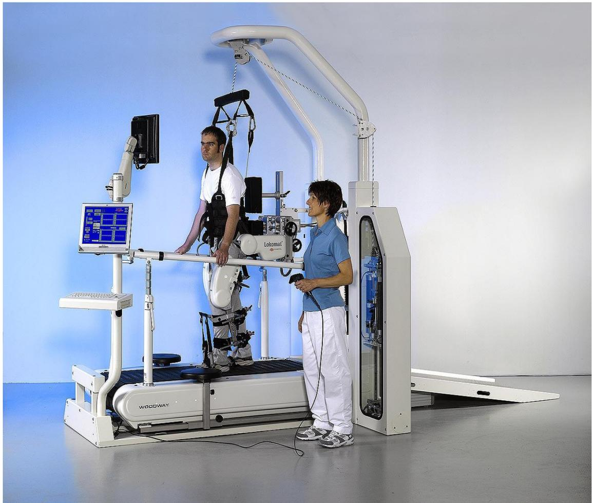
Figure 3.4 The driven gait orthosis Lokomat [16].
