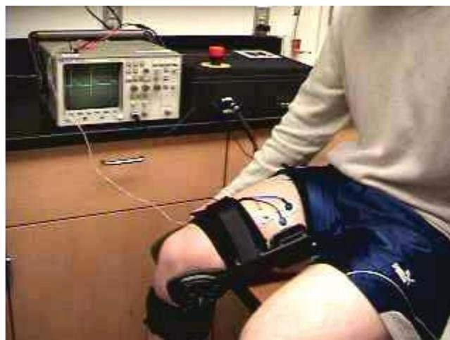
Figure 3.1 Human subjects wearing the instrumented biofeedback knee device [14].
