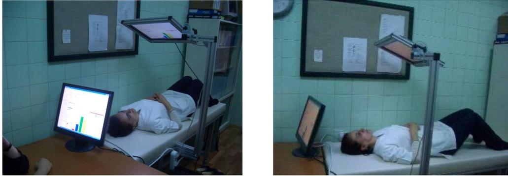
Figure 4.2 Manufactured Exercise Bed and Positions of the Monitors
