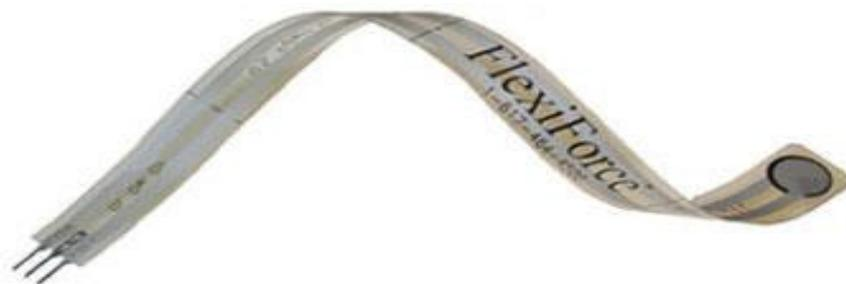
Figure 4.4 Force Resistive Sensor [28].
