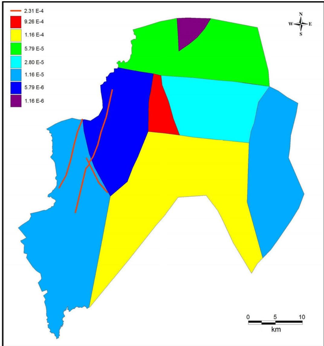
Figure 5.2 Distribution of hydraulic conductivity of Ulubey aquifer within the model domain (m/s)
