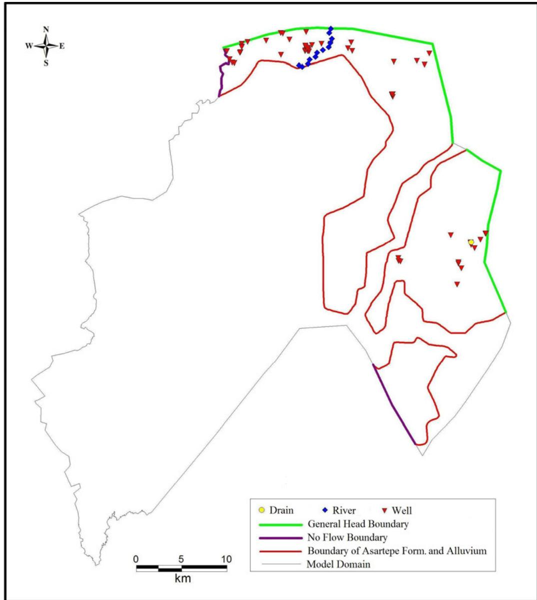
Figure 4.4 Boundary conditions of Asartepe and alluvium aquifers
