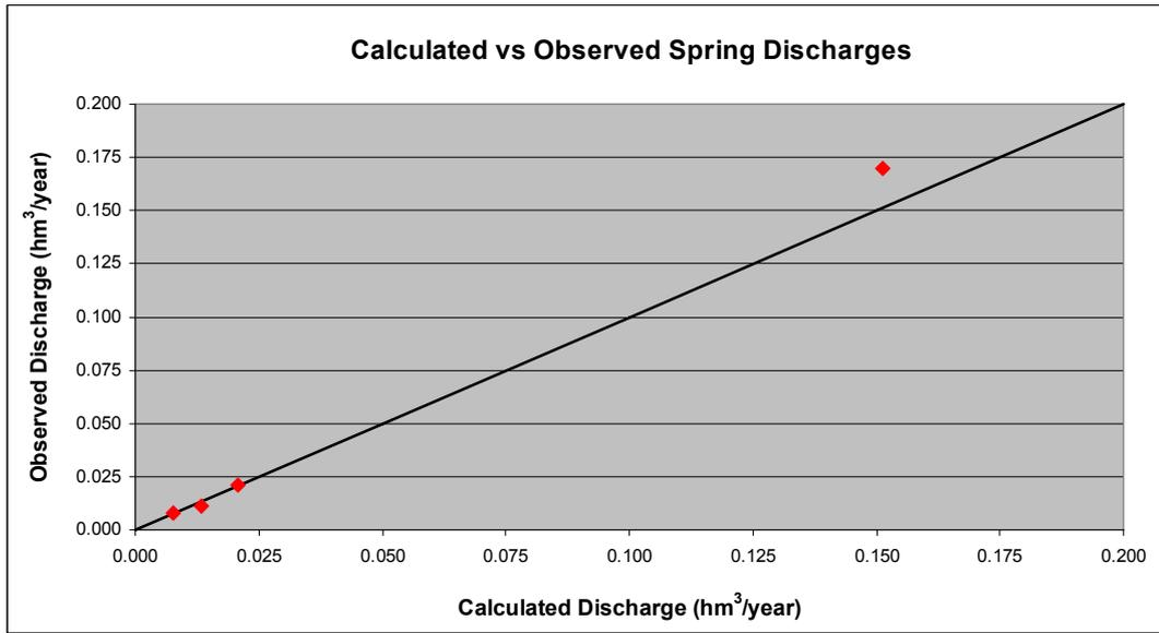
Figure 5.7 The graphical relation between calculated and observed spring discharges
