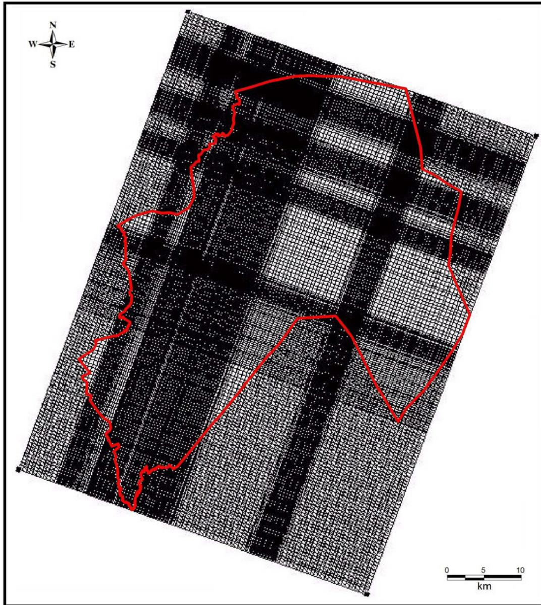
Figure 4.2 Groundwater flow model finite difference grid
