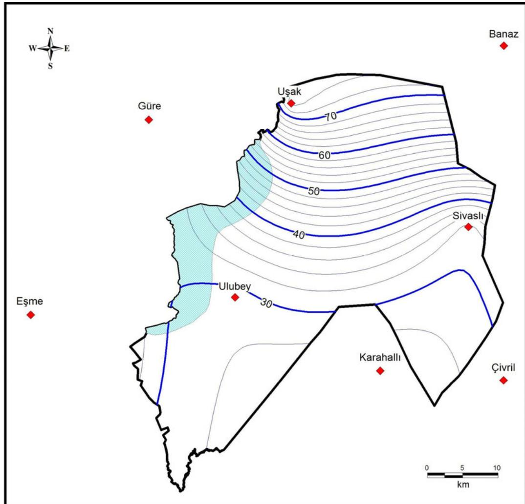
Figure 5.1 Areal distribution of recharge within the model domain (mm/year) and meteorological stations for which recharge is calculated by Thornthwaite method
