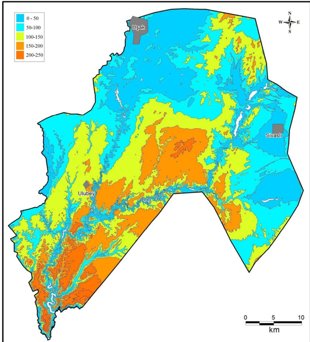
Figure 3.30 Depth to static groundwater level map of Ulubey aquifer
