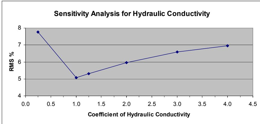
Figure 5.10 Results of sensitivity analysis for hydraulic conductivity
