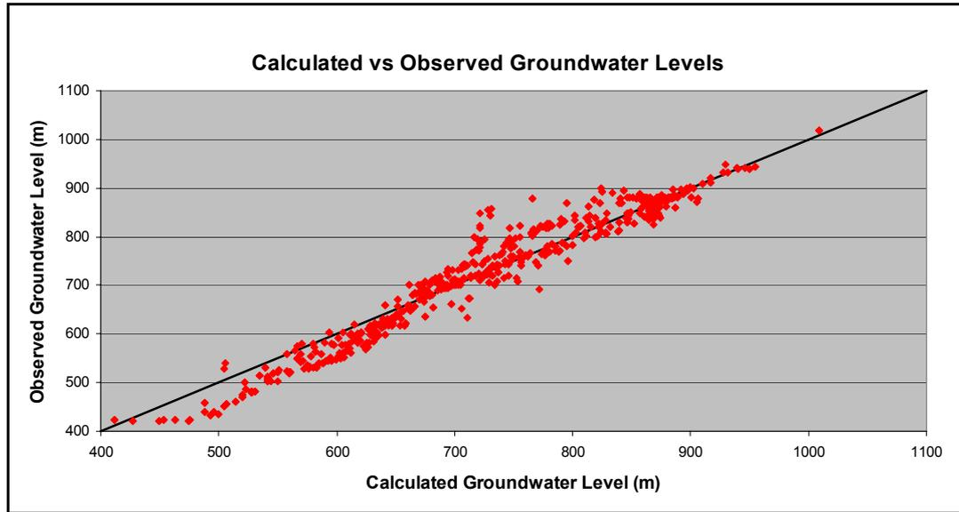
Figure 5.6 The graphical relation between calculated and observed groundwater levels
