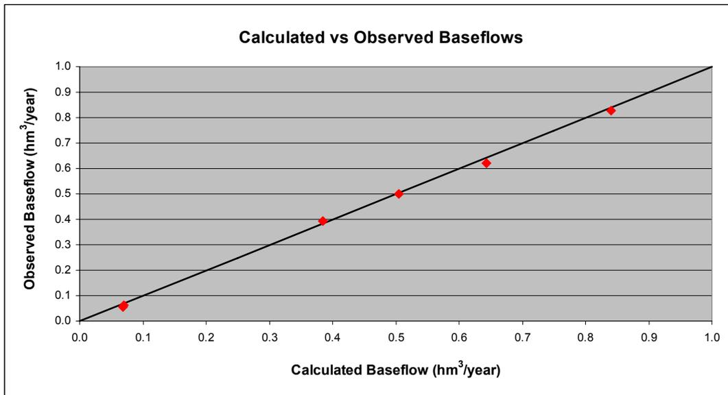
Figure 5.8 The graphical relation between calculated and observed baseflows
