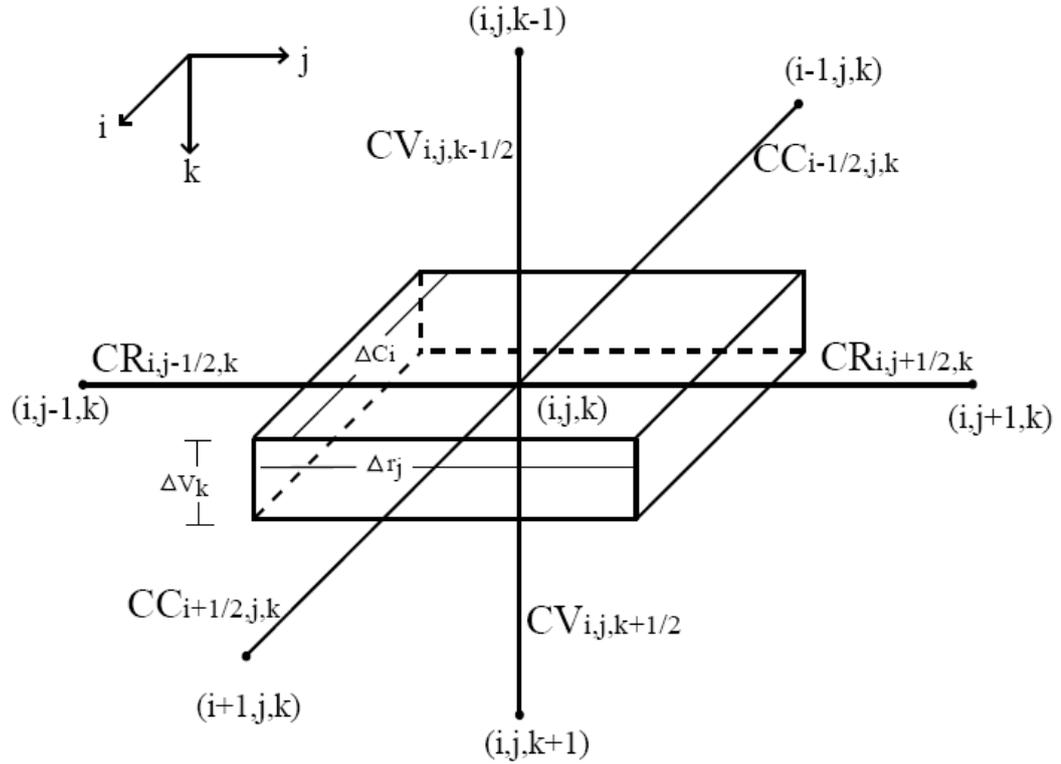
Figure 4.1 Definition of conductance terms between model cells
