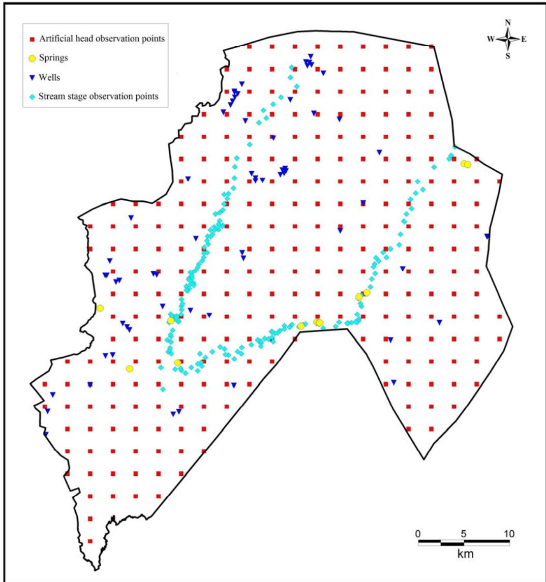
Figure 5.3 The points for which observed and calculated groundwater levels are compared during calibration
