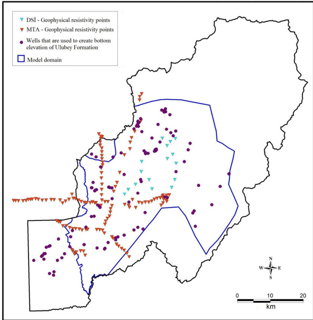
Figure 3.18 Locations of geophysical resistivity points and wells which are utilized to create bottom elevation map of Ulubey Formation
