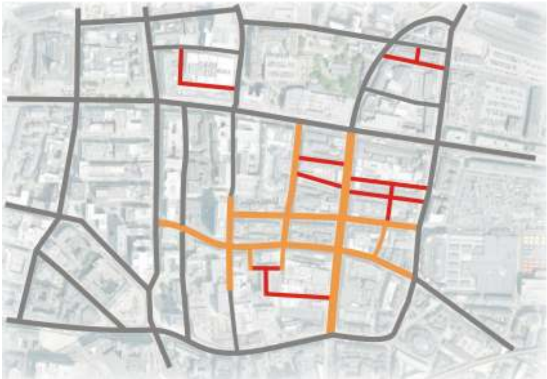
Figure 3.19. Communication network of Leeds commercial district (Grey indicates vehicle roads, orange indicates pedestrian ways, red indicates arcades and covered corridors)
