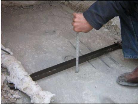
Figure 3.14 Spalling of Specimen (Test 2)
