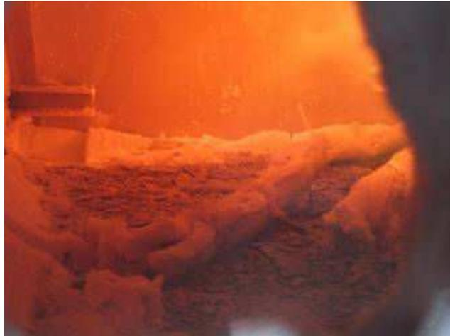
Figure 3.10 Concrete Face and Inside of Furnace (Test 3)
