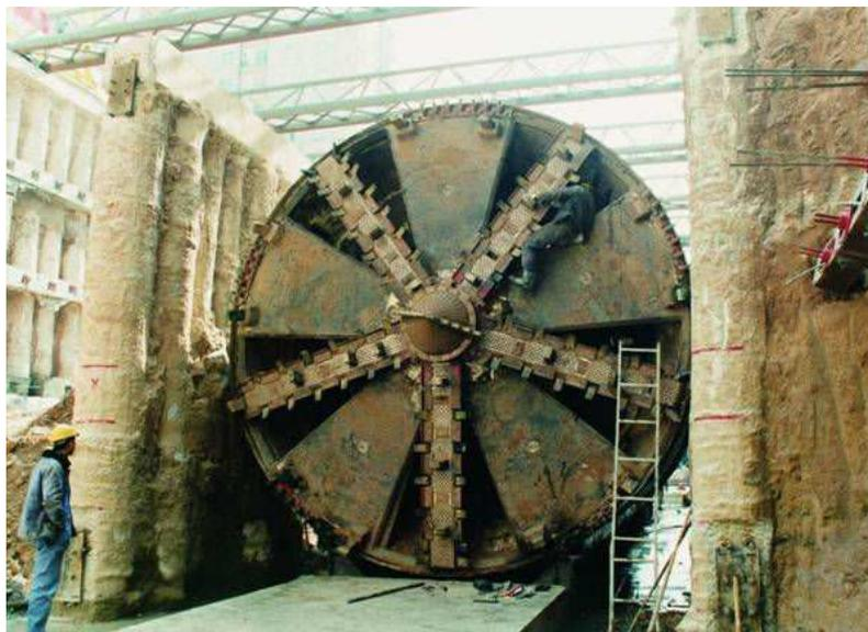
Figure 1.4 TBM Cutting Head [8]
