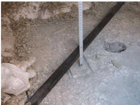
Figure 3.15 Spalling of Specimen (Test 3)
