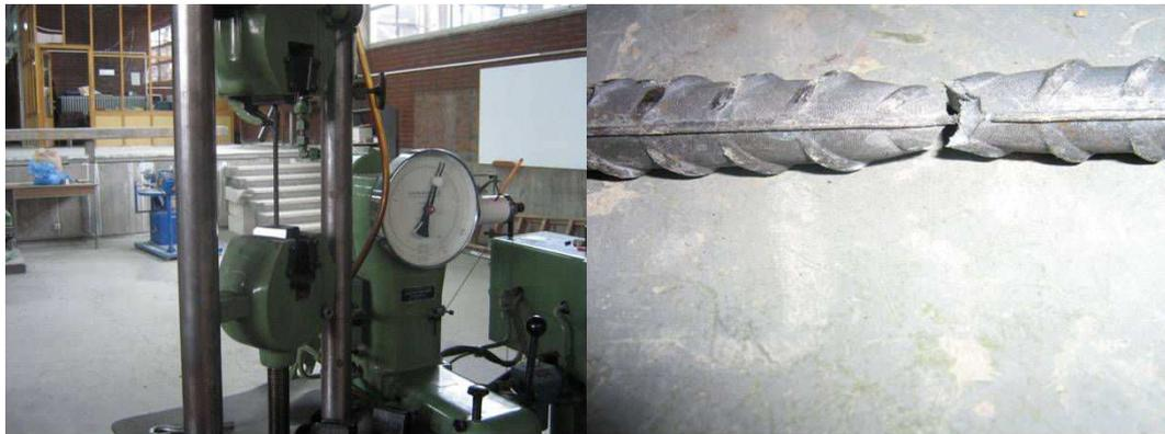
Figure 3.3 Tensile Strength Tests of Reference Segment
