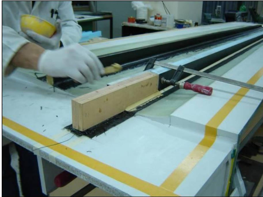
Figure 12: Hornbeam section of the front spar
