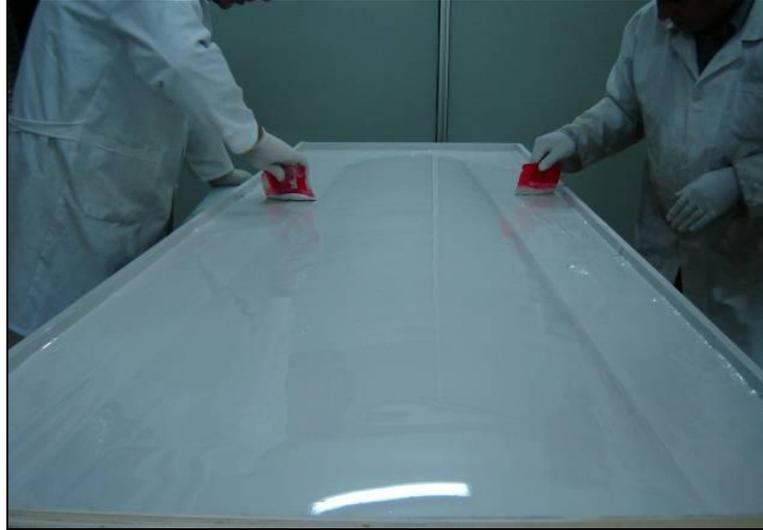
Figure 6: Covering the male mold with tool resin
