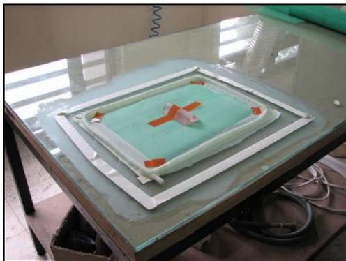
Figure 57: VARTM setup before covering with vacuum bag
