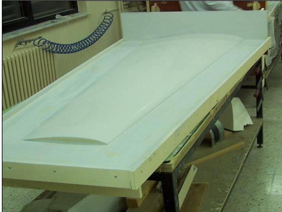
Figure 5: Male mold ready to be used as reference for female mold manufacturing
