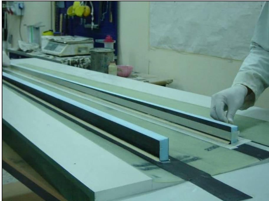
Figure 10: Positioning the spars
