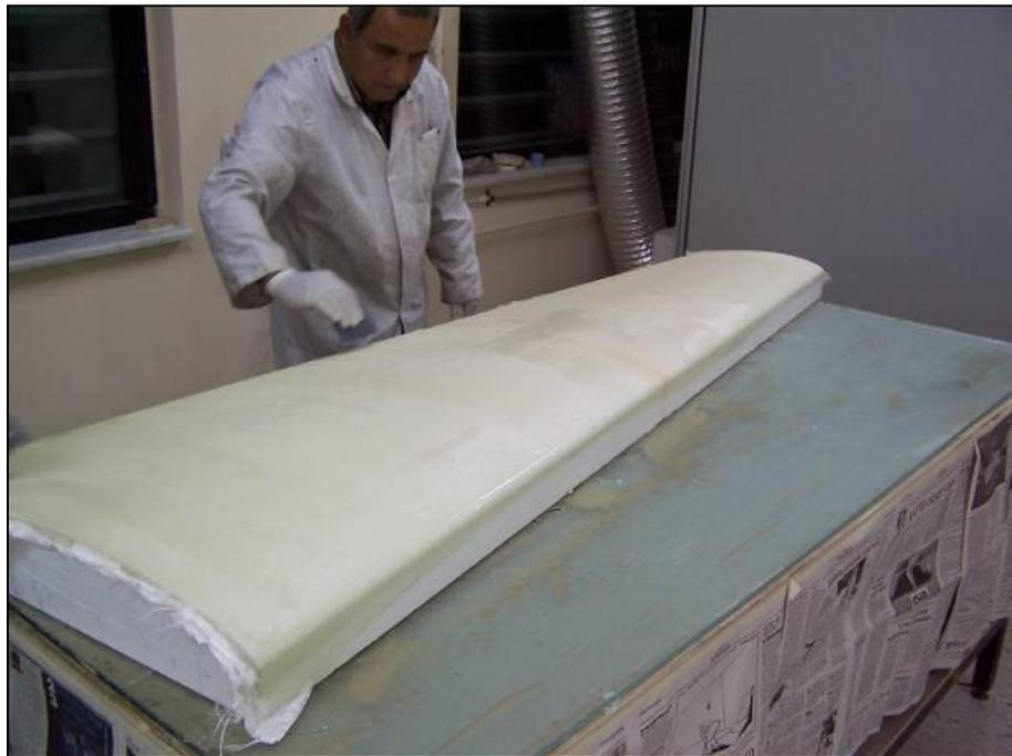
Figure 4: E-Glass coated polystyrene foam used in the manufacturing of the METU TUAV wing
