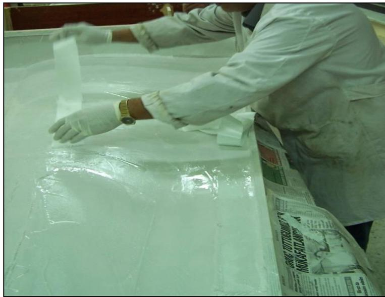
Figure 7: Reinforcing the mold with woven E-glass woven fabric
