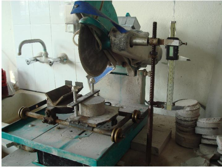
**Figure 5.5** Opening of notch in Smartcut 1004
