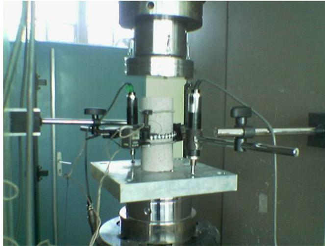
**Figure 5.1** UCS test: andesite specimen with circumferential and axial extensometer
