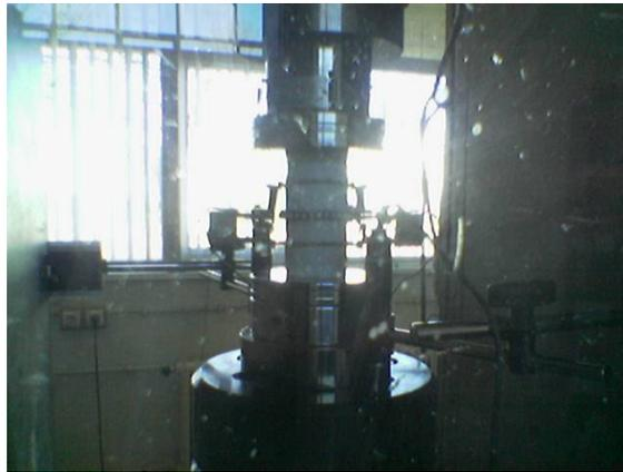
**Figure 5.2** UCS test marble specimen with circumferential and axial extensometer
