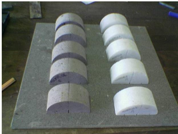
**Figure C.3** Andesite and marble SCB specimens after experiments
