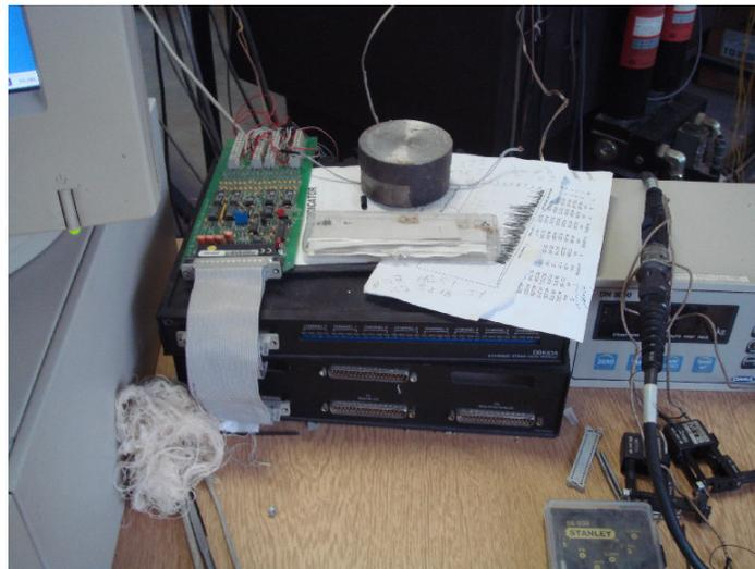
**Figure 5.8** DBK80 Analog Multiplexer, DBK43 and DBK43A strain-gage cards
