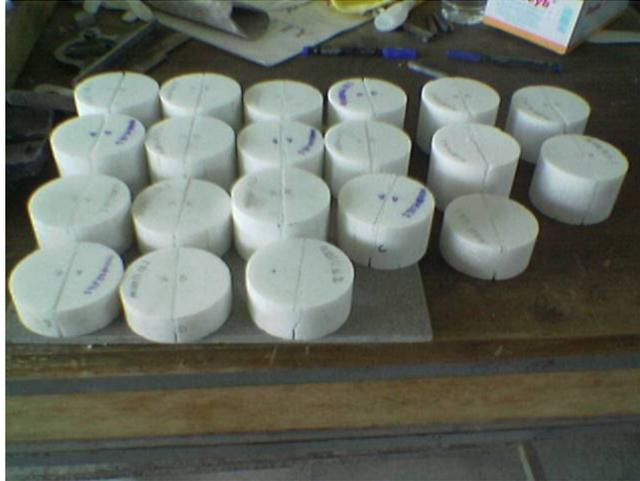
**Figure C.2** Marble SNDB specimens after experiments
