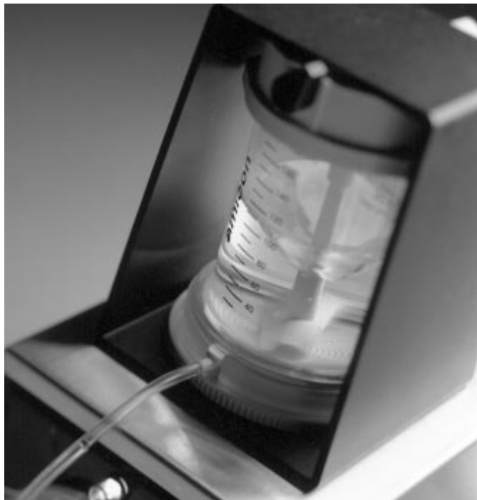
Figure 5.2. Microfiltration and Ultrafiltration Test Apparatus
