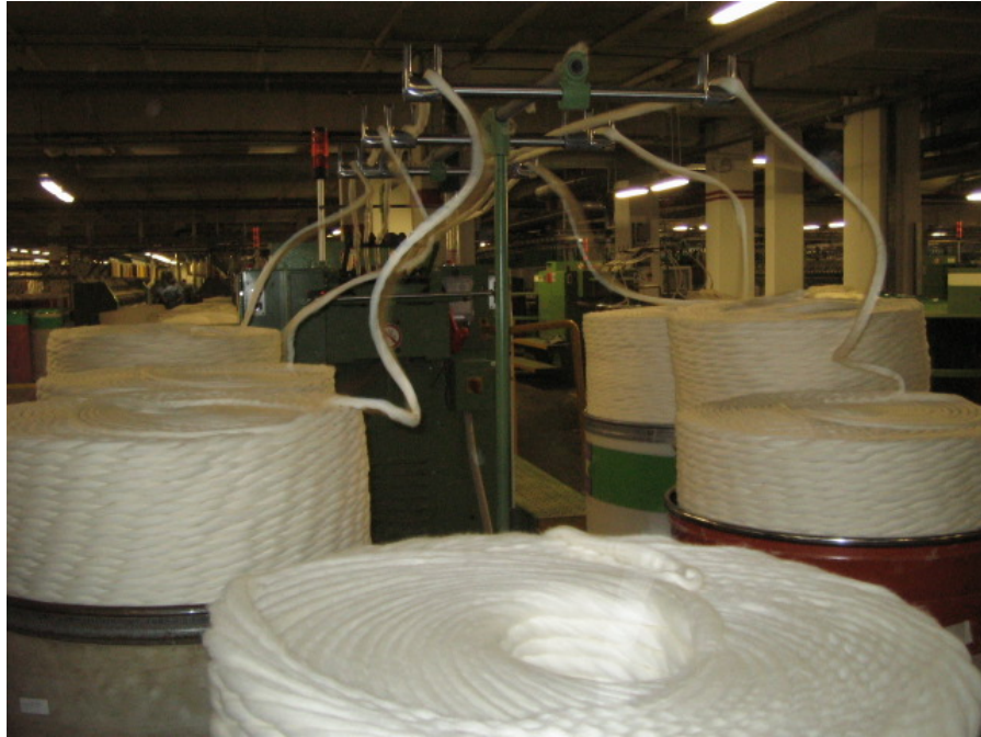
Figure 4.3. Drawing Process in which thick strips are formed
