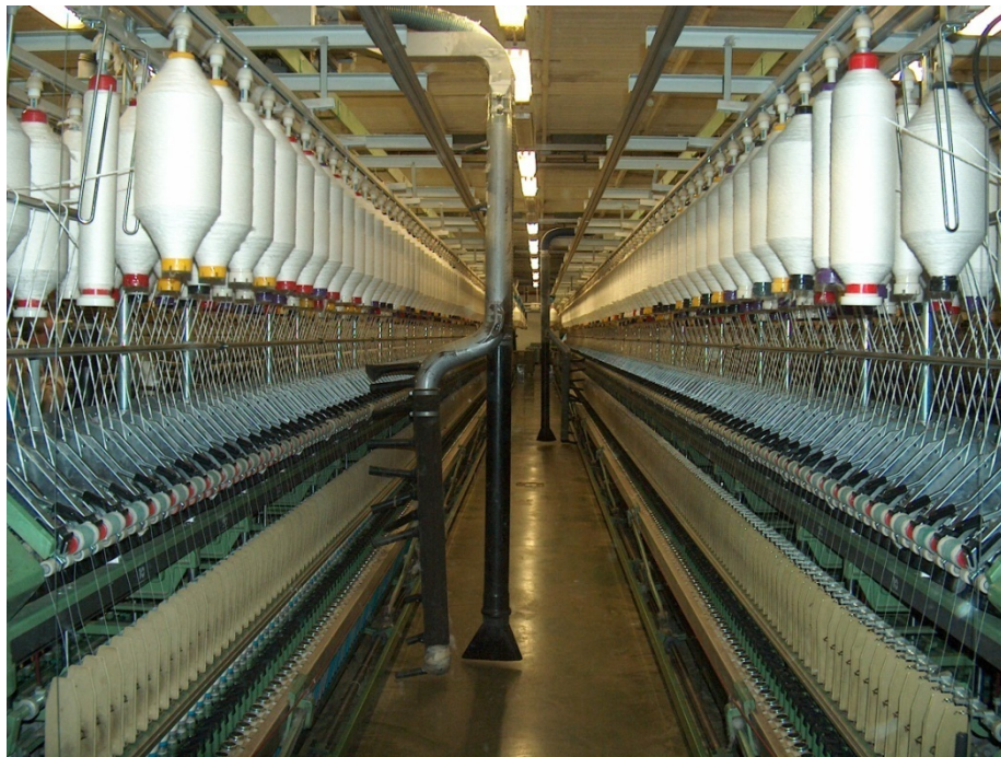
Figure 4.4. Spinning Process in which final thickness of the yarns are provided
