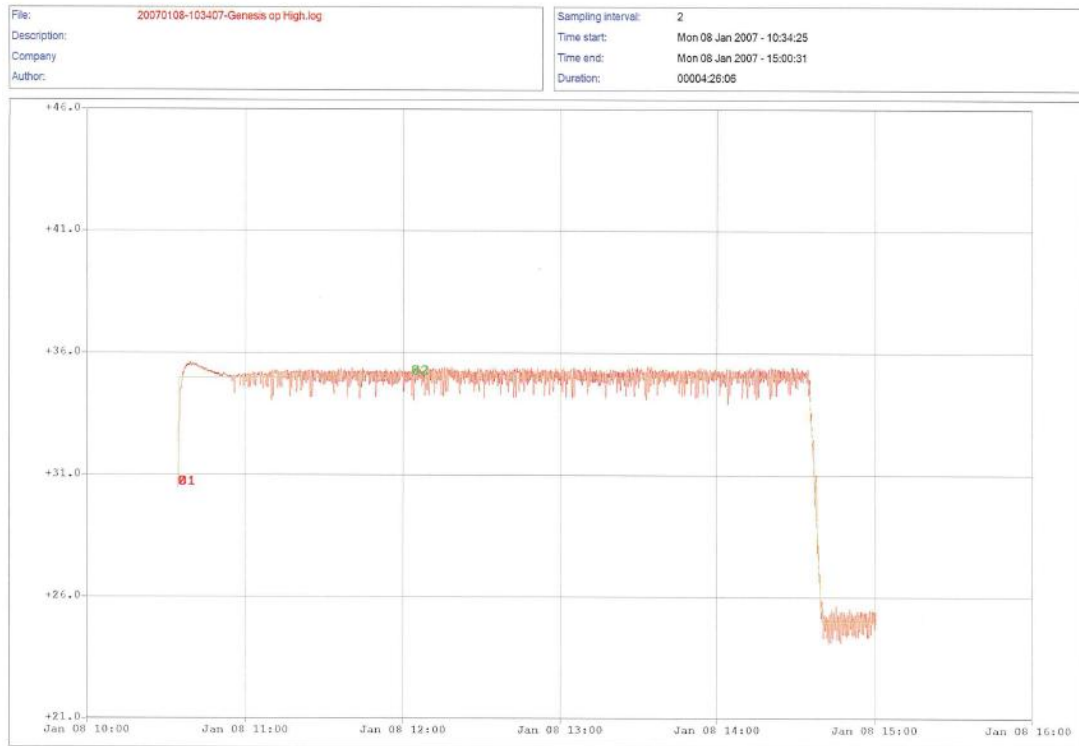
Figure 5.21 Thermal chamber obtained data during operational high temperature test
