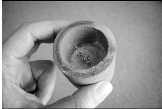
Figure B1 A sample cylindrical thermal analysis cup with three thermocouples placed at three different radial locations.
