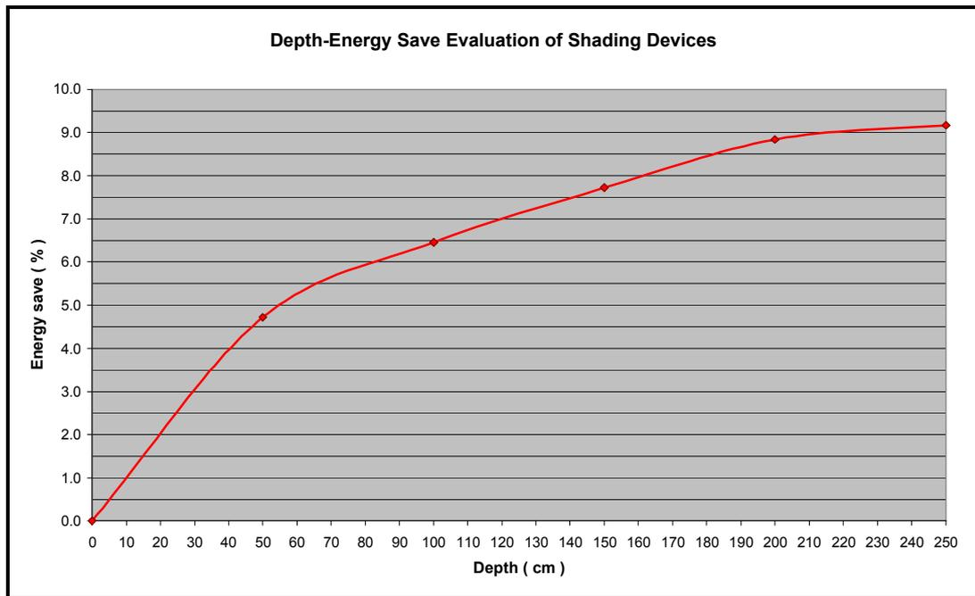
**Figure 4.11** Depth vs. energy savings chart of shading devices
