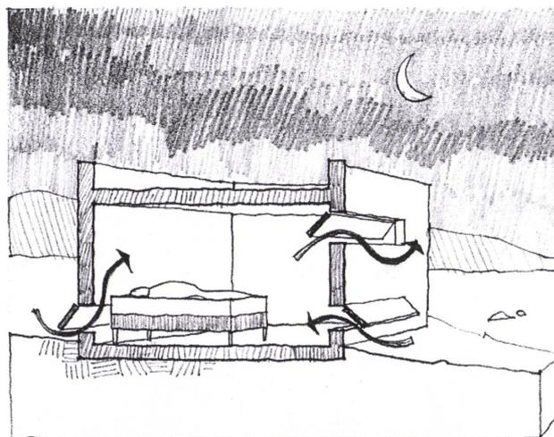
**Figure 2.09** Nocturnal ventilative cooling
