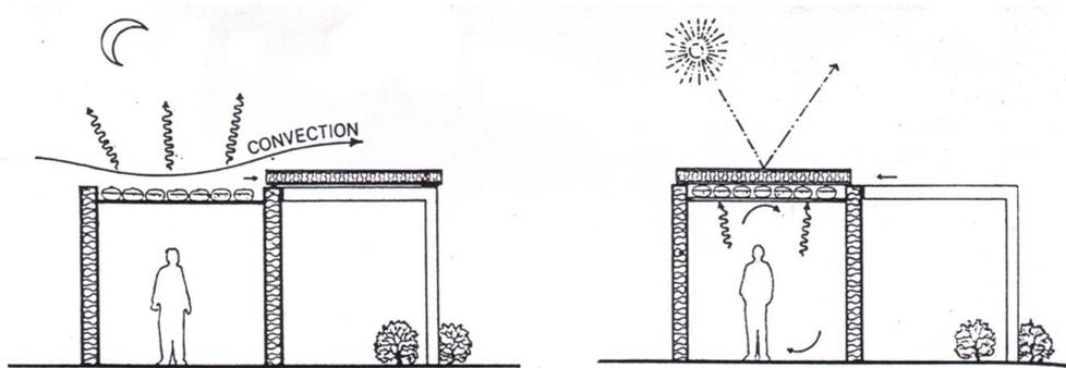
**Figure 2.10** Direct radiative cooling system
