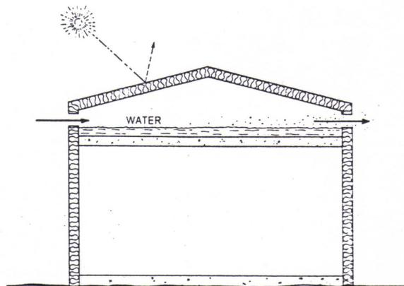
**Figure 2.14** Roof pond system with fixed insulation
