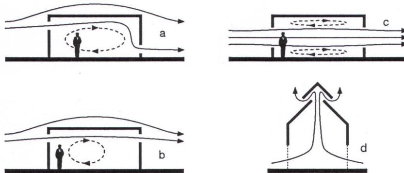
**Figure 2.03** Basic air flow principles, (ii)
