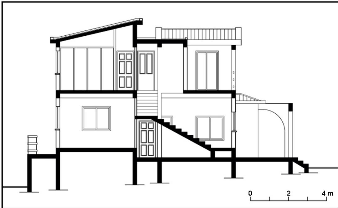
**Figure A.05** Section A-A of case study building
