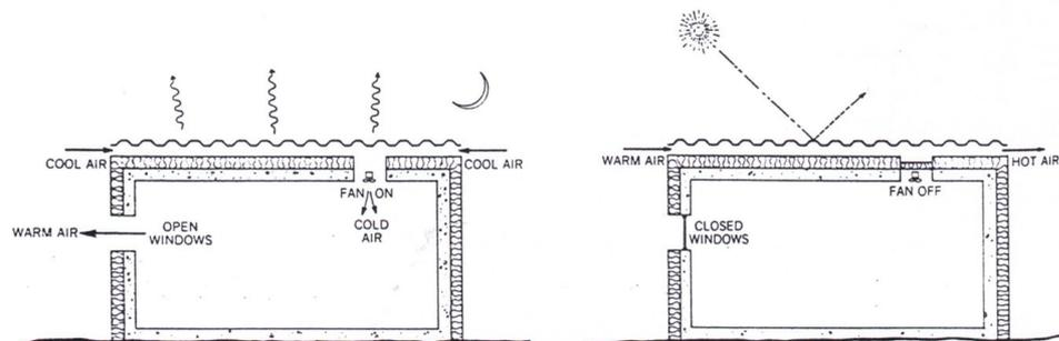
**Figure 2.11** Indirect radiative cooling system
