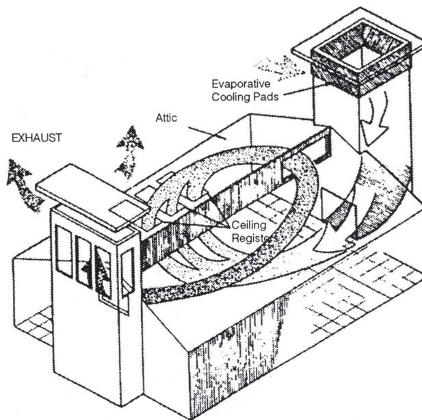
**Figure 2.13** Evaporative cooling towers
