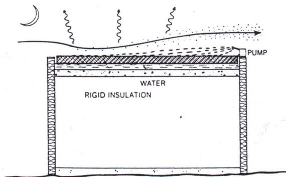
**Figure 2.15** Roof pond system with floating insulation
