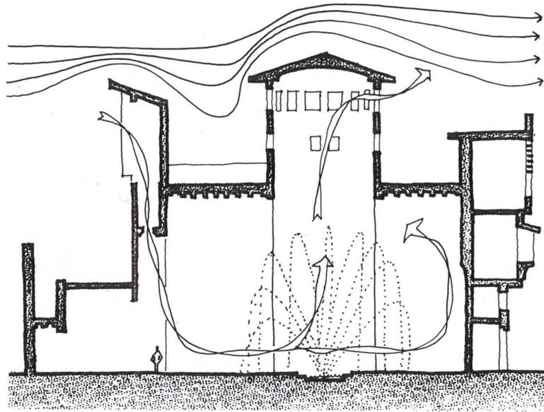
**Figure 2.12** Direct evaporative cooling with the use of an interior fountain
