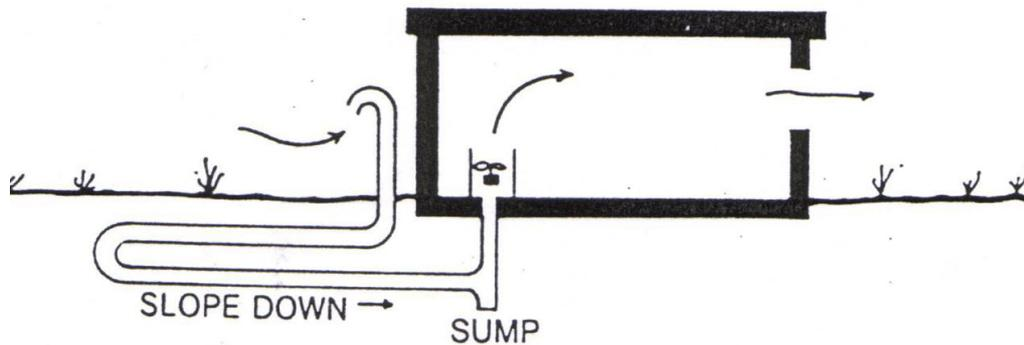
**Figure 2.18** Indirect earth cooling system with pipes
