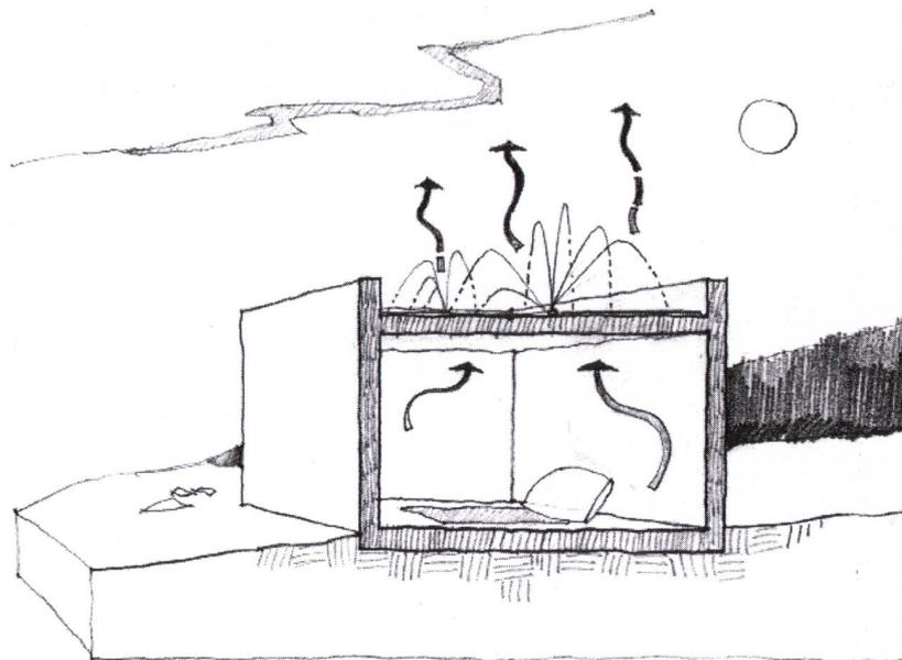
**Figure 2.16** Roof sprinkling systems for cooling
