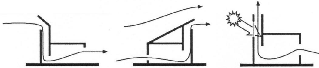
**Figure 2.07** Basic air flow principles, (vi)
