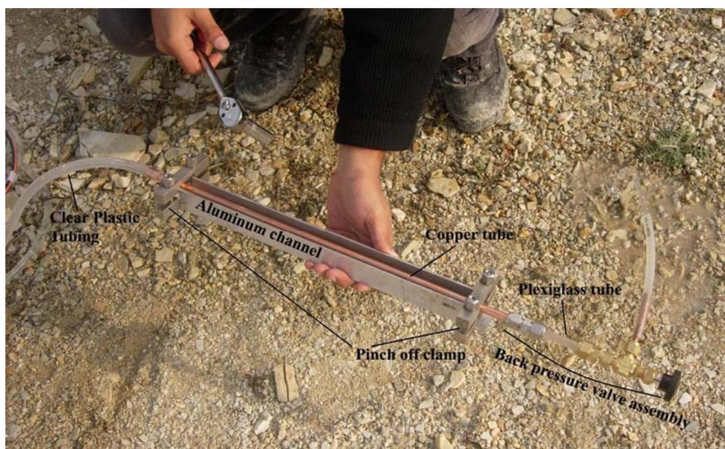
Figure 4.2 The equipment used to take noble gas samples.
