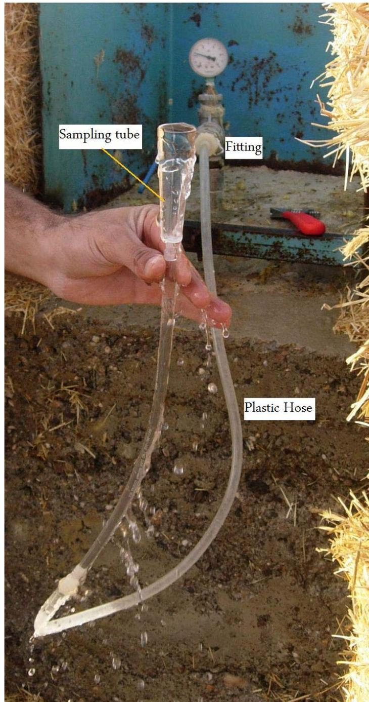
Figure 4.1 Sampling for Dissolved Oxygen.
