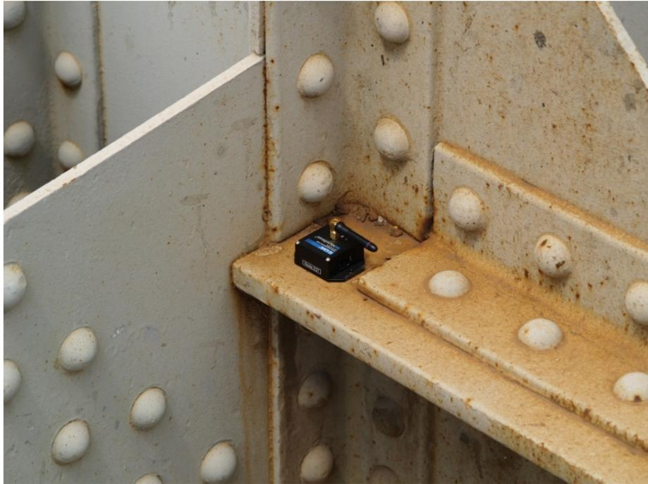
**Figure 3.3** A wireless accelerometer node
