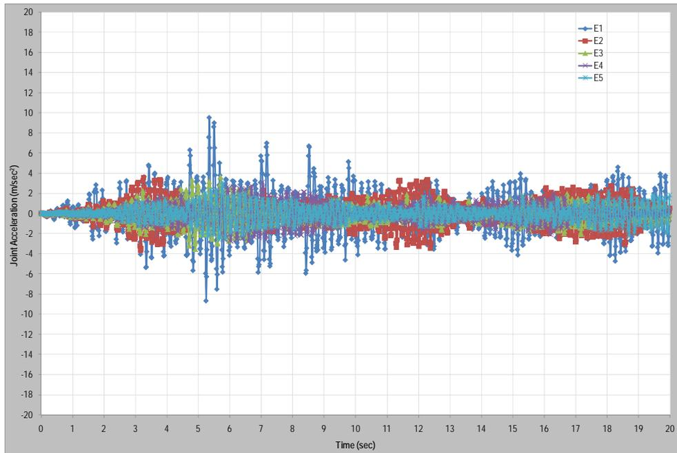
**Figure A.70** Combined Joint acceleration vs. time graphic of analysis models with a speed of 70 m/sec
