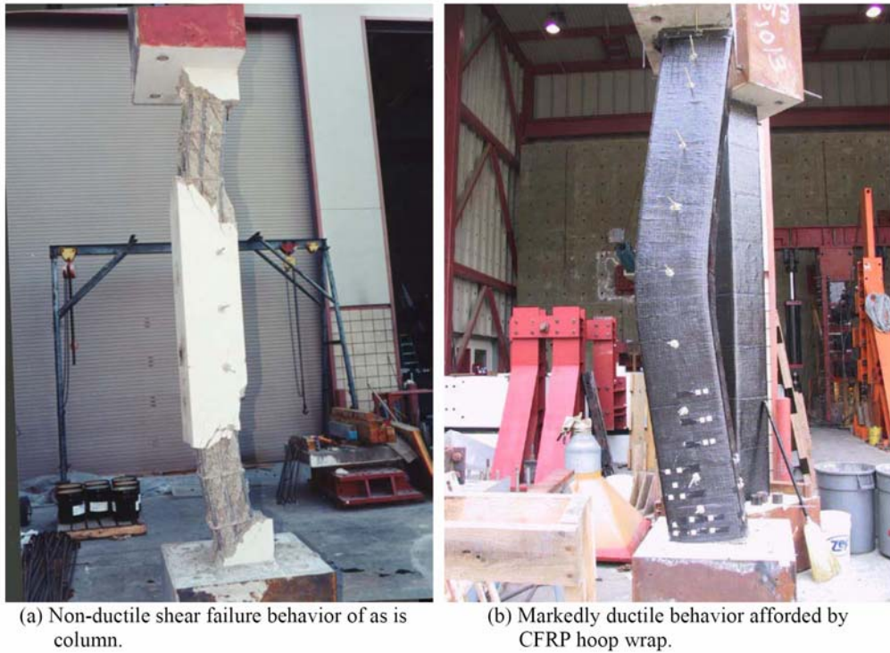
Figure 2.18 Behavior under statically applied simulated blast load for RC columns typical of an East Coast building [20]
