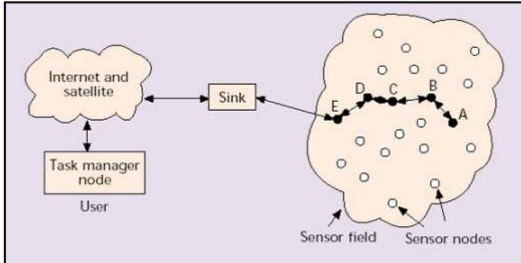
Figure 2.1: A common sensor network architecture (Akyildiz et al., 2002)
