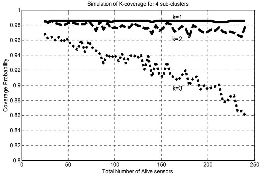
Figure 5.6: Simulation results for  $k$ -coverage probability
