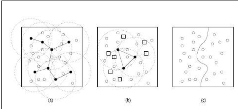
Figure A1: Area coverage (a), Point coverage (b) and Barrier coverage (c) (Cardei & Wu, 2006)
