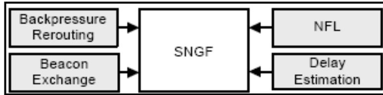
Figure 2.3: Routing components of SPEED (He et al., 2003)
