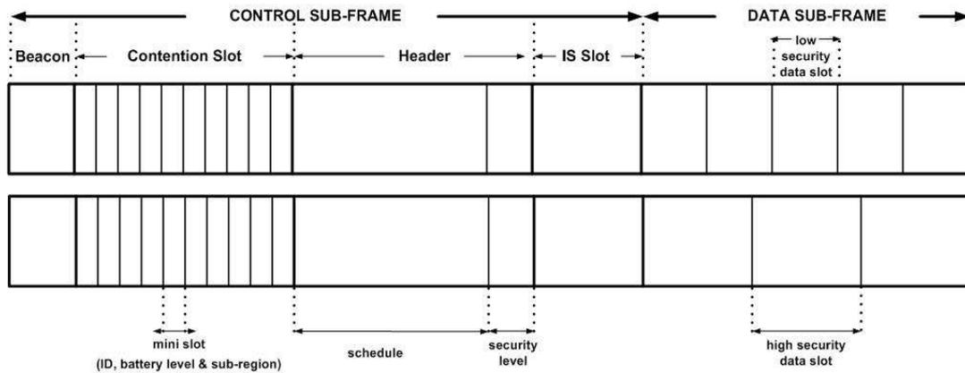
Figure 6.1: Frame format for the new method's MAC frame
