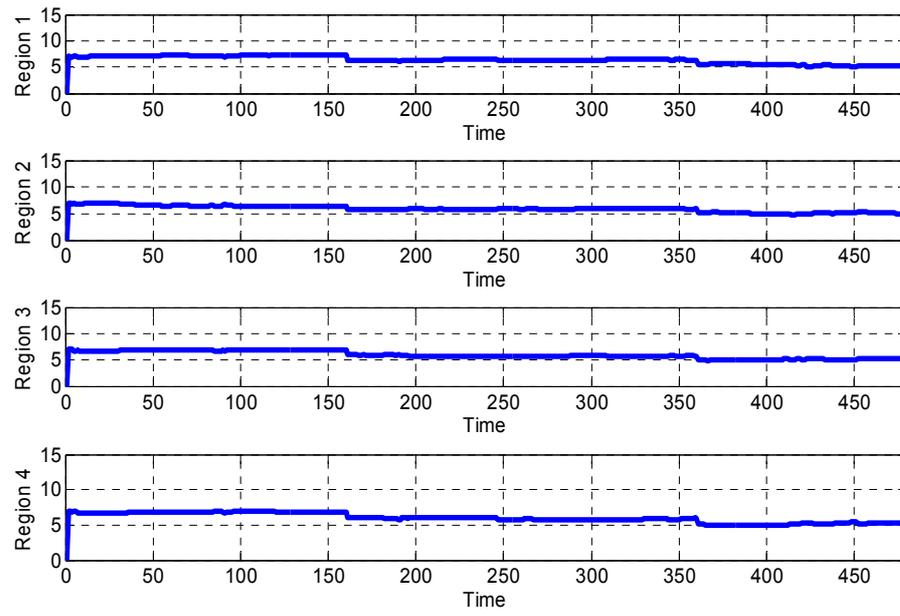
Figure 5.8: Distribution of active sensors on sub-regions for the coverage-enhanced ACK-based method
