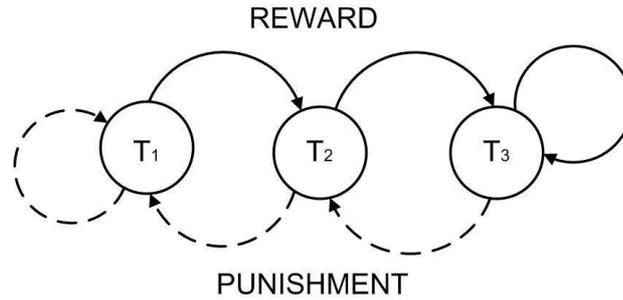
Figure 2.6: Finite state automaton for the ACK strategy of Kay and Frolik (2004)
