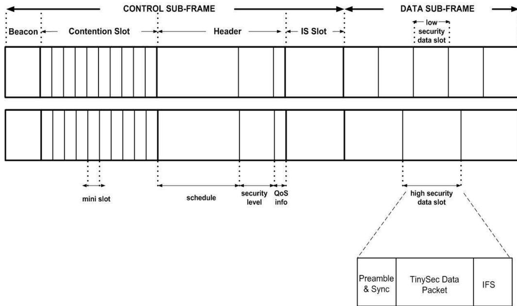
Figure 3.3: The frame format of the MAC scheme (2 frames are shown)
