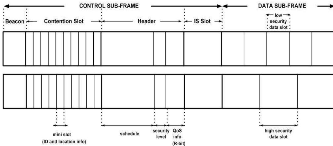
Figure 5.7: MAC Frame format of the coverage-enhanced ACK-based method (2 frames are shown)
