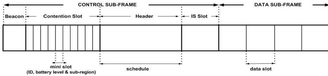
Figure 6.6: Frame format of the MAC scheme for the modified method
