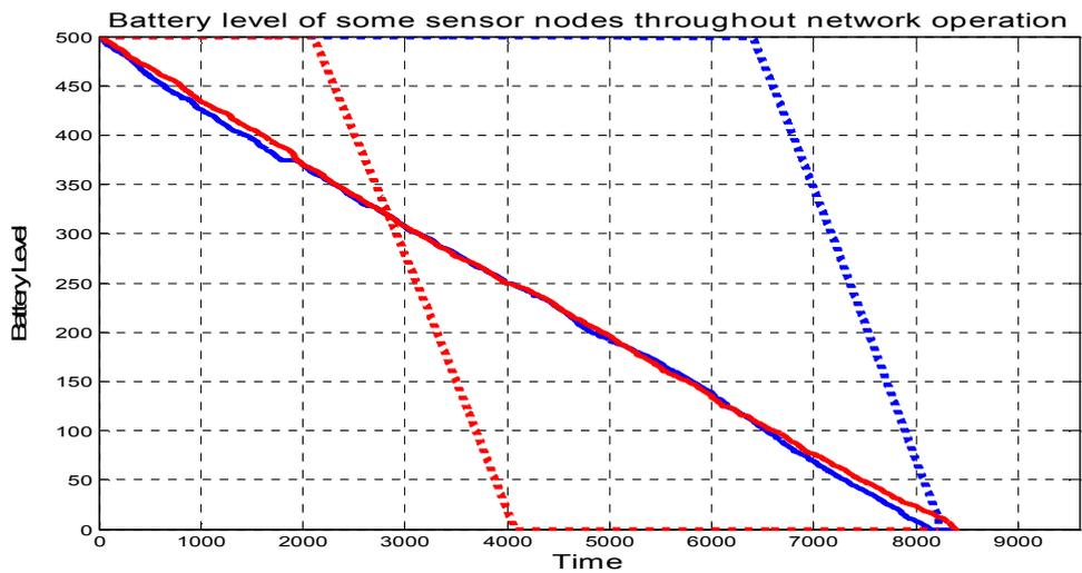
Figure 6.4: Battery level of nodes for both methods
