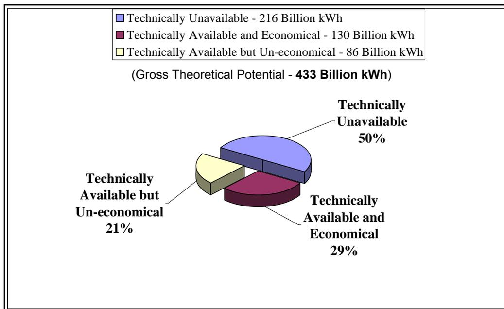
**Figure 2.6. Hydroelectric Potential of Turkey (Eroğlu, 2007)**
