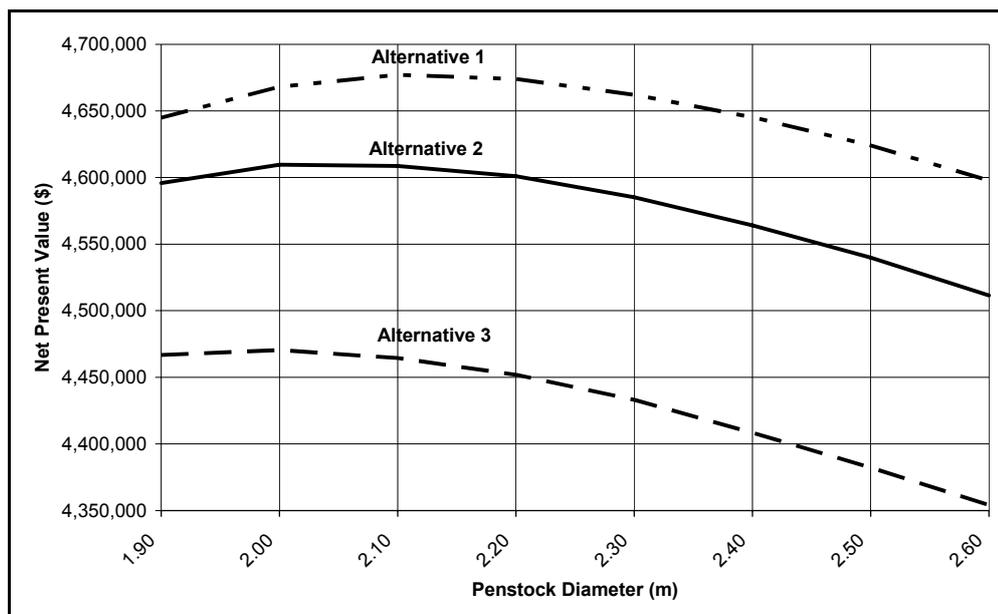
**Figure 6.3. Optimization of Penstock Diameters**
