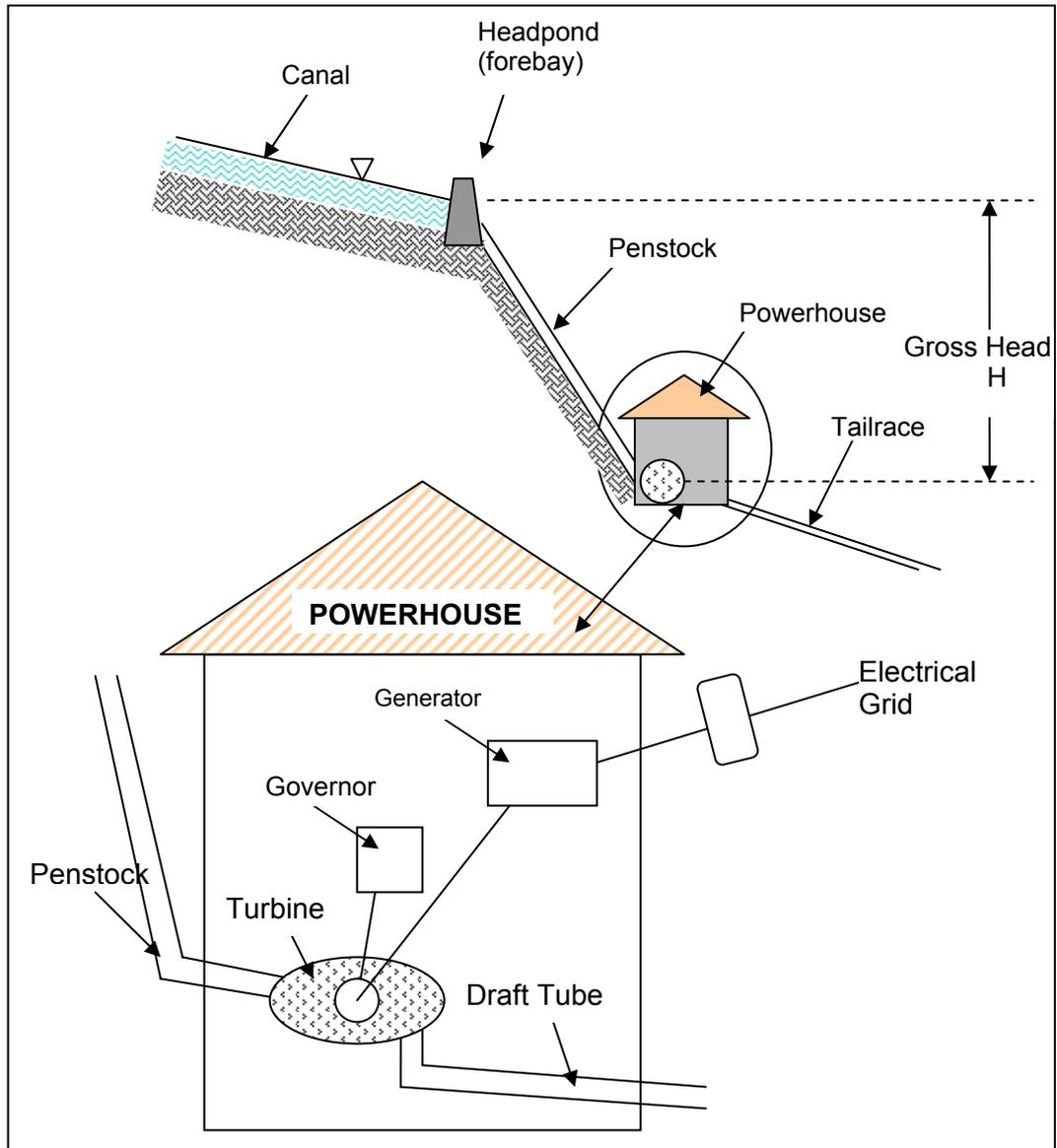
**Figure 2.2. Main Parts and Structures of Small Hydropower Site**
