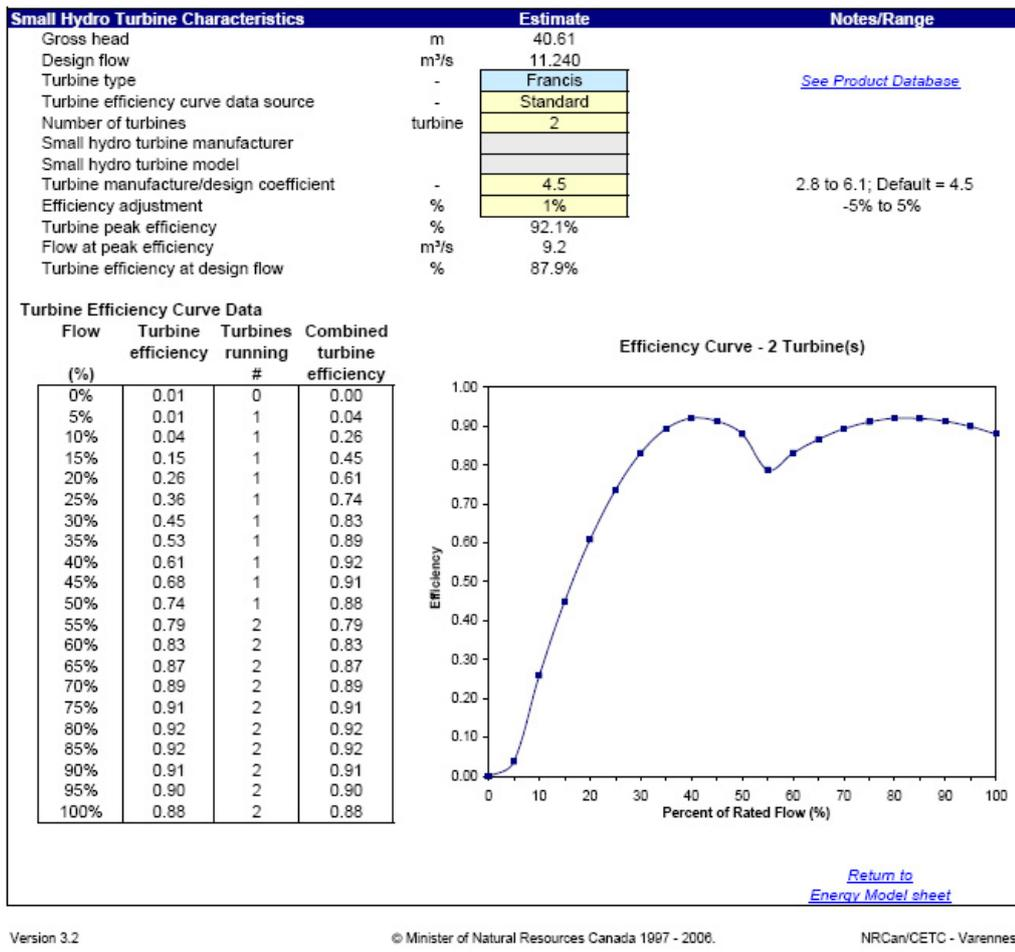
Figure F.3. "Equipment Data" Worksheet of Porsuk Dam ( $Q_d = Q_{25}$ )
