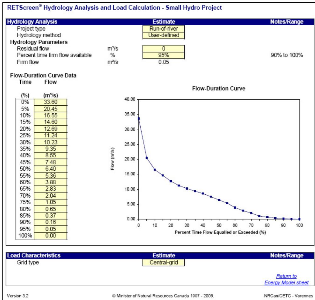
Figure F.2. "Hydrology Analysis and Load Calculation" Worksheet of Porsuk Dam ( $Q_d = Q_{25}$ )
