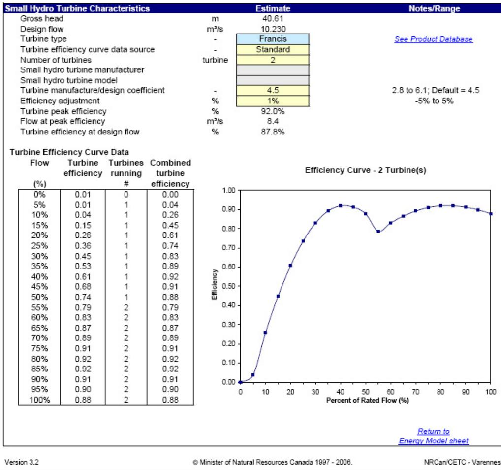
Figure G.4. "Equipment Data" Worksheet of Porsuk Dam ( $Q_d = Q_{30}$ )
