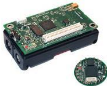
Figure 2.3: Mica and Mica2dot Motes
