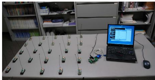
Figure 5.16: 5x5 mote test bed which is used in real experiments (Fok et al., 2006)
