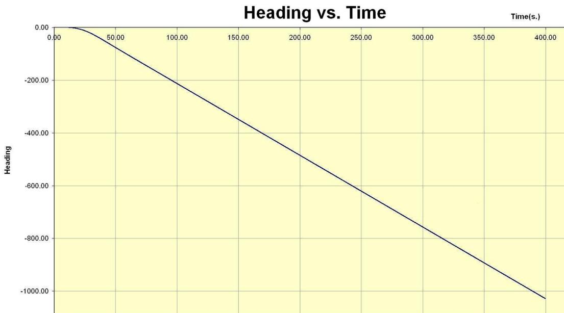
Figure 5.5: NSTMSS turning circle heading angle change
