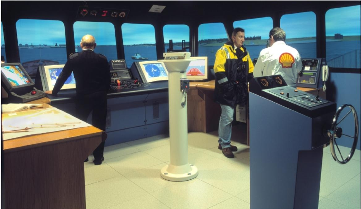
Figure 1.1: Lairside Maritime Simulator Bridge View
