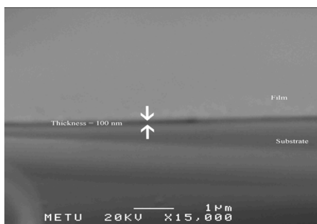
Figure 4.14 Cross sectional SEM image of a thin film prepared by main solution (S1) at 2000 rpm and sintered at 300 °C for 2 h in nitrogen atmosphere.
