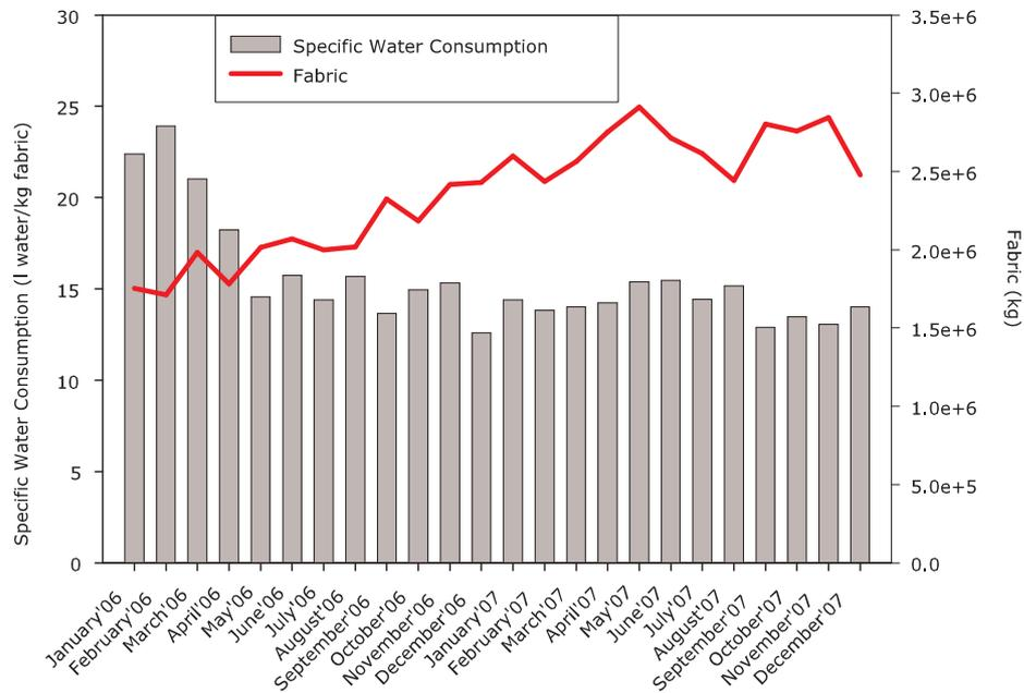
Figure 6.14: Overall specific water consumption and fabric production patterns in finishing process
