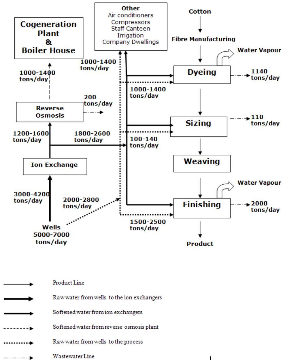
Figure 6.1: Water flow in the selected mill (as of 2005)
