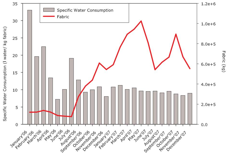
Figure A.9: Specific water consumption and fabric production patterns of M4
