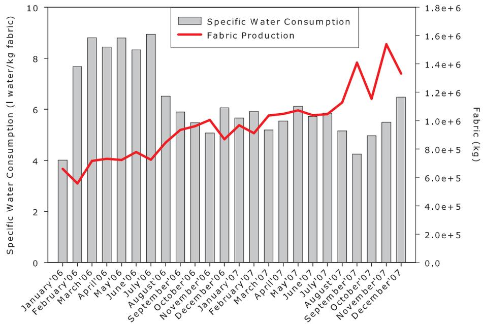
Figure 6.7: Specific water consumption and fabric production patterns in M7
