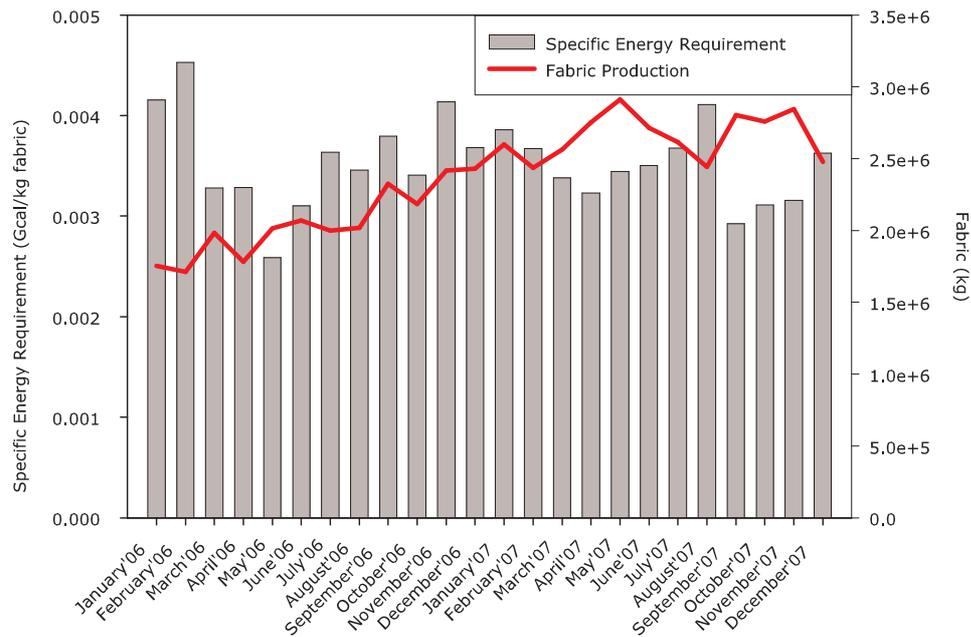
Figure 6.27: Specific energy requirement pattern in finishing process
