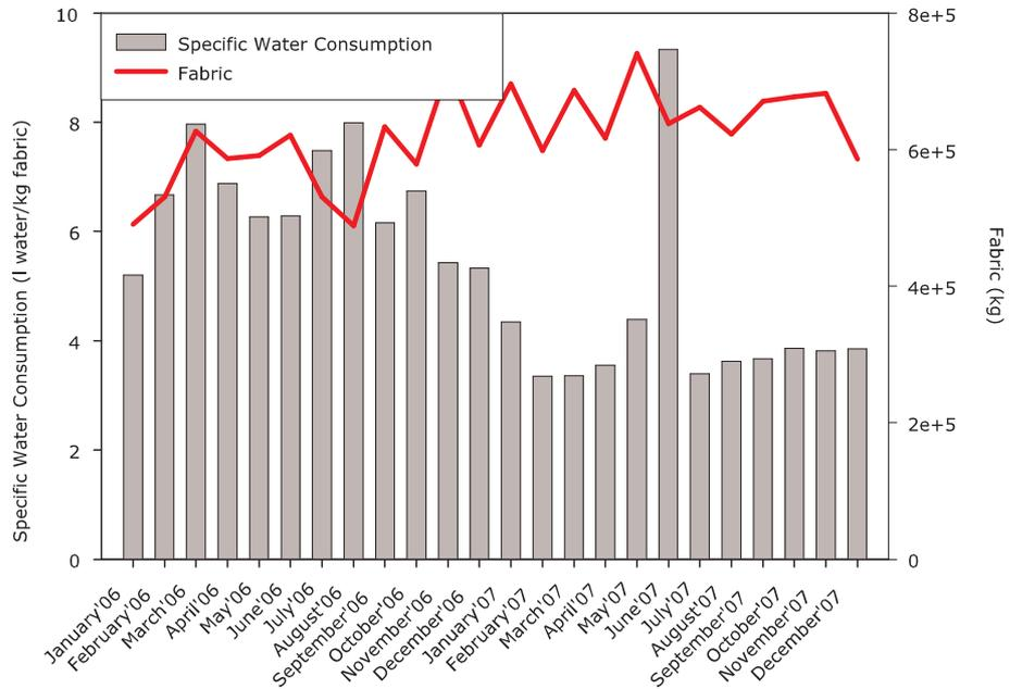
Figure A.11: Water consumption and fabric production patterns of M5
