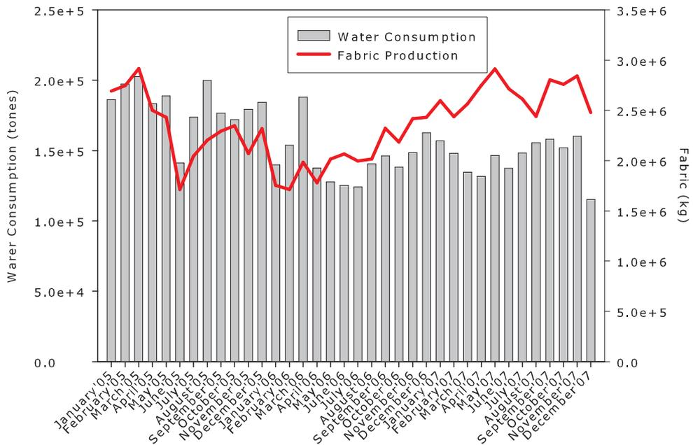
Figure 6.2: Water consumption and fabric production patterns in the mill
