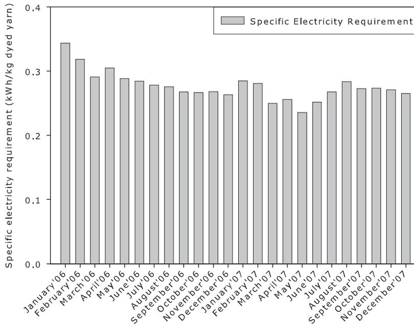
Figure 6.23: Specific electricity requirement in dyeing process
