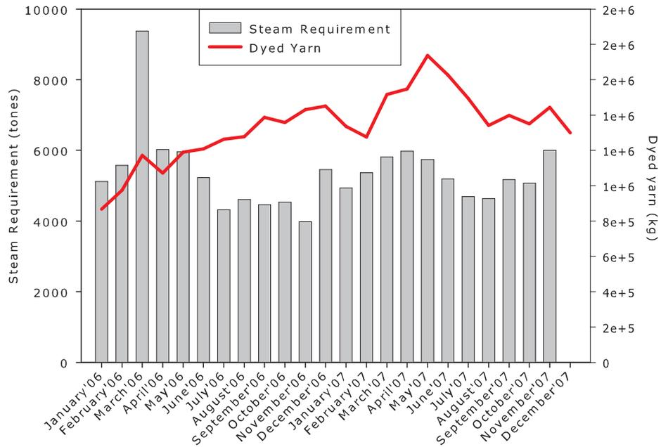
Figure 6.21: Steam requirement in dyeing process
