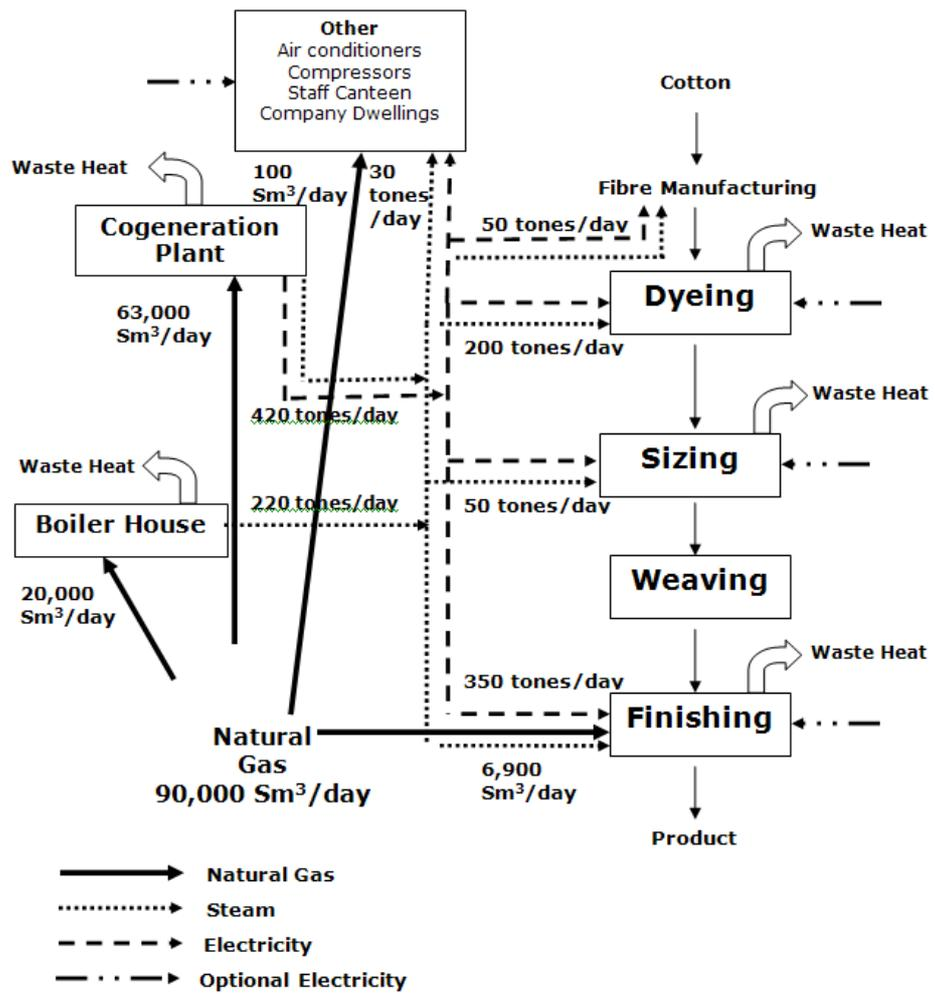
Figure 6.15: Energy flow in the mill (as of 2005)
