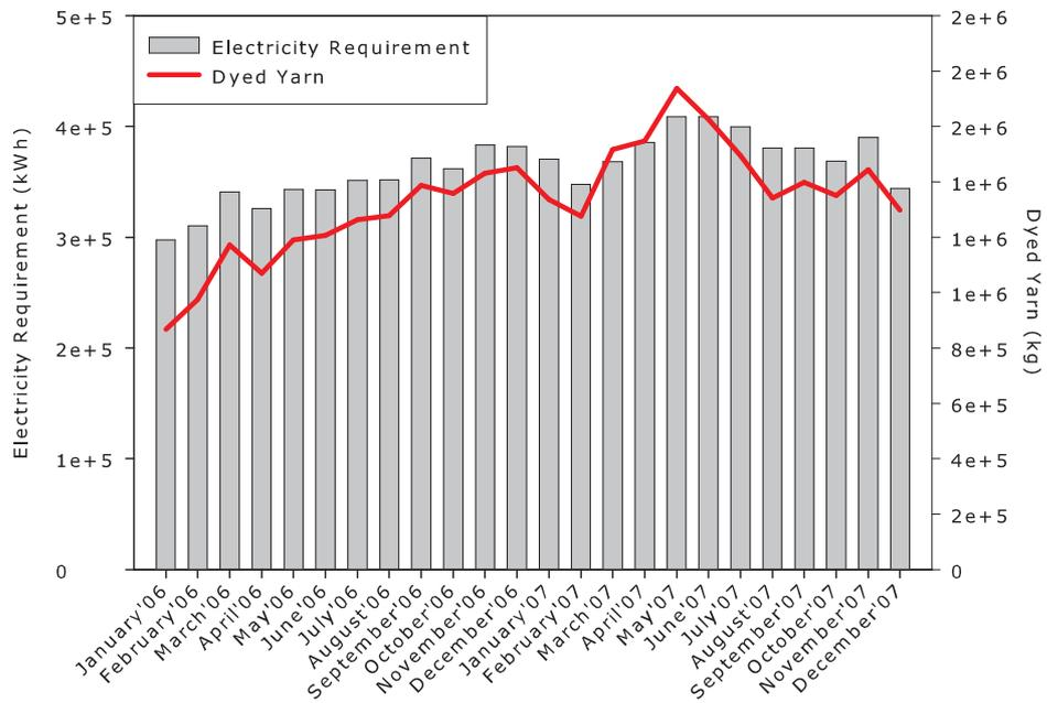
Figure 6.20: Electricity requirement in dyeing process
