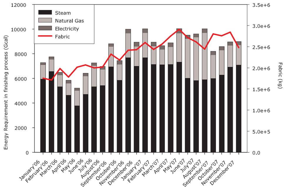
Figure 6.26: Energy source distribution in finishing process
