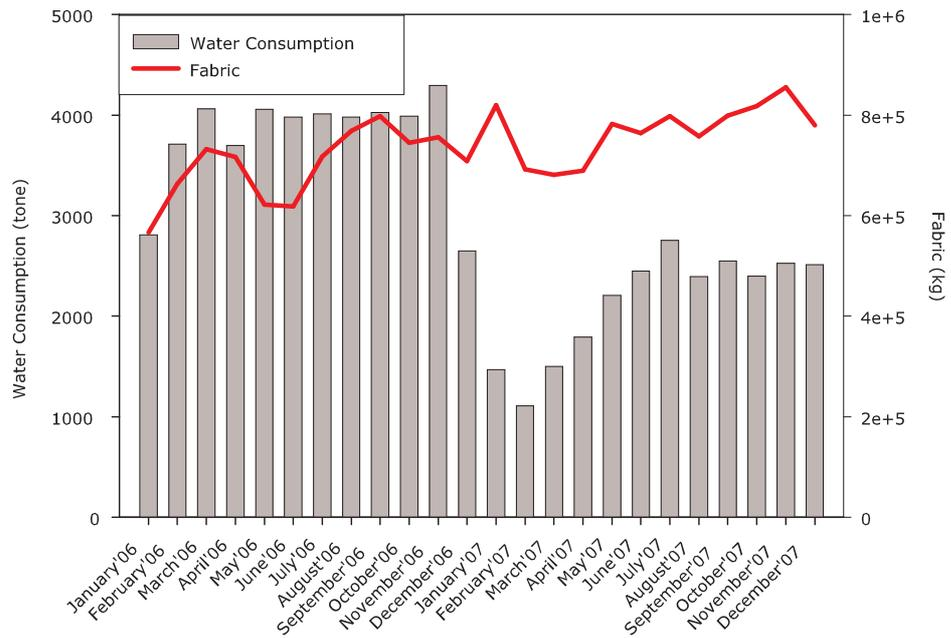
Figure A.12: Water consumption and fabric production patterns of M8
