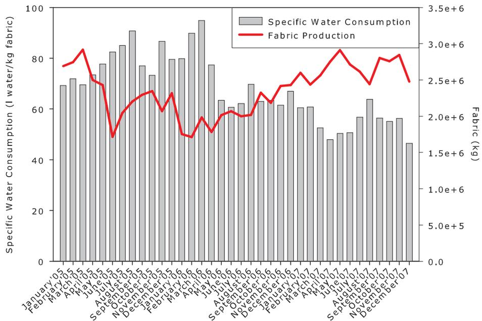
Figure 6.3: Specific water consumption and fabric production patterns in the mill
