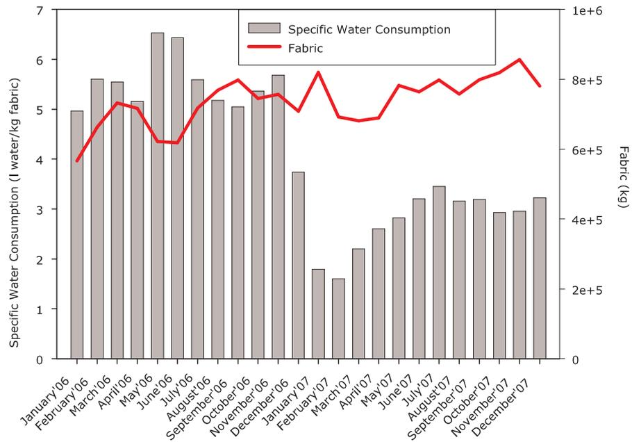
Figure A.13: Specific water consumption and fabric production patterns of M8
