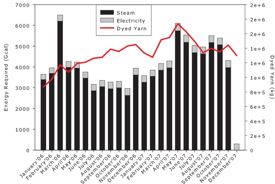
Figure 6.24: Energy source distribution in dyeing process
