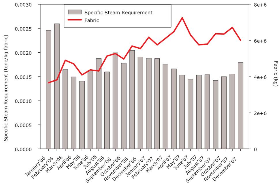
Figure 6.29: Specific steam requirement pattern in finishing process
