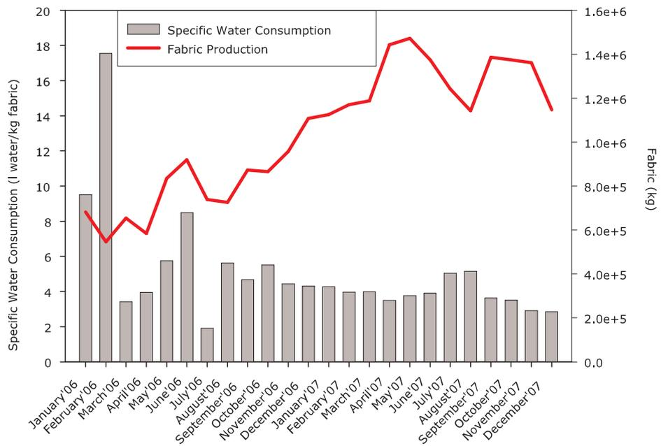
Figure 6.8: Specific water consumption and fabric production patterns in M1
