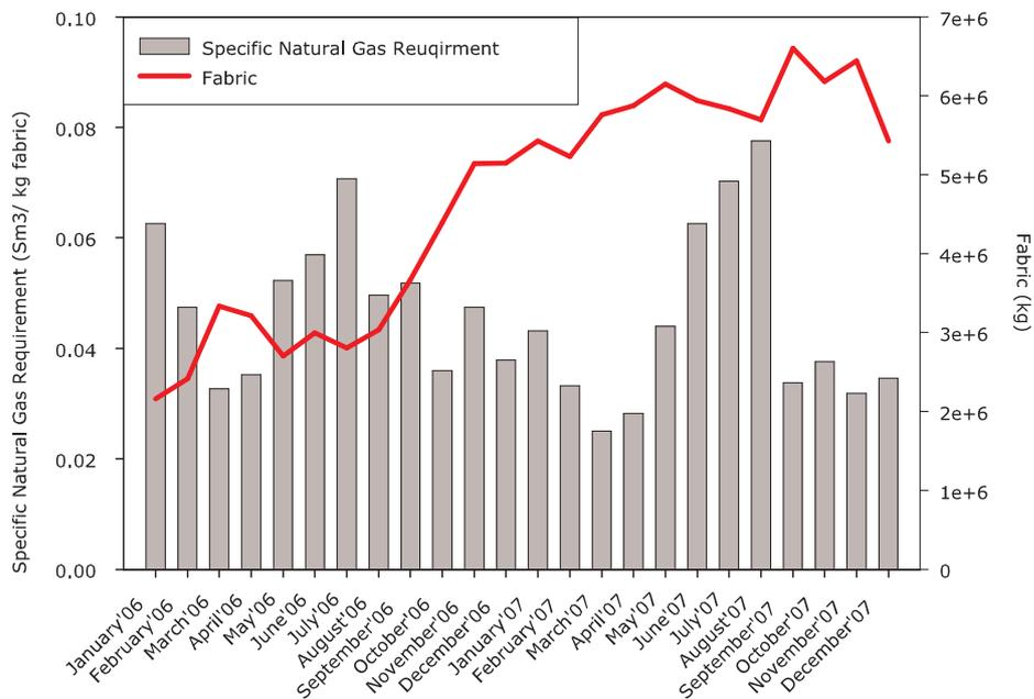
Figure 6.28: Specific natural gas requirement pattern in finishing process
