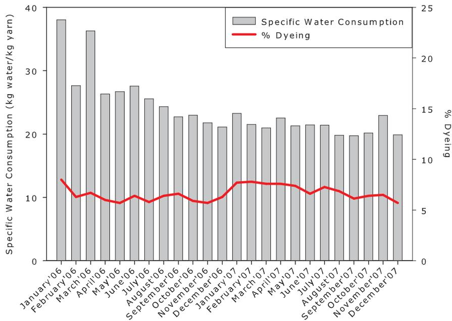
Figure 6.5: Specific water consumption and % patterns in the dyeing process
