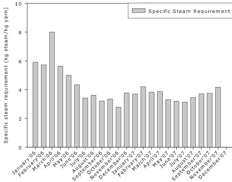
Figure 6.22: Specific steam requirement in dyeing process
