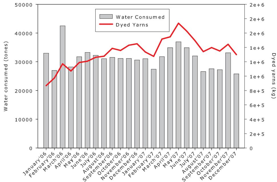
Figure 6.4: Water consumption and dyed yarns patterns in the dyeing process
