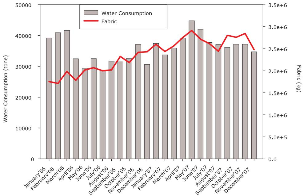
Figure 6.13: Overall water consumption and fabric production patterns in finishing process
