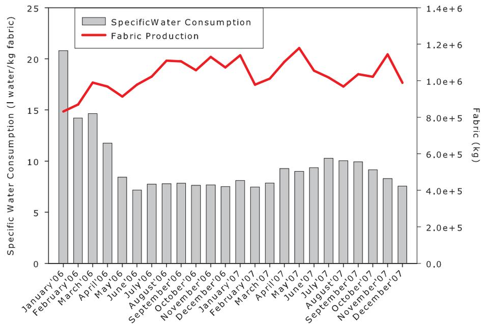
Figure 6.6: Specific water consumption and fabric production patterns in M6
