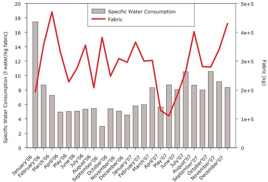
Figure A.5: Specific water consumption and fabric production patterns of M2
