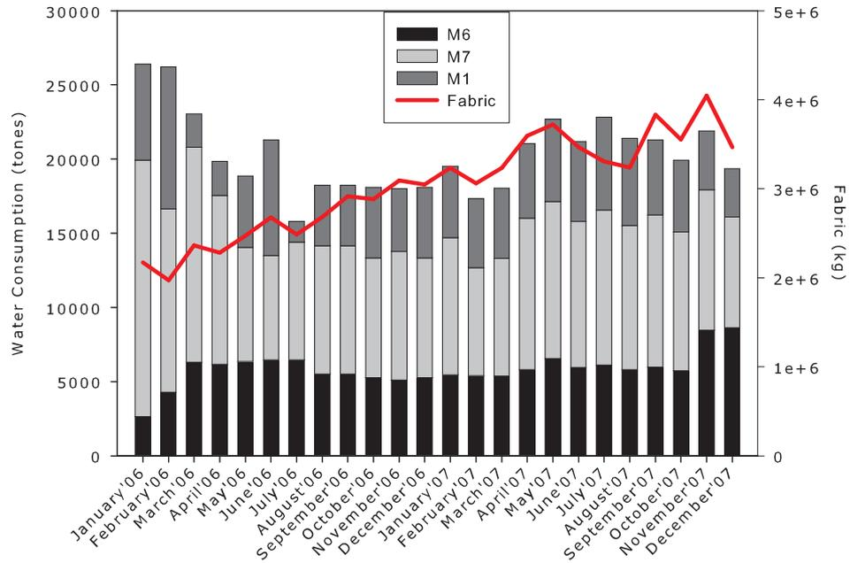
Figure 6.11: Combined water consumption and fabric production patterns of M1, M6 and M7
