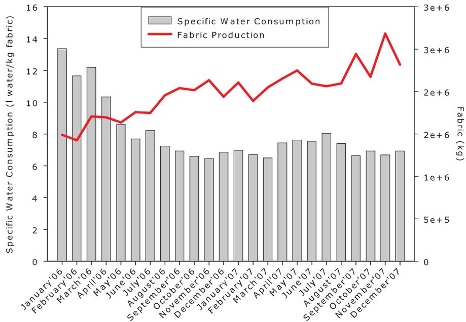
Figure 6.10: Specific water consumption pattern in M6 and M7
