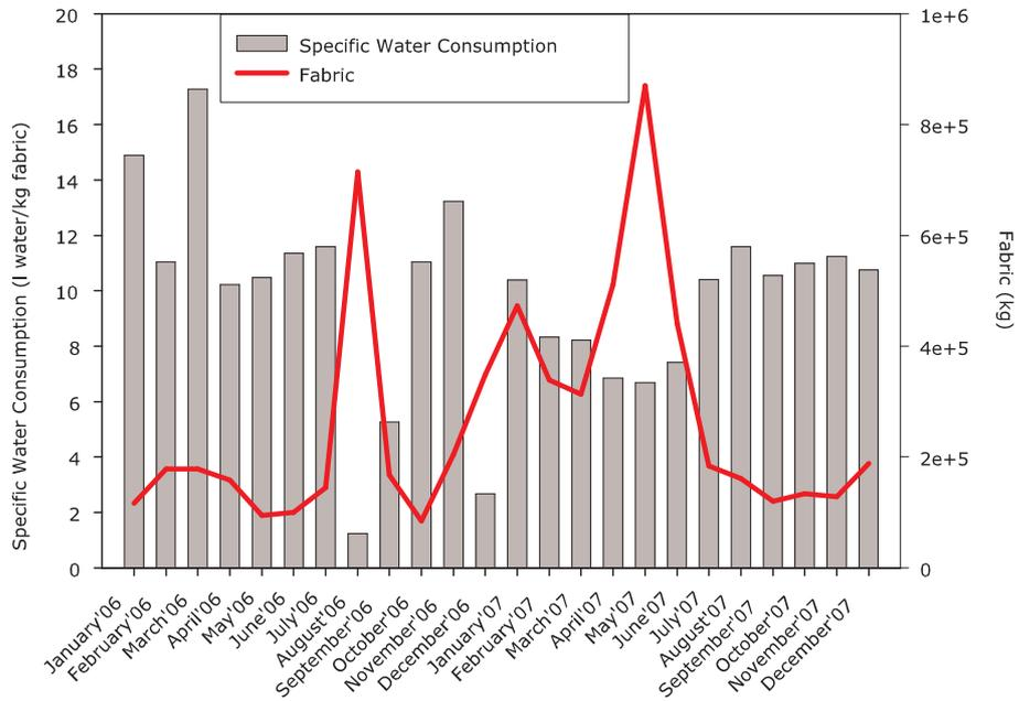
Figure A.7: Specific water consumption and fabric production patterns of M3
