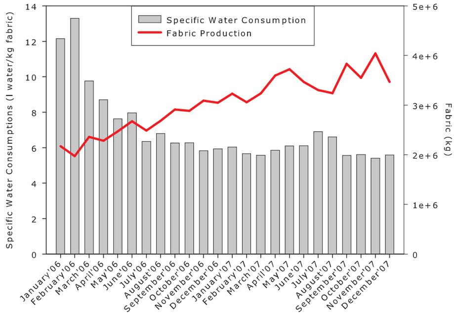
Figure 6.12: Specific water consumption and fabric production patterns of M1, M6 and M7
