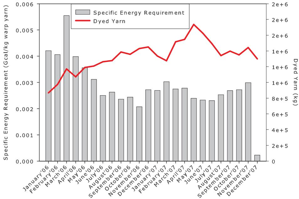
Figure 6.25: Specific energy requirement in dyeing process
