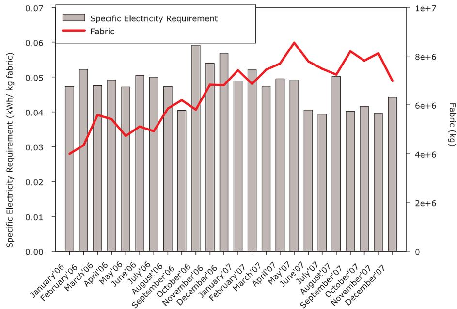
Figure 6.30: Specific electricity requirement pattern in finishing process
