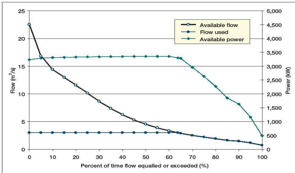
Figure 4.4. Example of a Power - Duration Curve (RETScreen, 2004-a)
