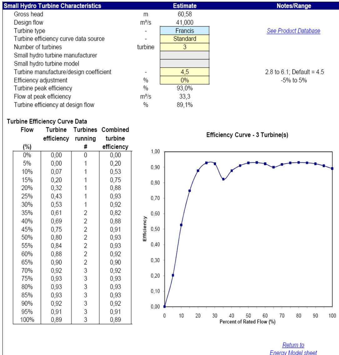
Figure 5.19. Kadincik-4 HEPP Alternative II, Equipment Data
