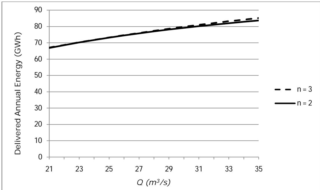
Figure 5.28. The Effect of the Number of Turbines on Delivered Energy
