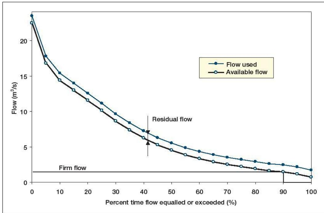
Figure 4.2. Example of a Flow-Duration Curve (RETScreen 2004-a)
