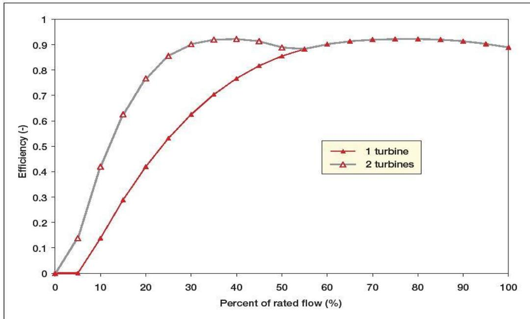
Figure 4.3. Example of a Turbine Efficiency Curve (RETScreen, 2004-a)
