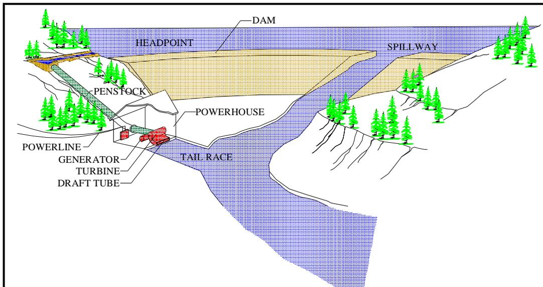
Figure 2.5. Components of a Hydropower Project (Overview)
