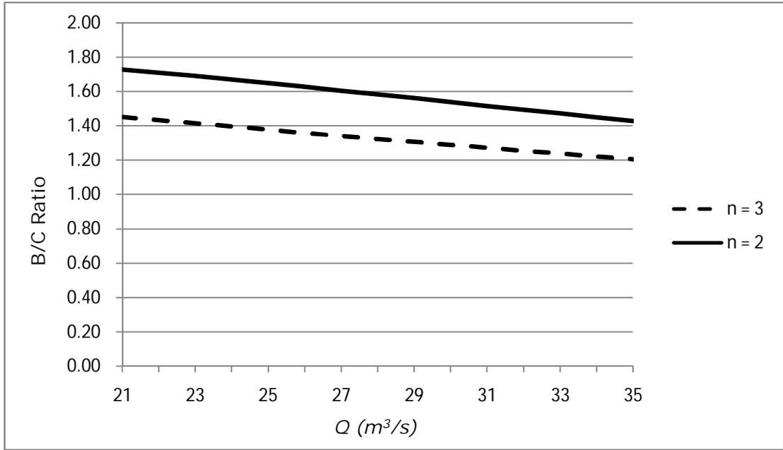
Figure 5.27. The Effect of the Number of Turbines on B-C Ratio
