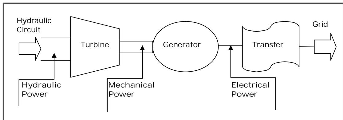
Figure 2.3. Electrical Power Conversion Scheme
