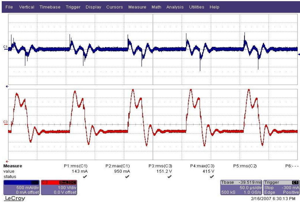
Figure 5.9 DPWM1 zoom in CMC (blue) and CMV (red) waveforms for M_i=0.8 .
