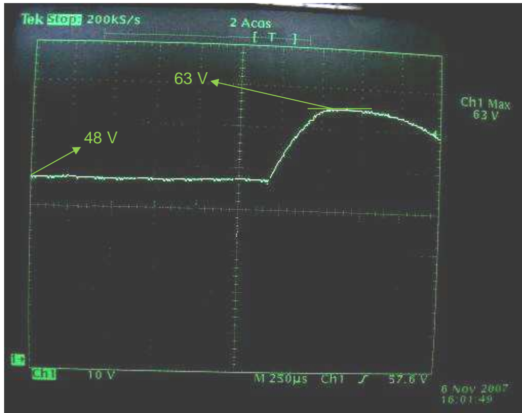
Figure 5-42: EPQM supply input under surge test
