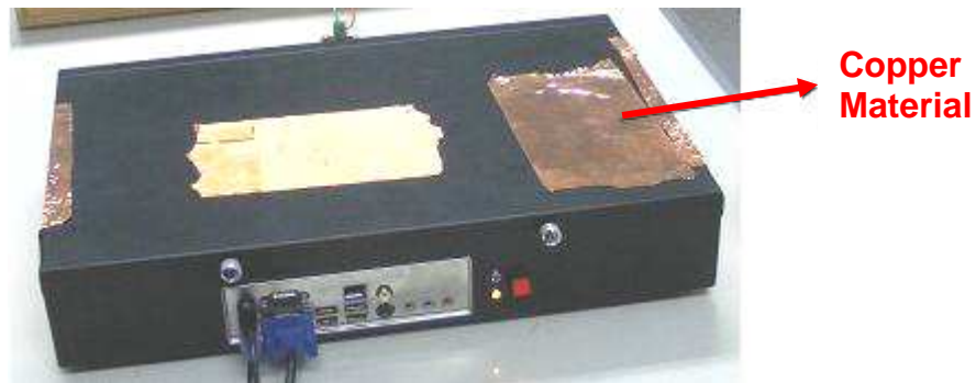
Figure 5-7: ESD countermeasures on EPQM
