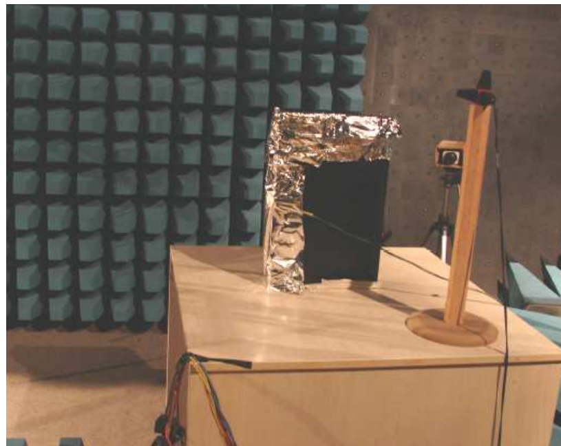
Figure 5-24: Aluminium foil bonded to the EPQM
