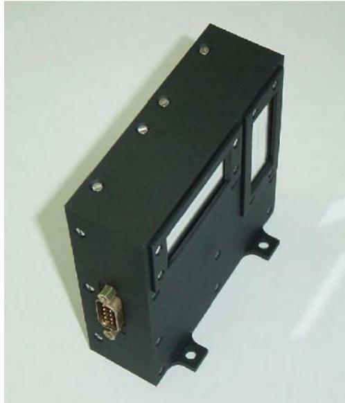
Figure 2.13 Satrec Initiative FSS\_05 Analog Sun Sensor
