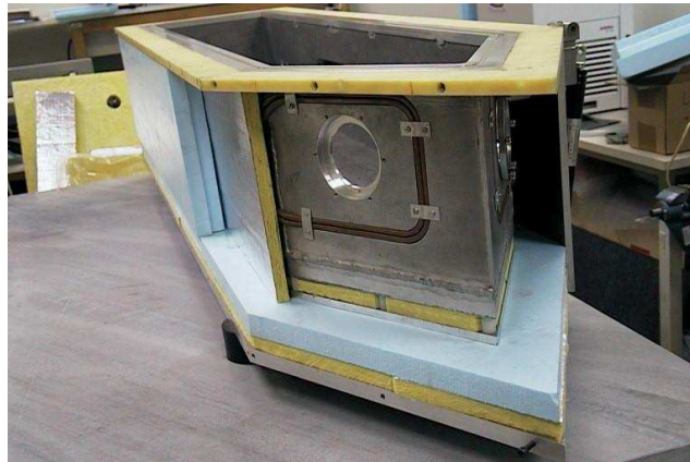
Figure 2. The mechanical design and cross-section of Köster Interferometer
