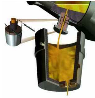
Figure C.3 EMLI™ Slag Indication Oxygen Vessel (EMLI-SIO) - for real-time slag detection on B.O.F. furnaces [110]
