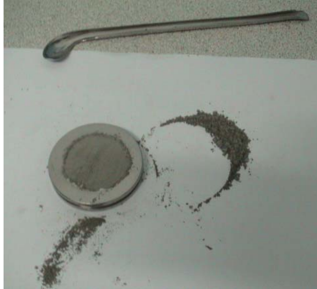
Figure 3.2 Powder of slag particles placed in hollow cylindrical shape steel, with a base covered by cellulose
