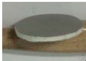
Figure 3.3 Pressed sample; Thin layer of slag sample (gray) over cellulose material (white)
