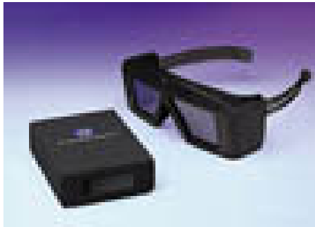
Figure 6.1 CrystalEyes3, stere3D eyewear and its emitter from StereoGraphics.
