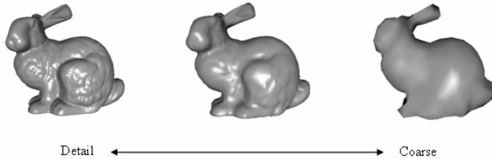
**Figure 3.16** Representations of a 3D model in different wavelet sublevels.
