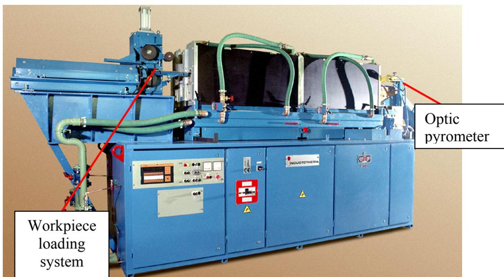
Figure 1.4 Sub-units of the Induction Heating Furnace
