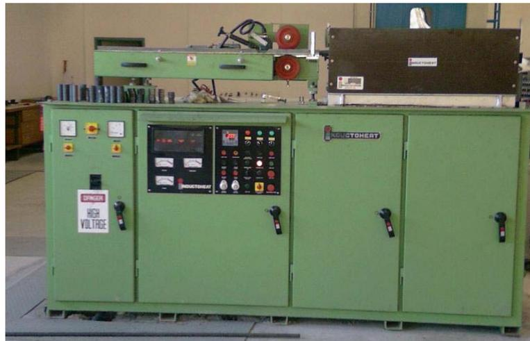
Figure 4.1 125 KW 3000 Hz Induction Heater
