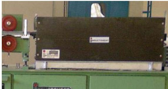
Figure 4.7 Induction coil box mounted on induction heater 125 KW 3000Hz
