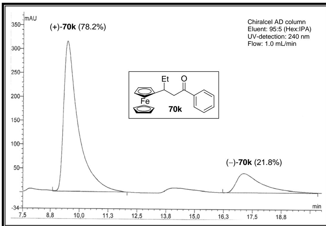
**Figure A80.** HPLC chromatogram of compound **70k** (56% ee)
