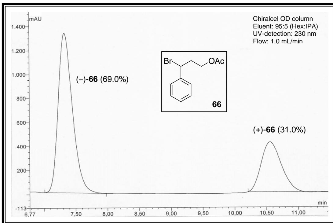
**Figure A46.** HPLC chromatogram of ester **66** (38% ee)
