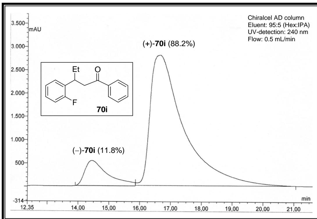
**Figure A78.** HPLC chromatogram of compound **70i** (76% ee)
