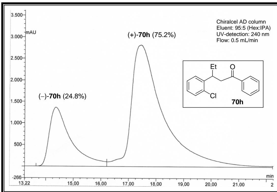
**Figure A77.** HPLC chromatogram of compound **70h** (50% ee)
