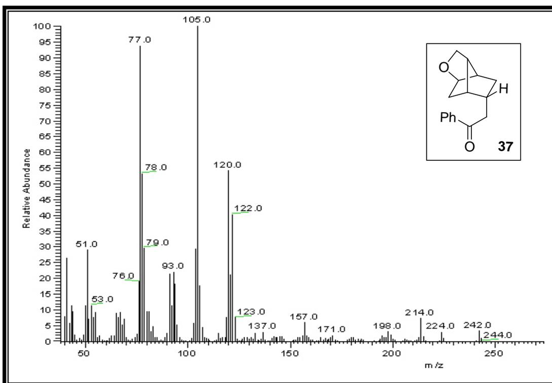
**Figure A10.** Mass spectrum of tricyclic ether **37**
