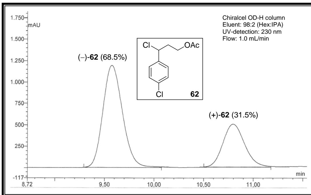
**Figure A38.** HPLC chromatogram of ester **62** (37% ee)
