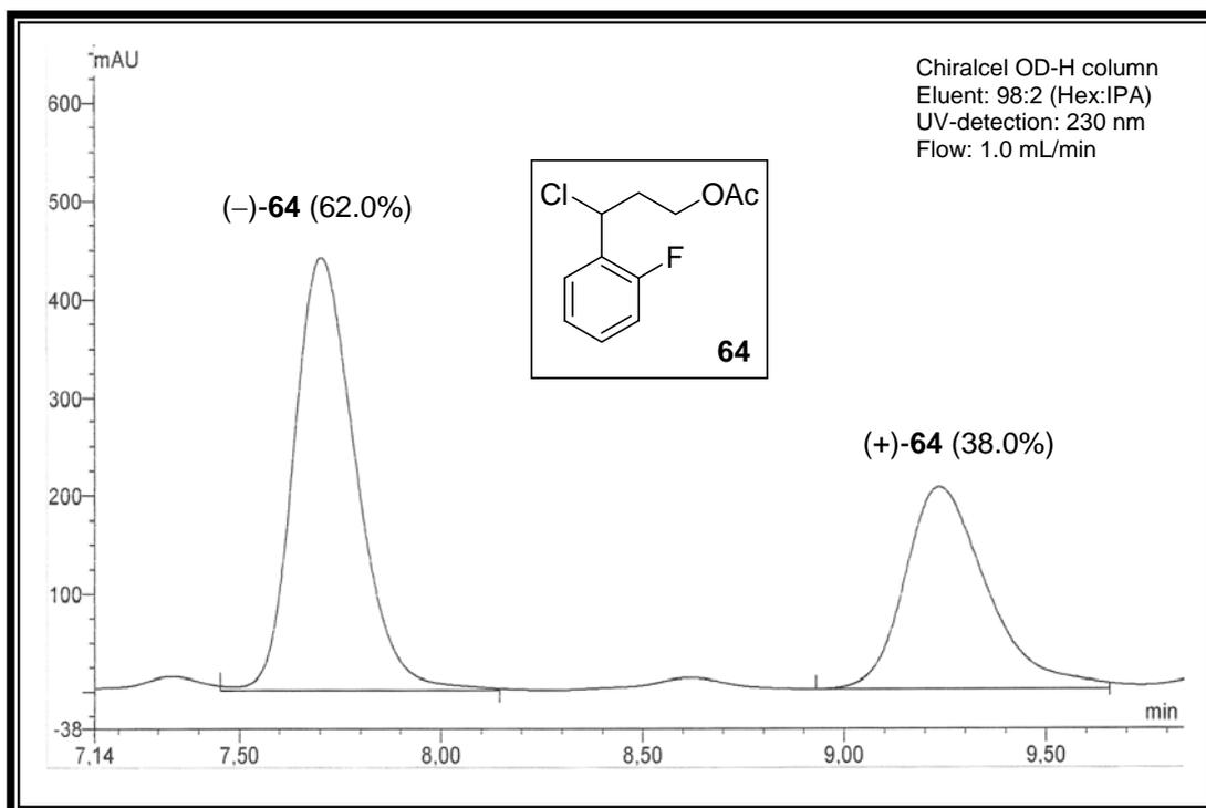
**Figure A42.** HPLC chromatogram of ester **64** (24% ee)
