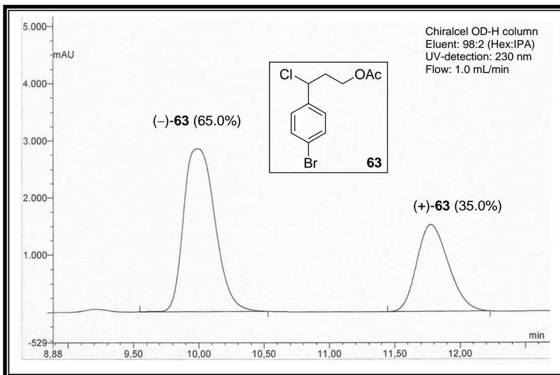
**Figure A40.** HPLC chromatogram of ester **63** (30% ee)
