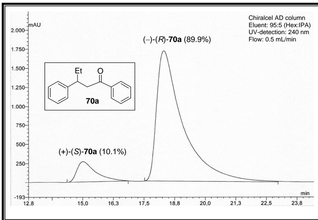
**Figure A70.** HPLC chromatogram of compound **70a** (80% ee)
