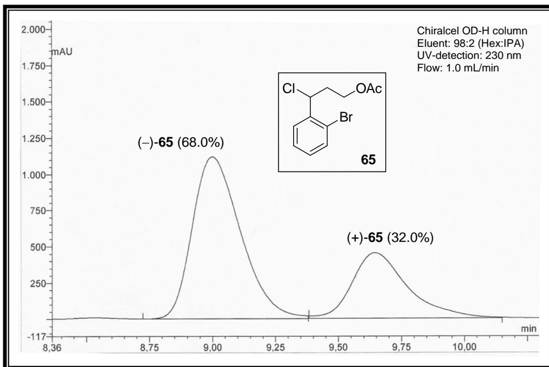
**Figure A44.** HPLC chromatogram of ester **65** (36% ee)
