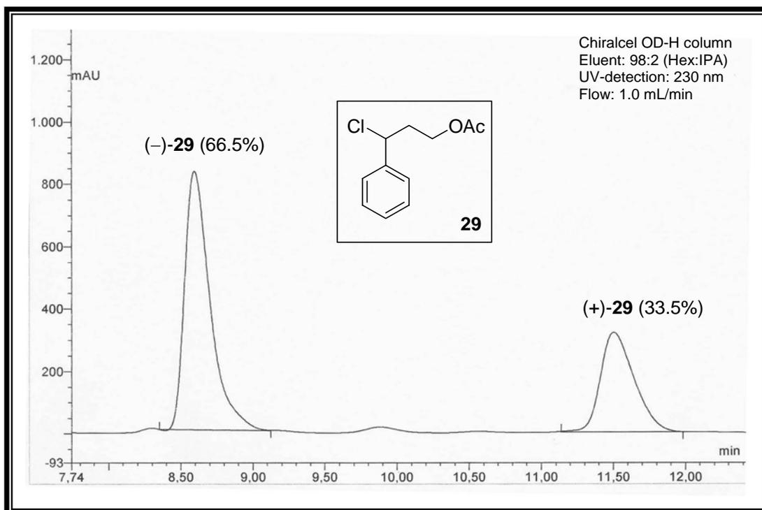
**Figure A34.** HPLC chromatogram of ester **29** (33% ee)
