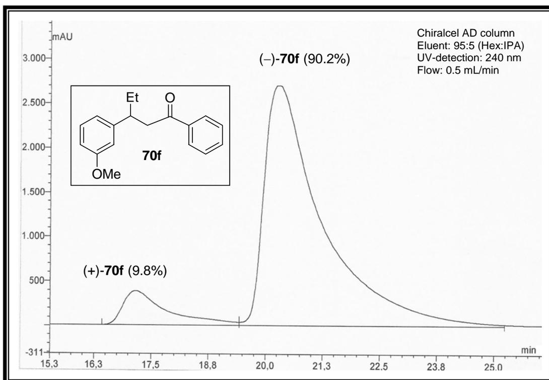
**Figure A75.** HPLC chromatogram of compound **70f** (80% ee)
