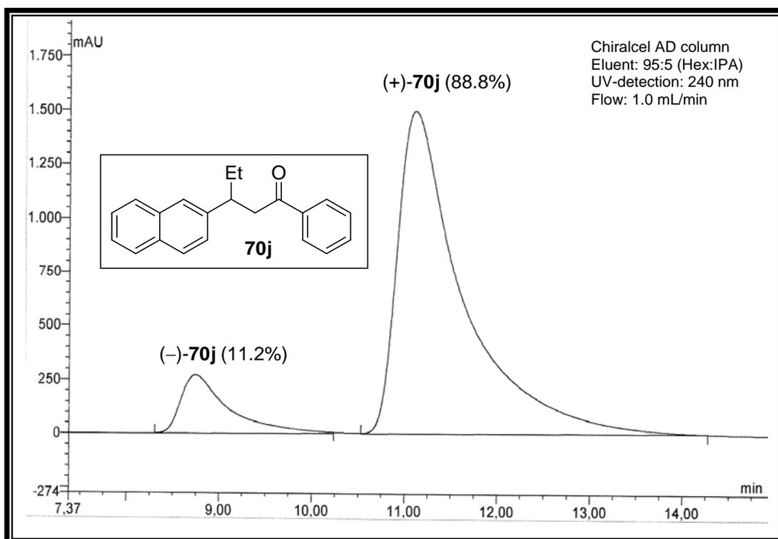
**Figure A79.** HPLC chromatogram of compound **70j** (78% ee)
