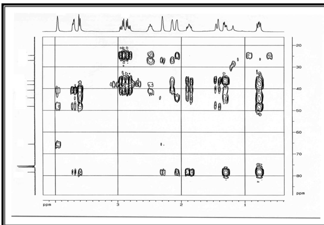
**Figure A8.** Part of HMBC spectrum of tricyclic ether **37**
