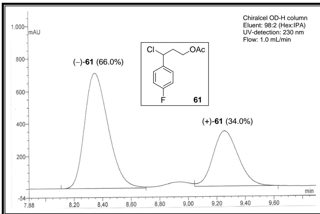
**Figure A36.** HPLC chromatogram of ester **61** (32% ee)
