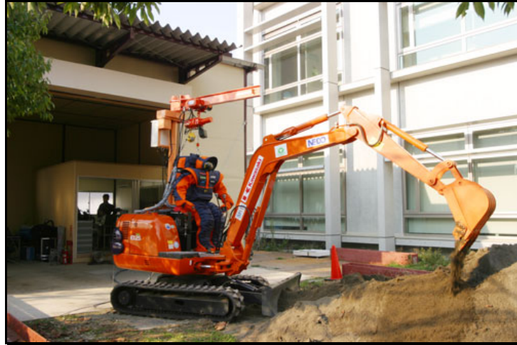
Figure 1.8 HRP-1S is remotely controlled to drive an industrial vehicle. It has been developed to operate the vehicle with tele-operation [22].
