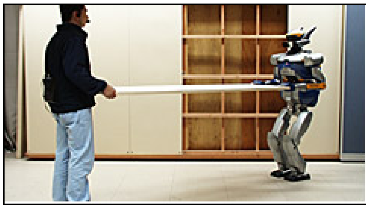
Figure 1.7 HRP-2, a humanoid, helps assembling a panel [21].
