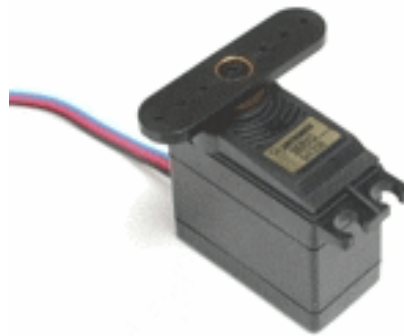
Figure C.1 RC Servo Motor Model Used to Actuate the Fourth Axis of the Robot.
