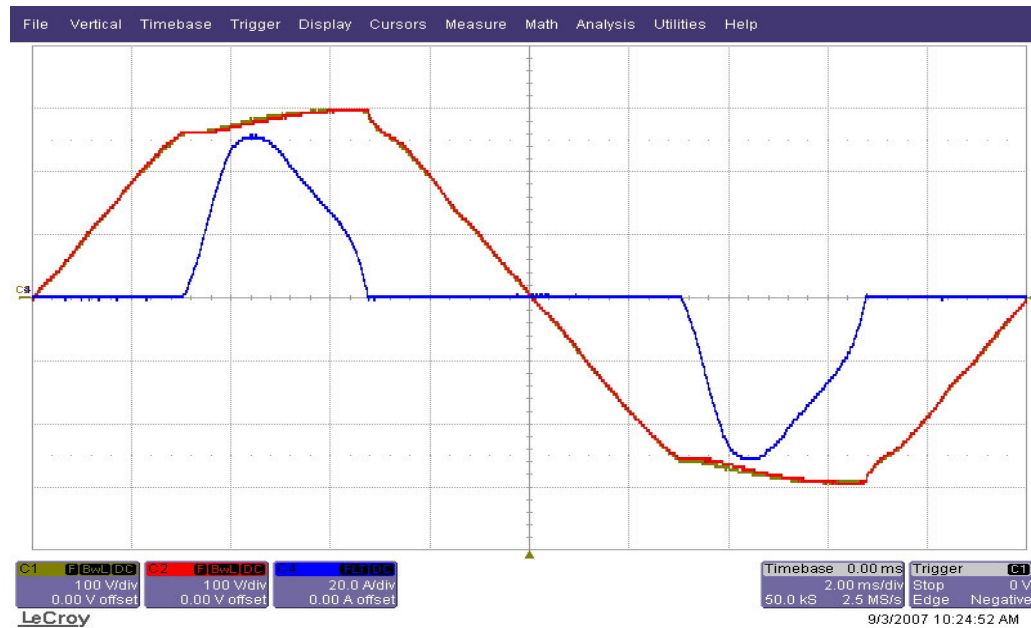
Figure 5.5 Uncompensated single-phase system line voltage (yellow), load voltage (red), and line current (blue) waveforms in by-pass mode.
