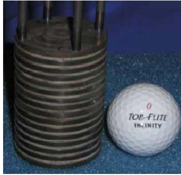
Figure 1.13 ITN 15-Cell Palm Power SOFC Stack [92]
