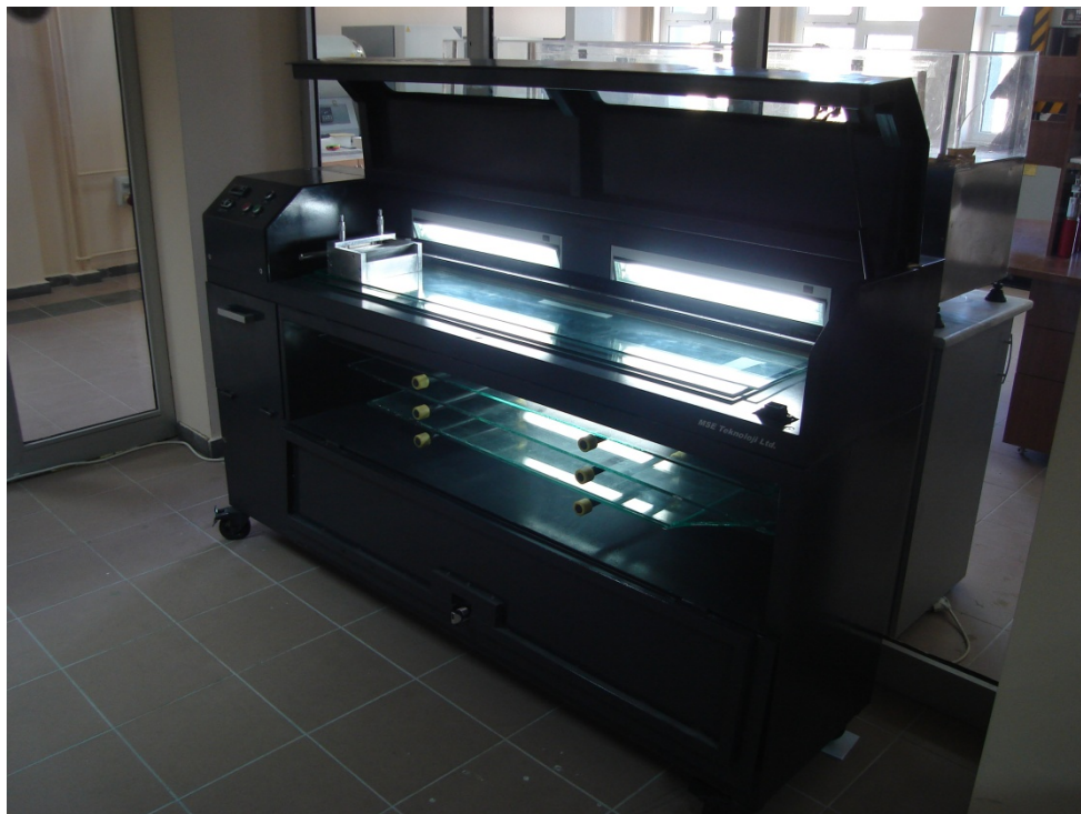
Figure 5.9 Laboratory scale tape casting equipment
