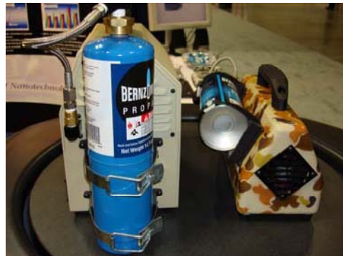
Figure 1.12 Nano Dynamic's portable solid oxide fuel cell unit [90]
