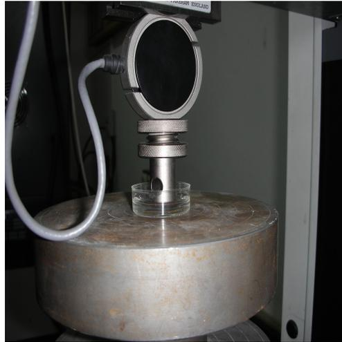
**Figure 2.3.** Set up used in stress-relation tests of agarose-chondrocyte discs.
