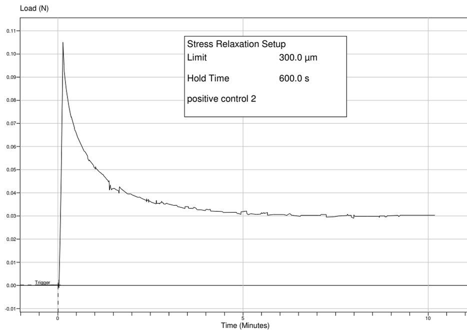
**Figure 3.14.** Typical unconfined compression stress-relaxation curve during 10 % strain stress-relaxation tests for healthy group of agarose-chondrocyte discs after 27 days of *in vitro* incubation.
