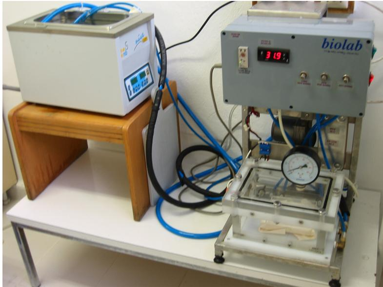
**Figure 2.2.** Custom-made pressure chamber
