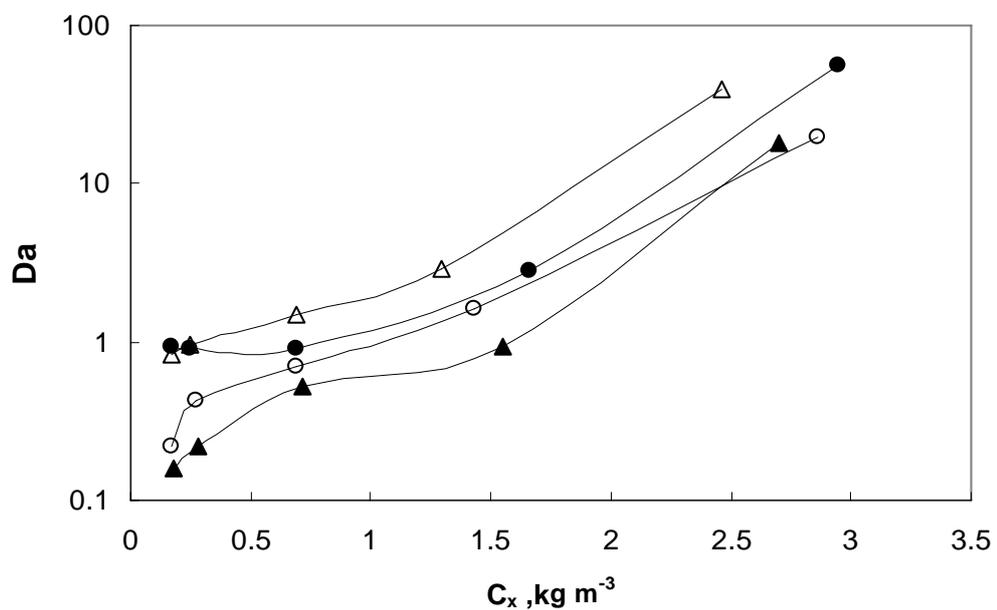
**Figure 4.9** The variation of Da ( $\text{OD}/\text{OTR}_{\text{max}}$ ) with cell concentration, agitation and air inlet rates: OT<sub>3</sub> (○); OT<sub>4</sub> (▲) OT<sub>5</sub> (△); OT<sub>6</sub> (●).  $C_G^0 = 8.0 \text{ kg m}^{-3}$ ,  $T=37^\circ\text{C}$ ,  $V_R=1.65 \times 10^{-3} \text{ m}^3$ ,  $\text{pH}_c=7.2$ .
