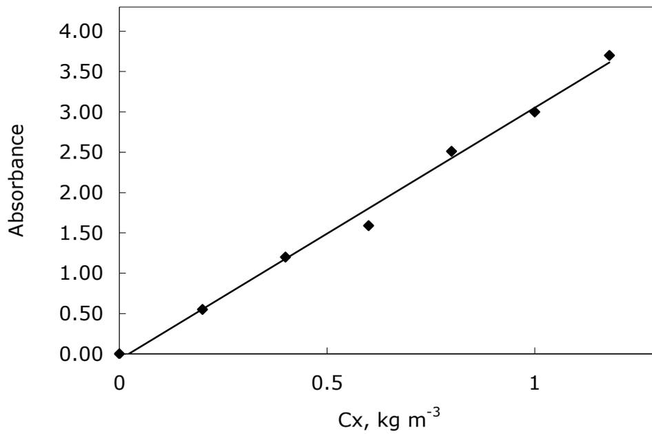
**Figure A.1** Calibration curve for *Escherichia coli* concentration
