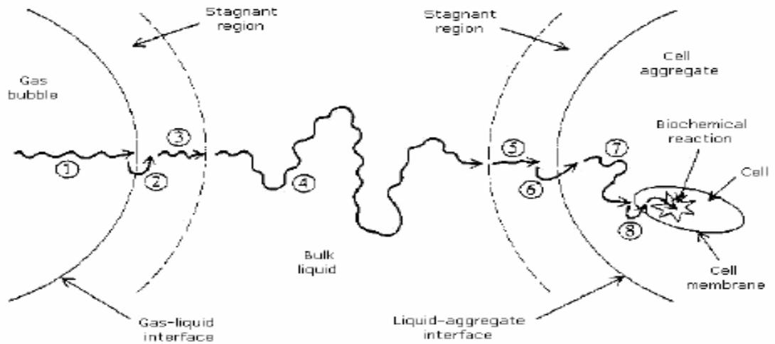
**Figure 2.4** Schematic diagram of steps involved in transport of oxygen from a gas bubble to inside a cell (Bailey and Ollis, 1986)
