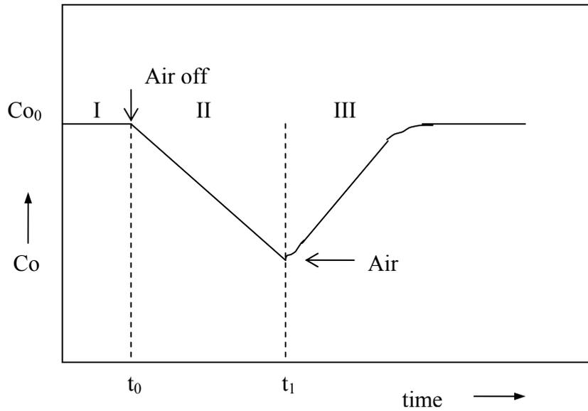
**Figure 2.5** Variation of dissolved oxygen concentration with time in dynamic measurement of  $K_L a$ .
