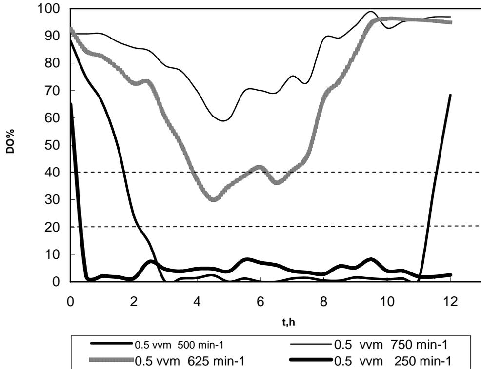
**Figure 4.1** The variations in the dissolved oxygen concentration with the cultivation time, agitation and air inlet rates applied.  $C_G=8.0 \text{ Kg m}^{-3}$ ,  $T=37^\circ\text{C}$ ,  $V_R=1.65 \times 10^{-3} \text{ m}^3$ ,  $\text{pH}_c=7.2$ .
