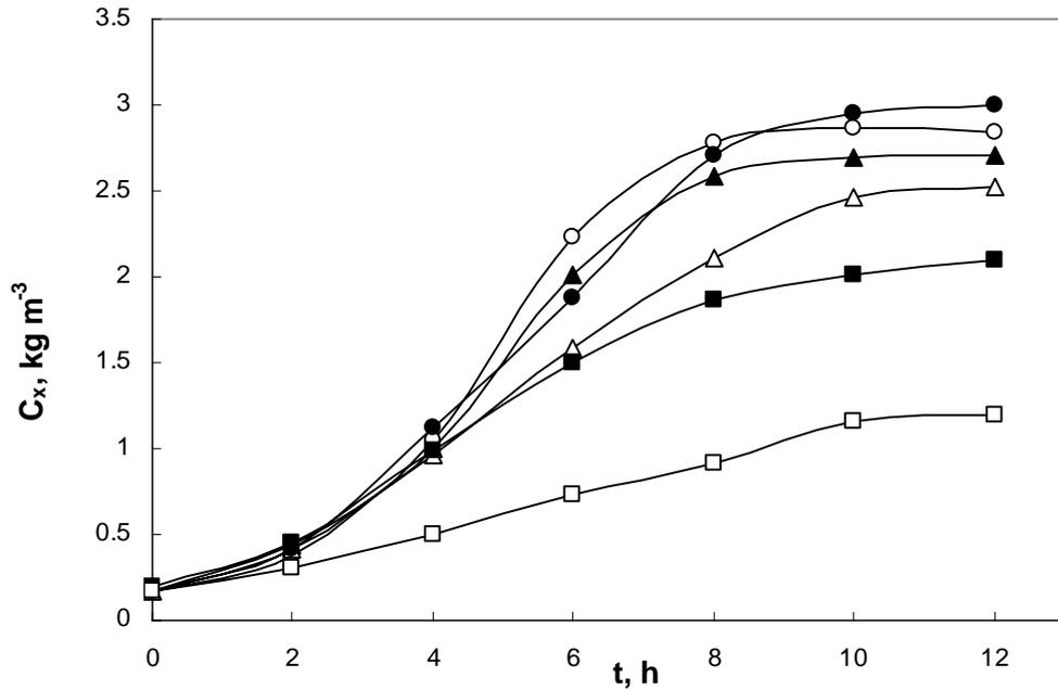
**Figure 4.3** The variations in cell concentration with the cultivation time, agitation rates and air inlet rates applied and medium contents: OT<sub>1</sub> (□); OT<sub>2</sub> (■); OT<sub>3</sub> (○); OT<sub>4</sub> (▲); OT<sub>5</sub> (△); OT<sub>6</sub> (●).  $C_G=8.0 \text{ Kg m}^{-3}$ ,  $T=37^\circ\text{C}$ ,  $V_R=1.65 \times 10^{-3} \text{ m}^3$ ,  $\text{pH}_c=7.2$ .
