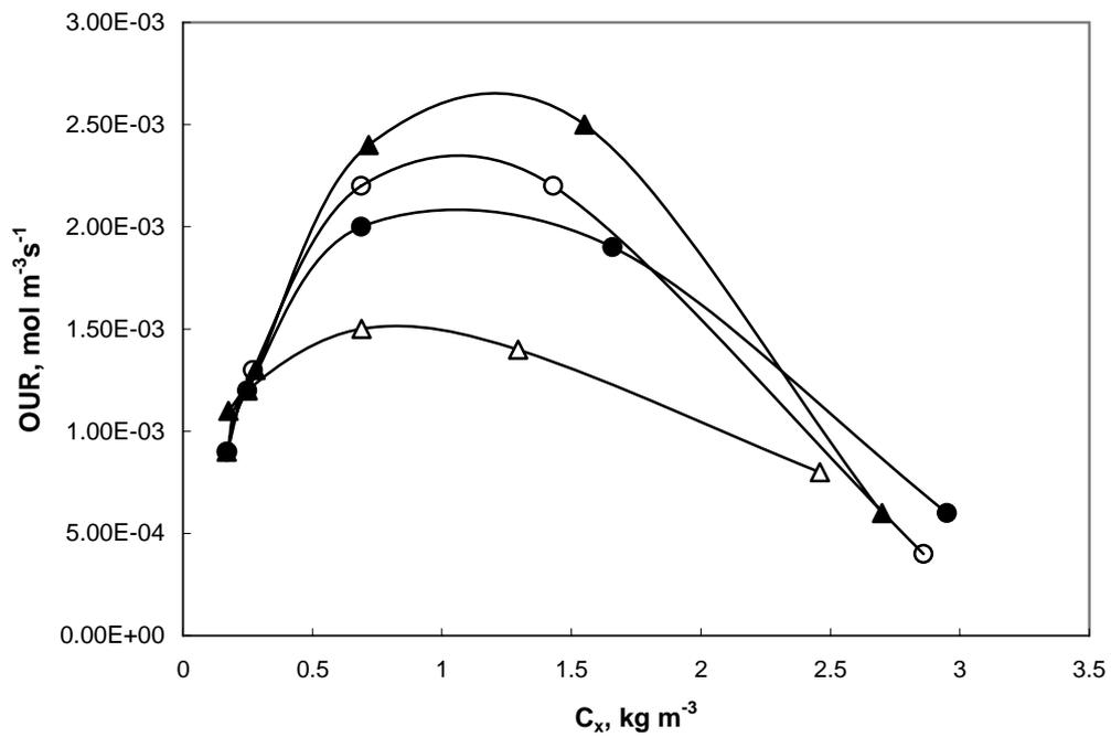
**Figure 4.8** The variation of OUR with cell concentration, agitation and air inlet rates: OT<sub>3</sub> (○); OT<sub>4</sub> (▲) OT<sub>5</sub> (△); OT<sub>6</sub> (●).  $C_G^0 = 8.0 \text{ kg m}^{-3}$ ,  $T=37^\circ\text{C}$ ,  $V_R=1.65 \times 10^{-3} \text{ m}^3$ ,  $\text{pH}_c=7.2$ .
