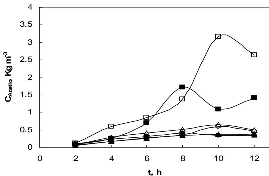
**Figure 4.6** The variations in acetic acid concentration with the cultivation time, agitation and air inlet rates: OT<sub>1</sub> (□); OT<sub>2</sub> (■); OT<sub>3</sub> (○); OT<sub>4</sub> (▲) OT<sub>5</sub> (△); OT<sub>6</sub> (●).  $C_G^0 = 8.0 \text{ kg m}^{-3}$ ,  $T = 37^\circ\text{C}$ ,  $V_R = 1.65 \times 10^{-3} \text{ m}^3$ ,  $\text{pH}_c = 7.2$ .
