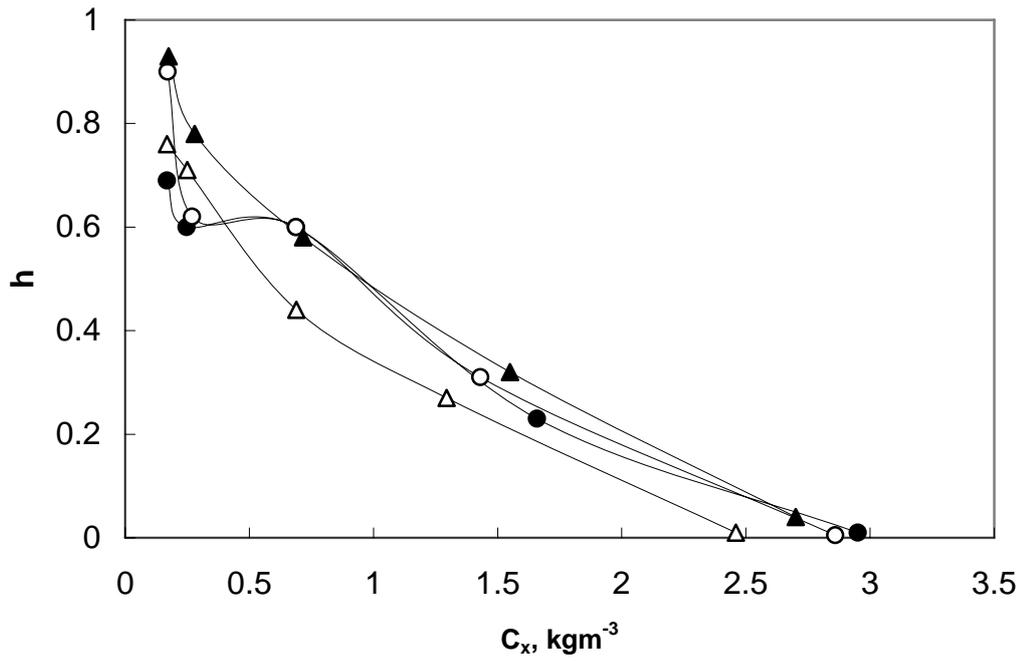
**Figure 4.10** The variation of  $\eta$  (OUR/OD) with cell concentration , agitation and air inlet rates:OT<sub>3</sub> (○); OT<sub>4</sub> (▲) OT<sub>5</sub> (Δ); OT<sub>6</sub> (●).  $C_G^0 = 8.0 \text{ kg m}^{-3}$ ,  $T=37^\circ\text{C}$ ,  $V_R= 1.65 \times 10^{-3} \text{ m}^3$ ,  $\text{pH}_c=7.2$ .
