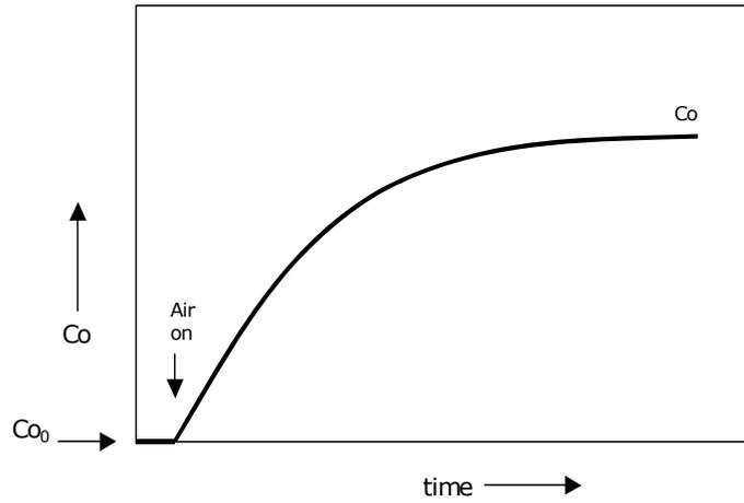
**Figure 2.7** Variation of dissolved oxygen concentration with time in dynamic measurement of  $K_{La0}$  using the Dynamic Method
