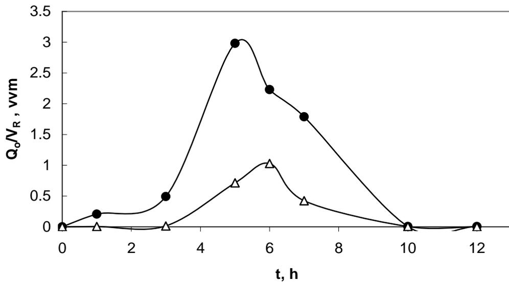
**Figure 4.2** The variations in air flow rate with the cultivation time: OT<sub>5</sub> ( $\Delta$ ); OT<sub>6</sub> ( $\bullet$ ).  $C_G=8.0 \text{ Kg m}^{-3}$ ,  $T=37^\circ\text{C}$ ,  $V_R=1.65 \times 10^{-3} \text{ m}^3$ ,  $\text{pH}_c=7.2$ .
