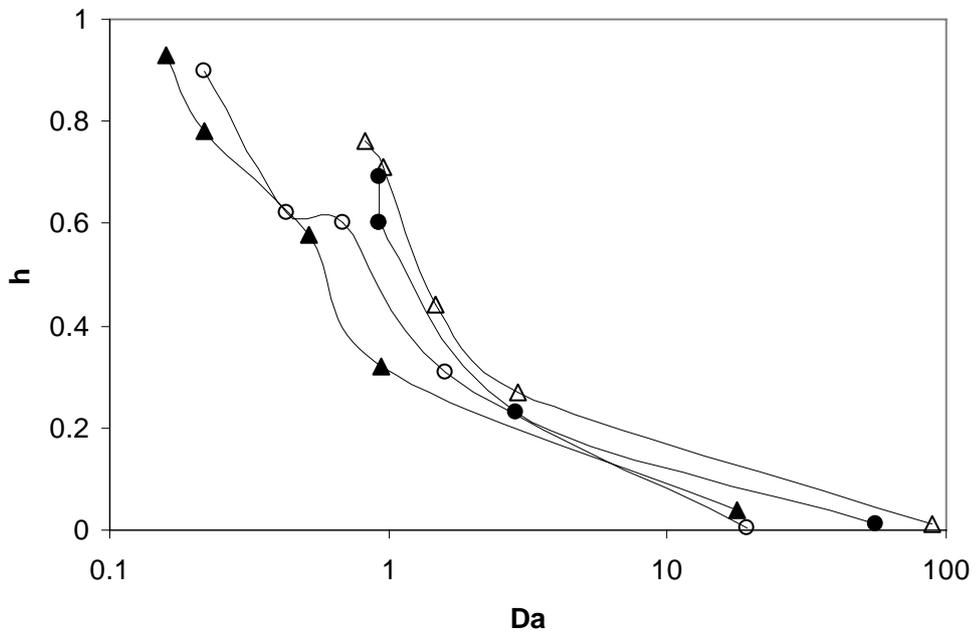
**Figure 4.11** The relationship between  $Da$  and  $\eta$  at different oxygen transfer conditions: OT<sub>3</sub> (○); OT<sub>4</sub> (▲) OT<sub>5</sub> (Δ); OT<sub>6</sub> (●).  $C_G^0 = 8.0 \text{ kg m}^{-3}$ ,  $T=37^\circ\text{C}$ ,  $V_R= 1.65 \times 10^{-3} \text{ m}^3$ ,  $\text{pH}_c=7.2$ .
