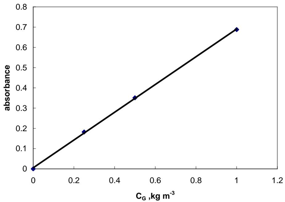
**Figure B.1** Calibration curve of the glucose analysis solution
