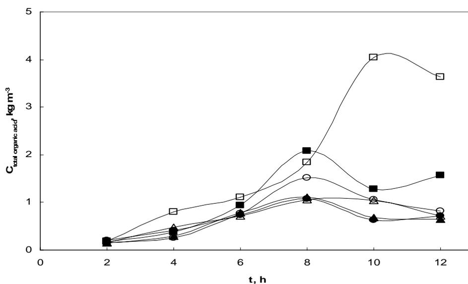
**Figure 4.7** The variations in total organic acid concentration with the cultivation time, agitation and air inlet rates: OT<sub>1</sub> (□); OT<sub>2</sub> (■); OT<sub>3</sub> (○); OT<sub>4</sub> (▲) OT<sub>5</sub> (△); OT<sub>6</sub> (●).  $C_G^0 = 8.0 \text{ kg m}^{-3}$ ,  $T = 37^\circ\text{C}$ ,  $V_R = 1.65 \times 10^{-3} \text{ m}^3$ ,  $\text{pH}_c = 7.2$ .
