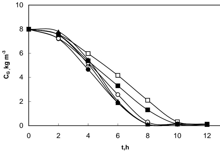
**Figure 4.4** The variations in glucose concentration with the cultivation time, agitation rates and air inlet rates applied and medium contents: OT<sub>1</sub> (□); OT<sub>2</sub> (■); OT<sub>3</sub> (○); OT<sub>4</sub> (▲) OT<sub>5</sub> (Δ); OT<sub>6</sub> (●).  $C_G=8.0 \text{ Kg m}^{-3}$ ,  $T=37^\circ\text{C}$ ,  $V_R=1.65 \times 10^{-3} \text{ m}^3$ ,  $\text{pH}_C=7.2$ .
