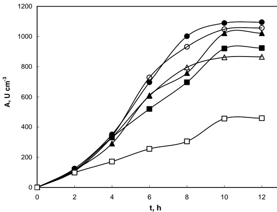
**Figure 4.5** The variations in benzaldehyde lyase volumetric activity with the cultivation time, agitation and air inlet rates applied: OT<sub>1</sub> (□); OT<sub>2</sub> (■); OT<sub>3</sub> (○); OT<sub>4</sub> (▲) OT<sub>5</sub> (△); OT<sub>6</sub> (●).  $C_G=8.0 \text{ Kg m}^{-3}$ ,  $T=37^\circ\text{C}$ ,  $V_R=1.65 \times 10^{-3} \text{ m}^3$ ,  $\text{pH}_c=7.2$ .
