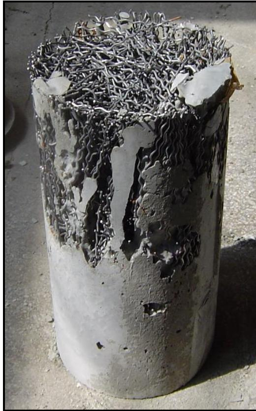
**Figure 2.5: An example of failed preparation because of the lack of fluidity of slurry**
