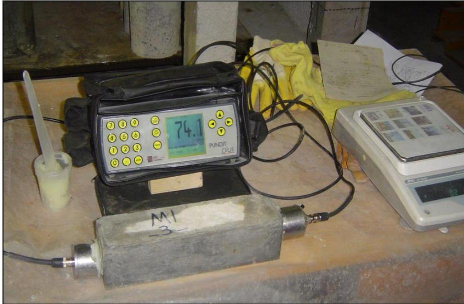
**Figure 3.16: UPV testing of freeze-thaw specimens**
