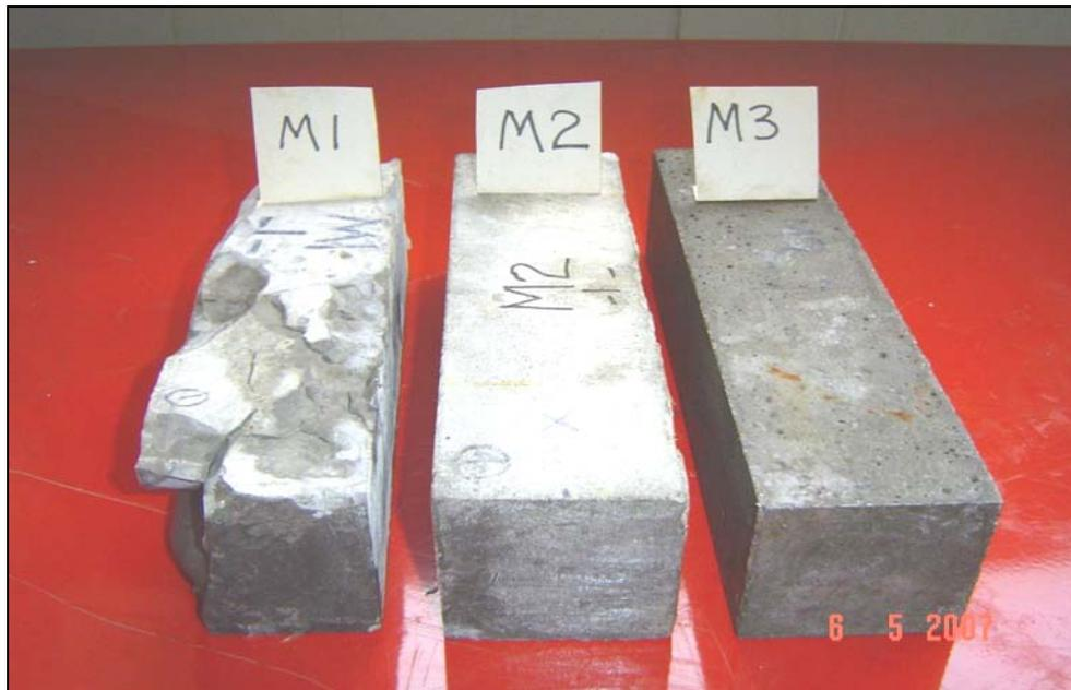
**Figure 4.38: Plain specimens after 300 cycles of freezing and thawing**
