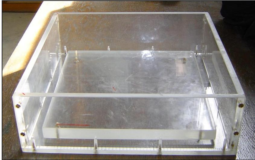
**Figure 3.8: A mold for chloride penetration test specimens**
