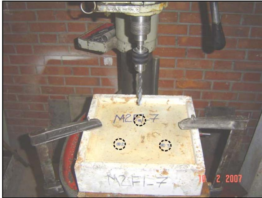
**Figure 3.10: Setup of extracting dust samples of chloride penetration test**
