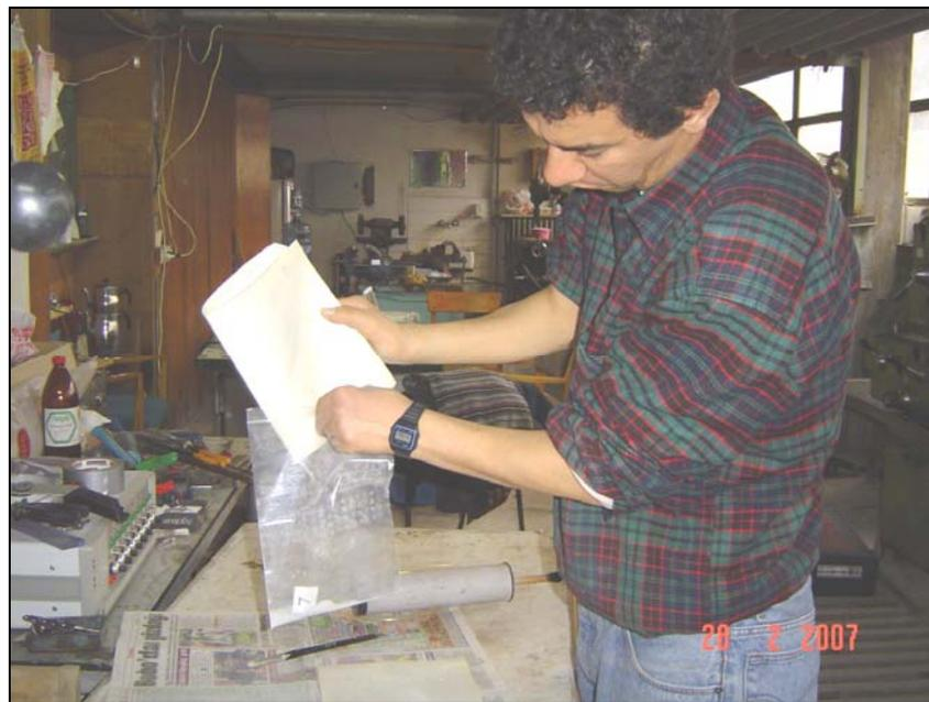
**Figure 3.11: Collecting dust samples in sealed bags for chloride chemical analysis**
