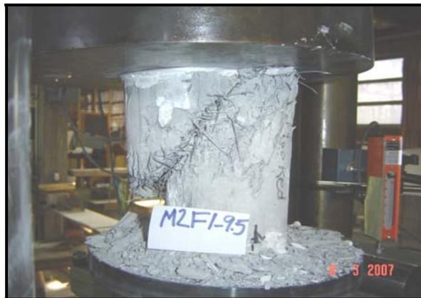
**(c) The specimen shows high deformations but still resist the loading**
