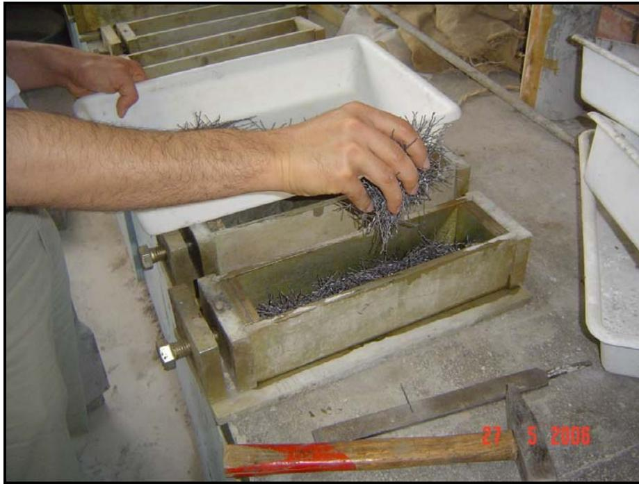
**Figure 2.1: Placement of steel fibers in a mold**
