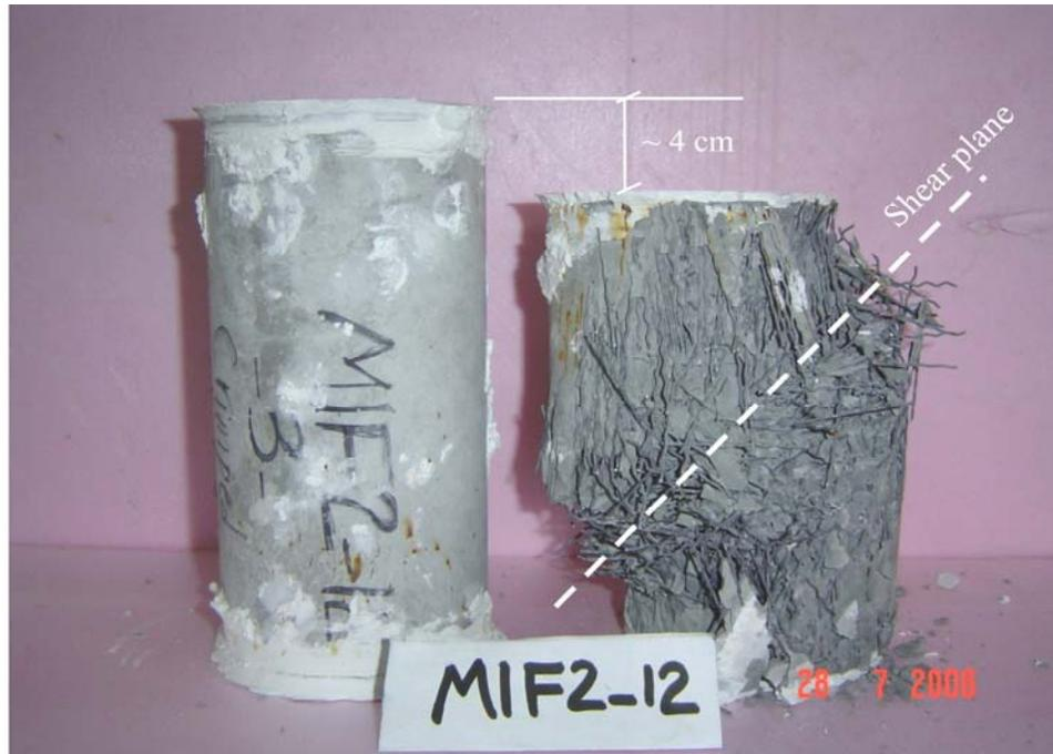
**Figure 4.3: Shear Failure and high deformation in a tested SIFCON specimen**
