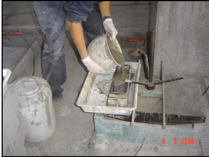
**Figure 2.4: Slurry infiltration aided with external vibration**
