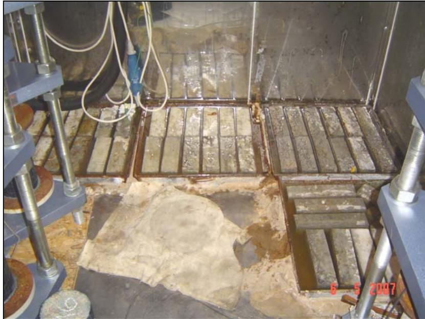
**Figure 3.13: Specimens subjected to freezing-thawing cycles in the climate chamber**
