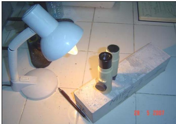
**Figure 4.12: Crack microscope used in crack mapping of SIFCON**
