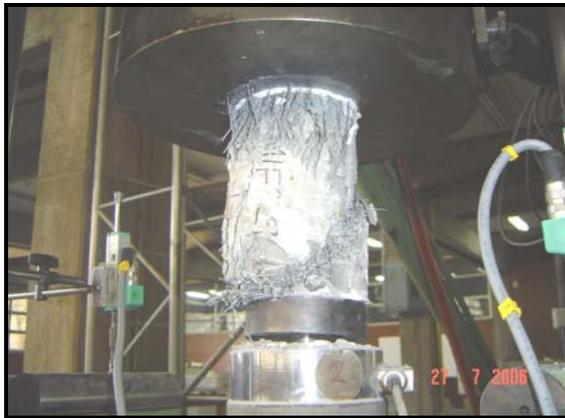
**(b) Formation of diagonal shear crack**
