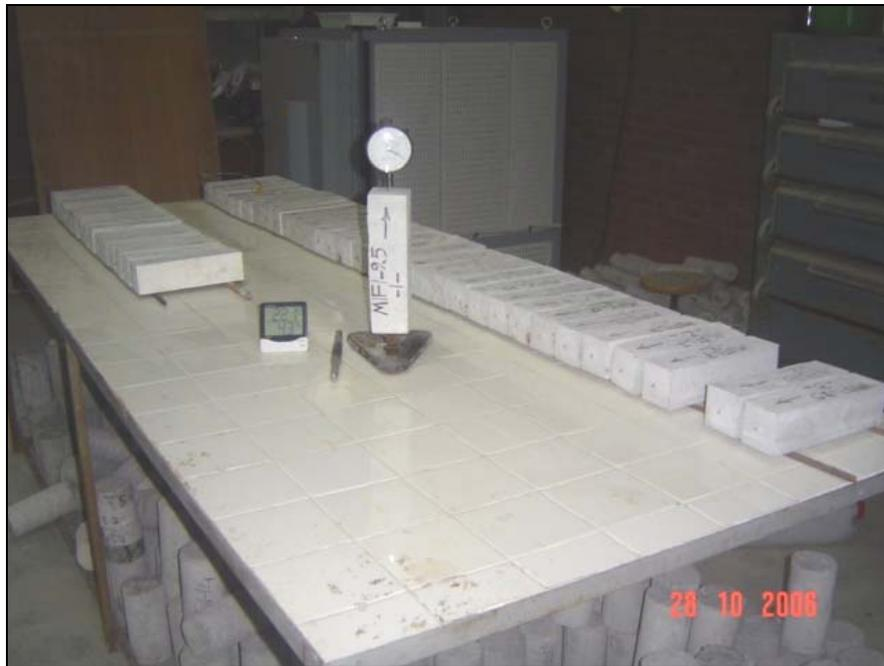
**Figure 3.7: The drying shrinkage specimens and the length measurement device**
