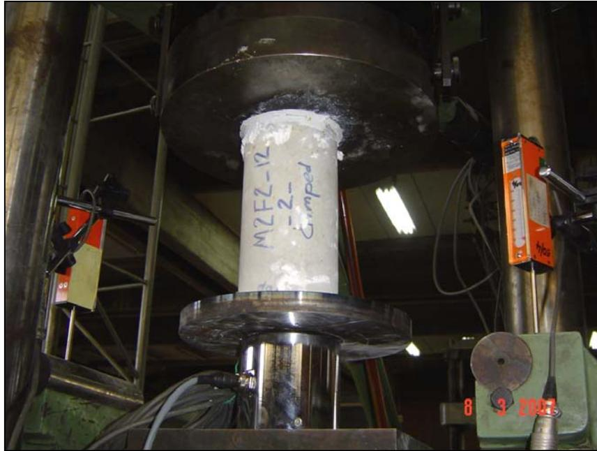
**Figure 3.3: The testing system of stress-strain behavior**
