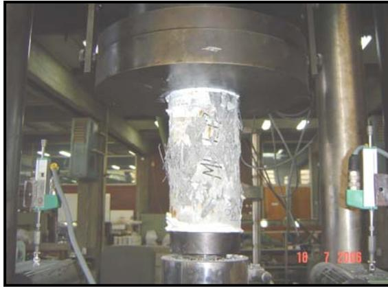
**(a) Surface scaling starts after reaching the peak load**
