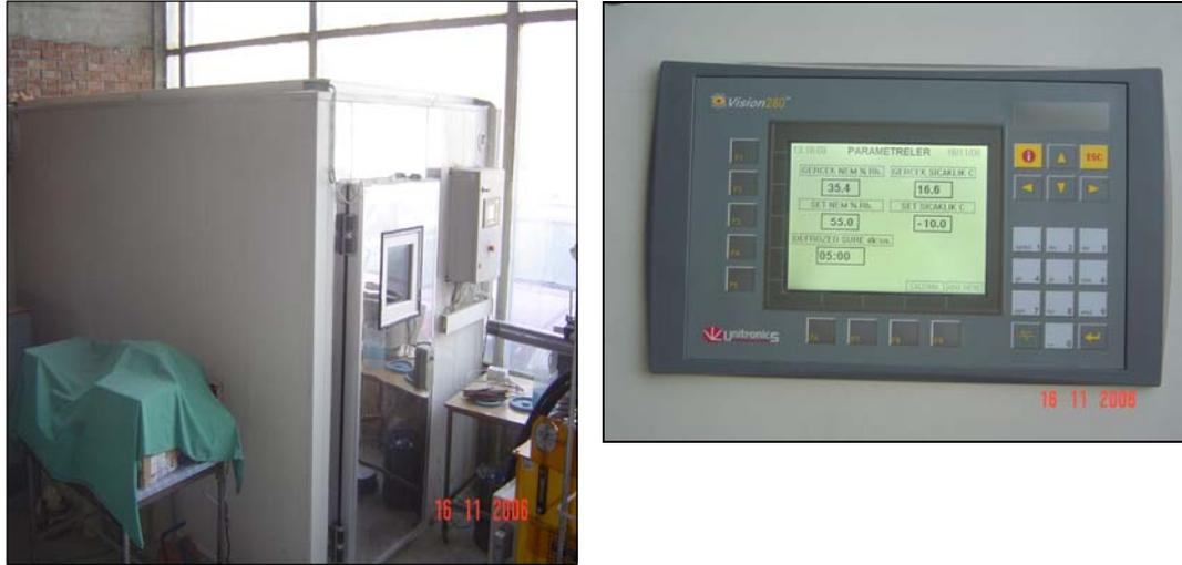
**Figure 3.15: The climate room used for freeze-thaw test and its control panel**
