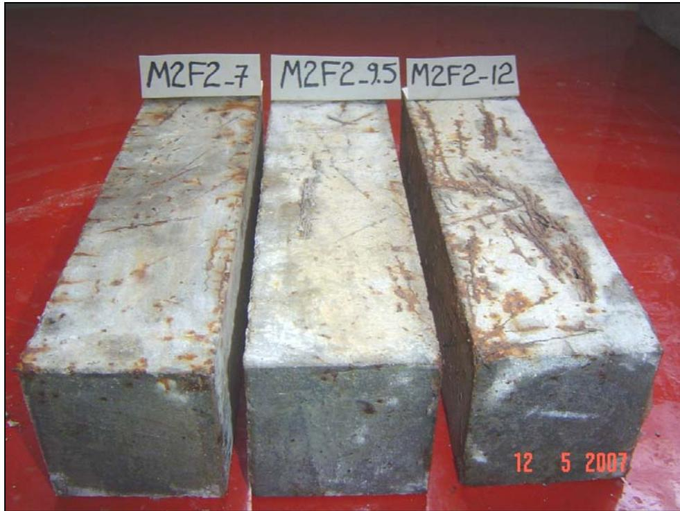
**Figure 4.42: Representative samples of mortar SIFCON after 300 cycles of freezing and thawing**
