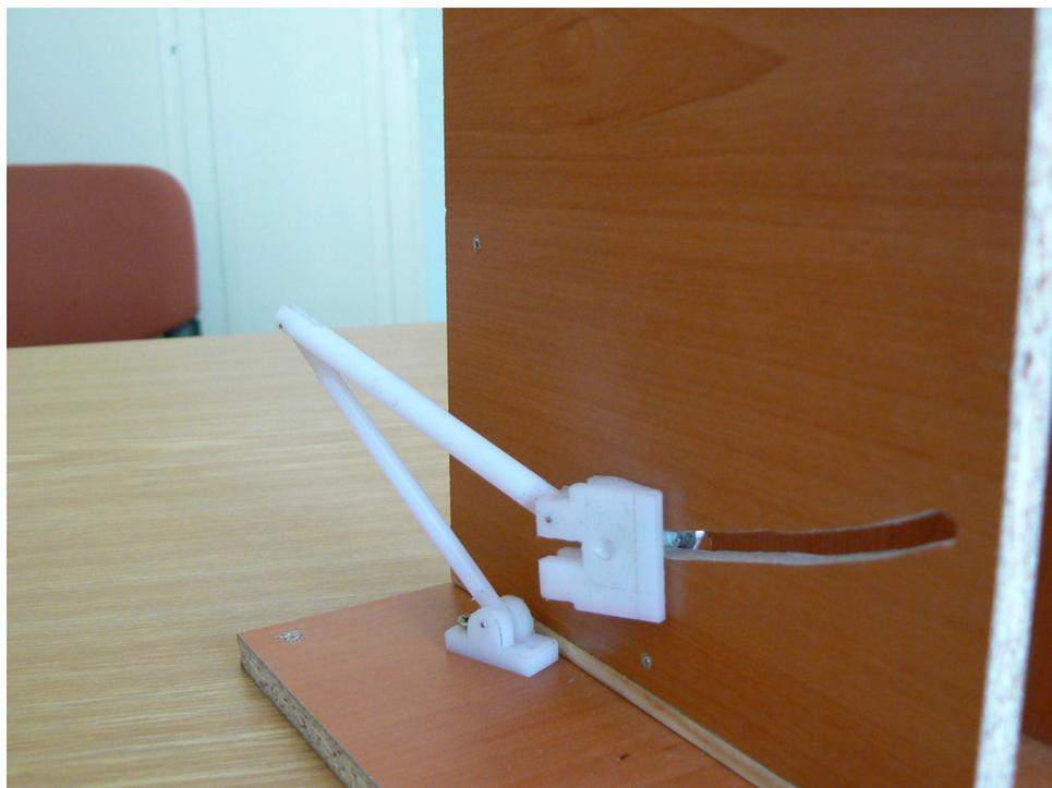
Figure 6.3 Position of center of mass prototype in a jumping leg model until take-off (Atılım University, Biomimetic Design Laboratory)
