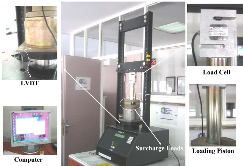
**Figure 3.15 System for CBR Testing**
