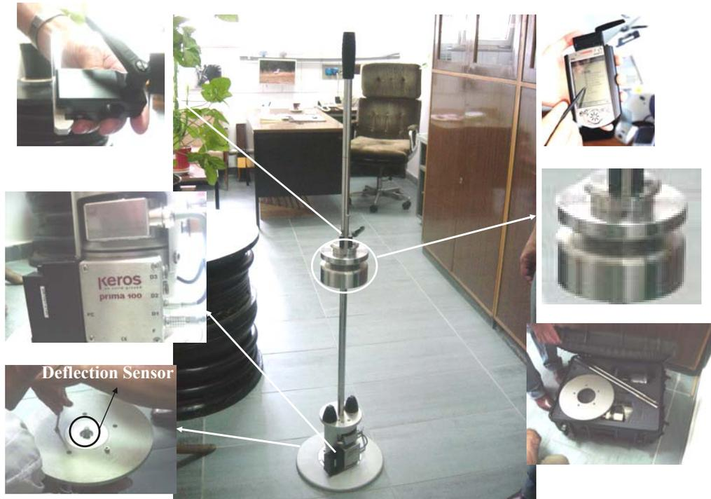
**Figure 3.18 LFWD Test Setup**
