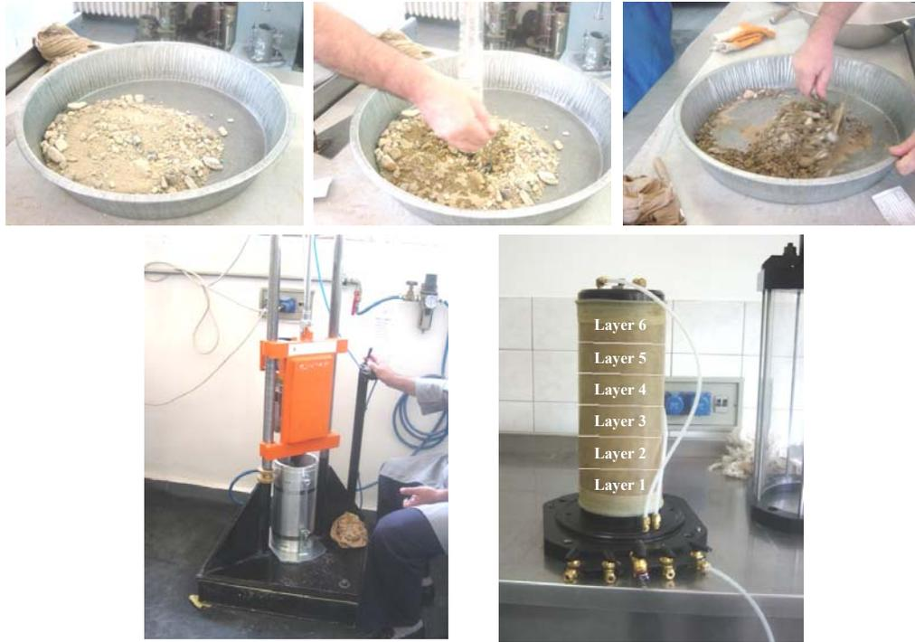
**Figure 3.11 Specimen Preparation Procedure for Granular Materials**
