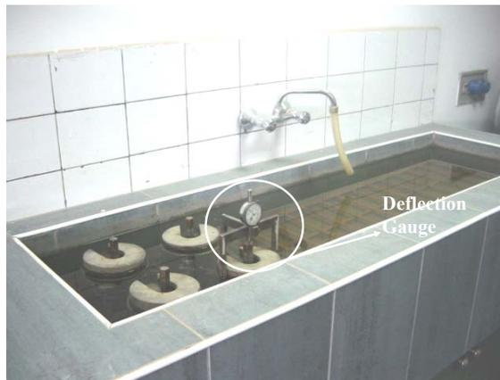
**Figure 3.16 Saturation Pool for Soaked CBR Specimen Preparation**
