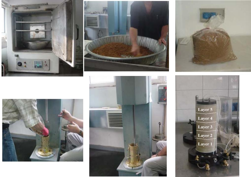
**Figure 3.12 Specimen Preparation Procedure for Fine-Grained Soil Types**
