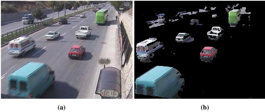
**Figure 2.9 Simulation result of the shadow removal algorithm (a) Input image (b) Shadow removed mask**
