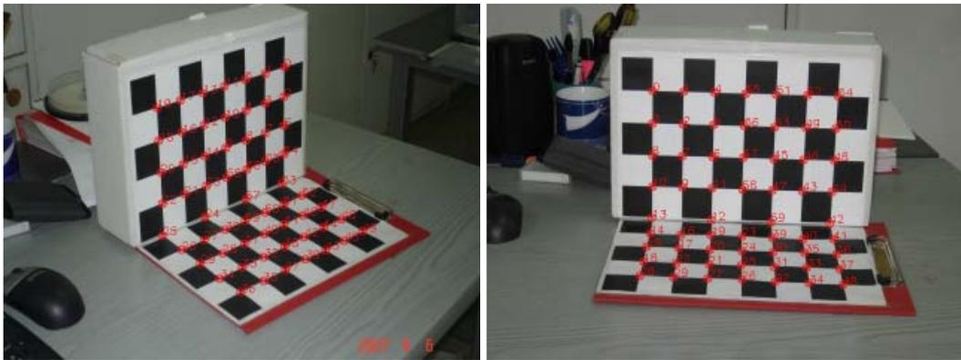
**Figure 5.6 Features that are detected by using Harris corner method**
