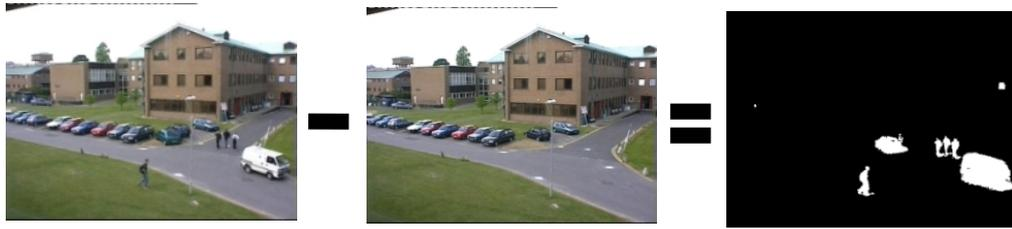
**Figure 2.1 Moving object detection process : Foreground mask is obtained by determining the difference between the input image and the available background model**
