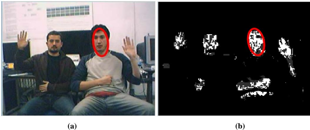
**Figure 2.10 Probability image generation (a) Input image (b) backprojection image where the face is used as the color model**
