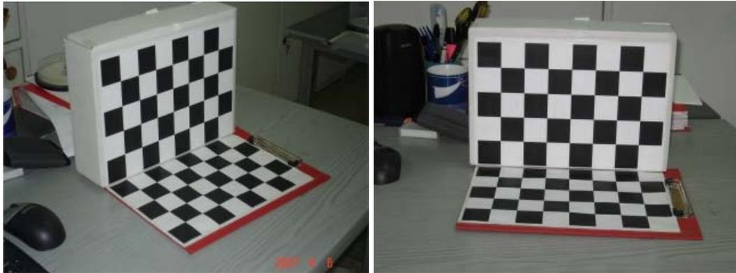
**Figure 5.5 Checker-board patterns which are used to calibrate cameras**
