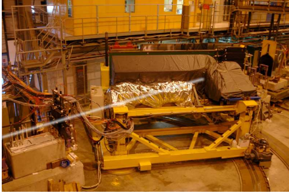
Figure 4.2: EB,HB and HE on the rotatable table. The white line represents the beam.
