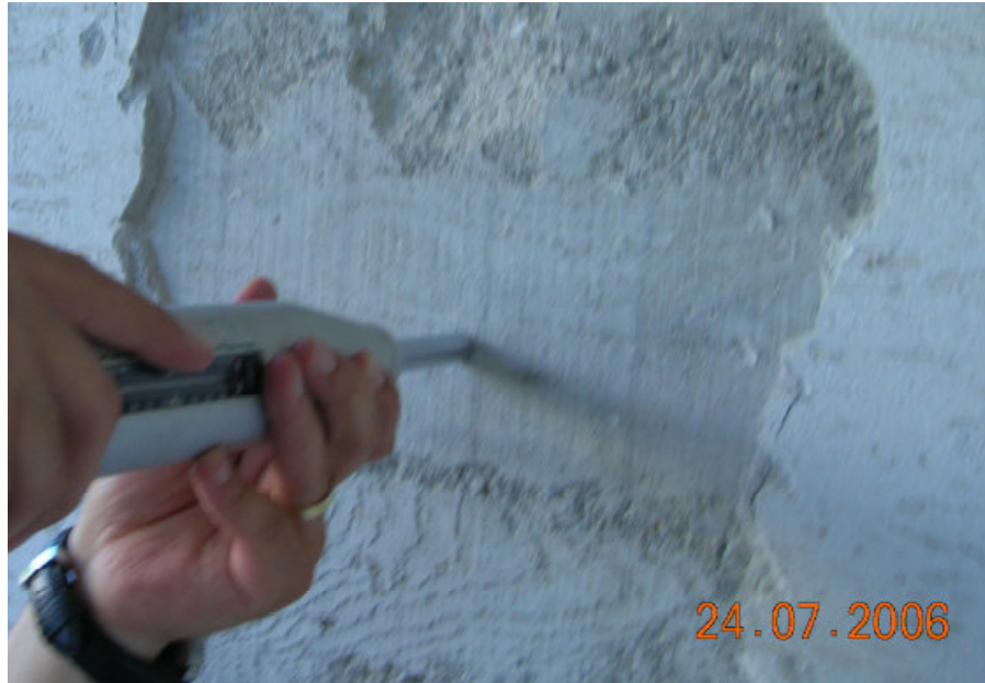
Figure 3.2 Rebound numbers taken by Schmidt Hammer
