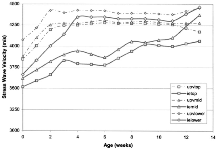
Figure 2.10 The increase in wave velocities with time in a concrete specimen with 0.45 W/C ratio. A comparison is also shown between the impact-echo and the ultrasonic pulse method. [11]
