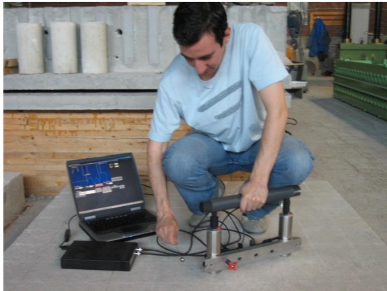
Figure 3.7 An instant during wave speed measurement
