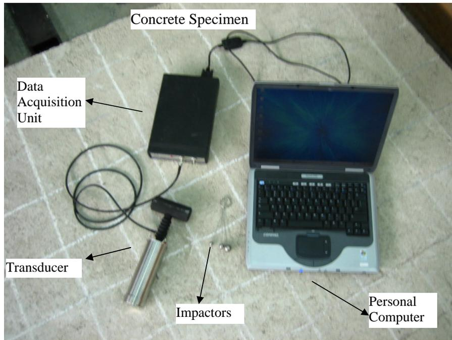
Figure 2.7 The main components of the impact-echo method
