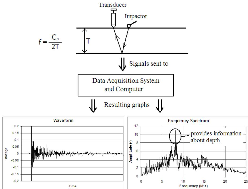
Figure 2.3 Schematic description of the impact-echo test procedure
