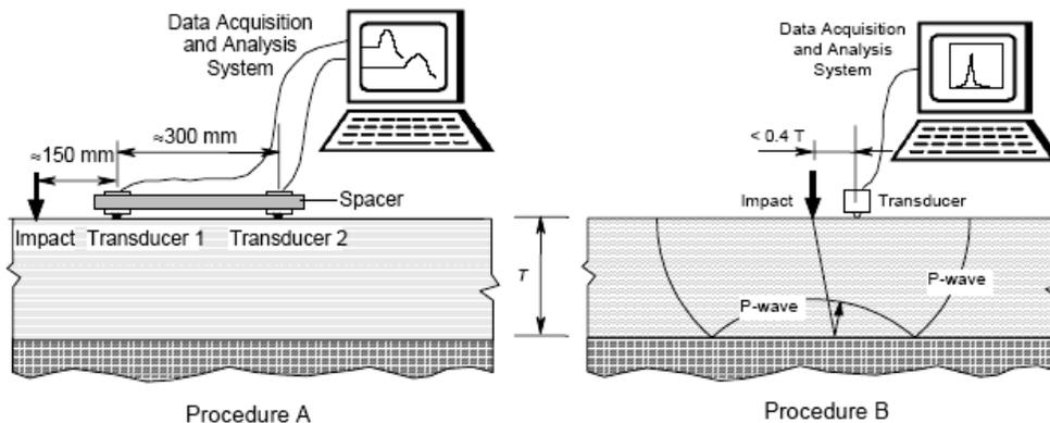
Figure 2.12 Procedure to be followed for impact-echo testing [16]
