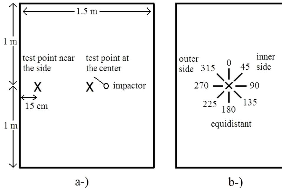
Figure 4.8 Schematic view of the test locations
