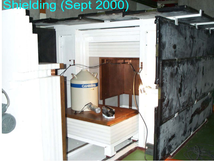
Figure 4.2: The multi-purpose inner target volume where both ULB-HPGe and CsI(Tl) scintillating crystal detectors were placed with dimension of 100 \times 80 \times 75 \text{ cm}^3 showing the HPGe detector and shielding materials.
