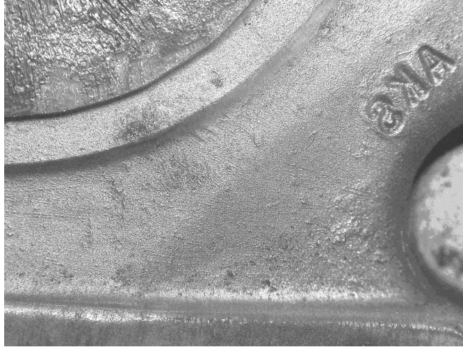
Figure 1.4 The surface manufactured by using EDM [8]
