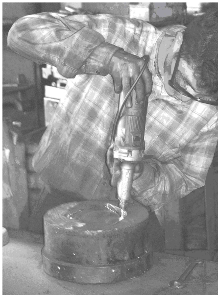
Figure 1.5 Manual polishing on die surface [8]
