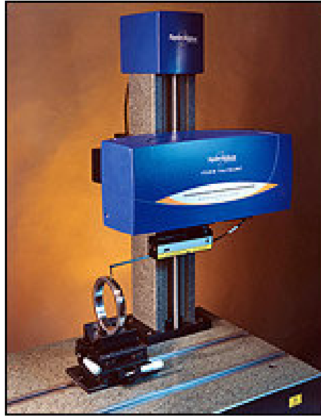
Figure 5.4 Taylor Hobson's Talysurf PGI stylus type surface roughness measuring machine
