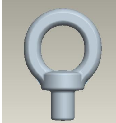
Figure 4.1 CAD model of M24 forged eye bolt
