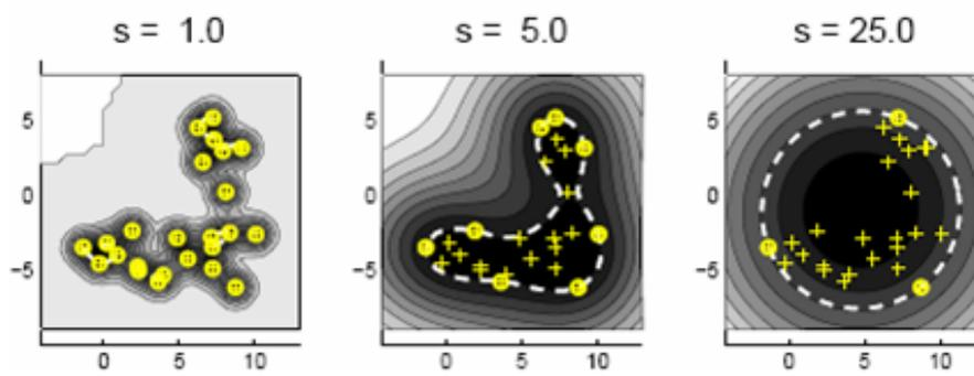
Figure 2.4: Impact of different width parameters values on a data description trained on a banana-shaped set. Support vectors are marked by circles.
