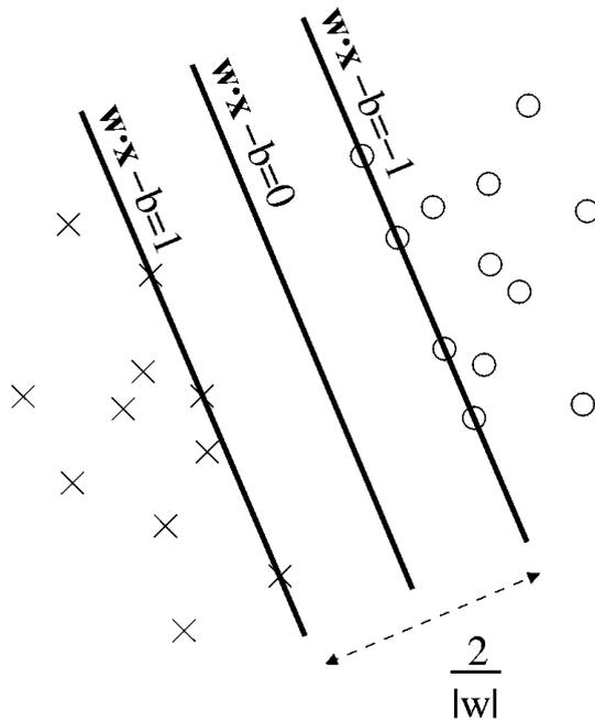
Figure 2.2: Maximum-margin hyperplanes for a SVM trained with samples from two classes. Samples along the hyperplanes are called the support vectors.
