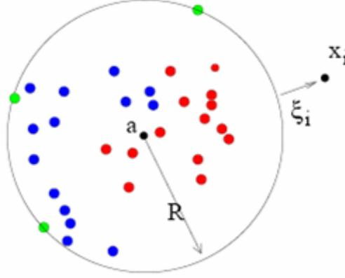
Figure 2.3: Spherical data description: hypersphere containing the target data is described by the center  $a$  and radius  $R$ . Three objects are on the boundary which are the support vectors. One object  $x_i$  is outside and has  $\xi_i > 0$ .
