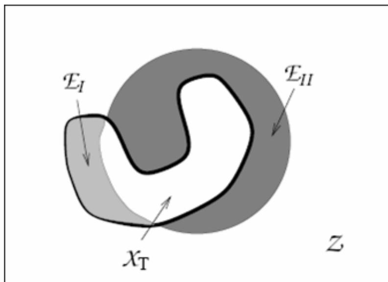
Figure 2.1: Regions in classification: a spherical data description boundary is trained around a banana shaped target distribution.
