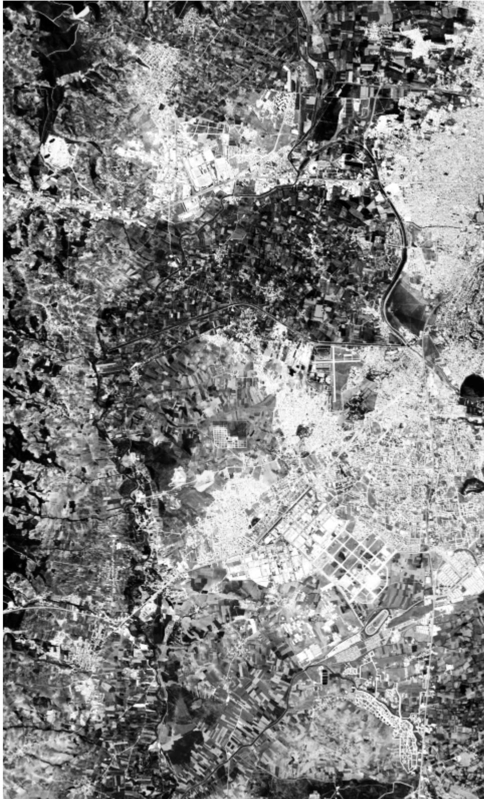
Figure 4.1: Prototype experiment image: single band SPOT panchromatic image of size  $(2400 \times 4000)$  with a spatial resolution of  $10m$ .
