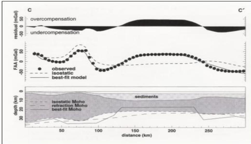
Figure 5.5: Gravity and state of flexure in the Eastern Black Sea (Detail of CC' Section in **Figures 5.1 & 5.2**) [20]
