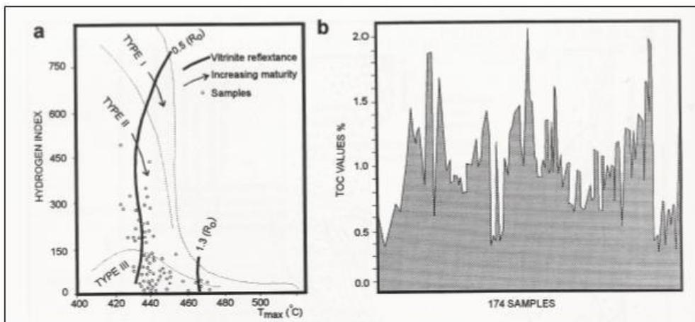
Figure 5.12: a) Rock-Eval Pyrolysis and b) Total Organic Carbon (TOC) Analyses of the Shales of the Çağlayan Formation from the Sinop Region [21]
