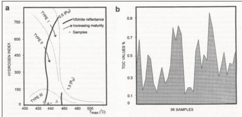
Figure 5.13: a) Rock-Eval Pyrolysis and b) Total Organic Carbon (TOC) Analyses of the Shales of the Kusuri Formation from the Sinop Region [21]
