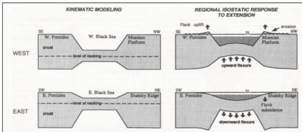
Figure 5.6: Diagram illustrating a scenario for the large-scale deformation of the Black Sea Basin and the surrounding regions [20]
