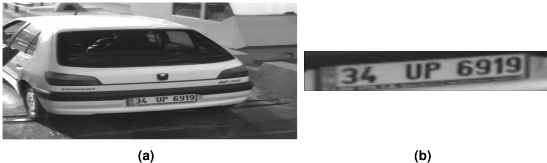
Figure 15 Extracted license plate image (a) the original image, (b) extracted plate region (zoomed)
