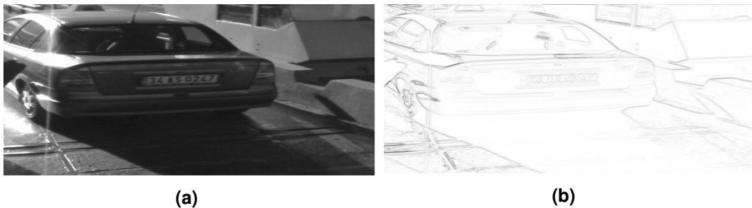
Figure 5 Sample image and its edge map (a) acquired image, (b) Sobel edges without preprocessing
