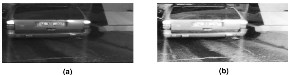
Figure 7 Histogram equalization (a) original image, (b) histogram equalized image,
