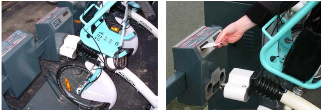
Figure 3.4 Adshel (Rennes) - release of the PUB through the use of a magnetic stripe card ( http://velo-lacarte.free.fr/smartbike.html )
