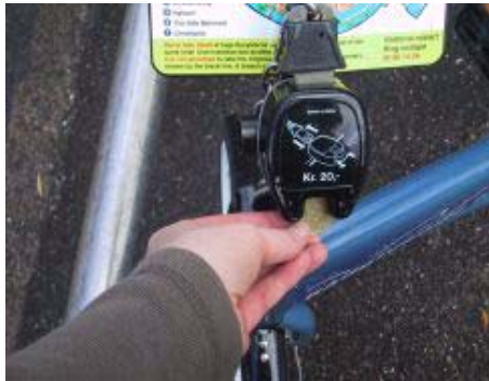
Figure 4.1 Coin deposit system ( http://ruk.ca/article/2870 )
